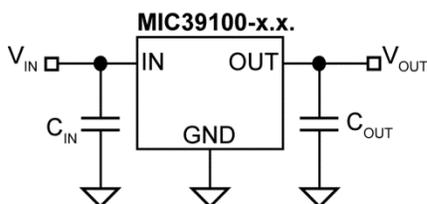
Figure 1. Capacitor Requirements
