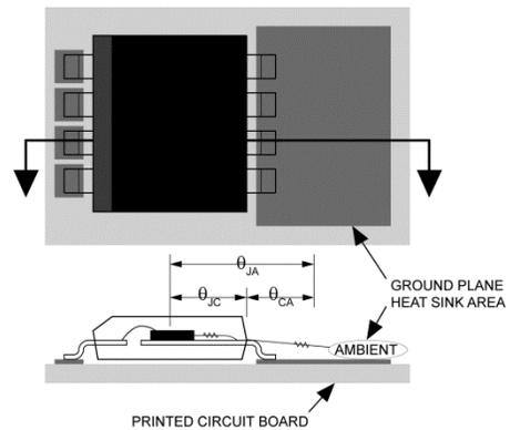
**Figure 3. Thermal Resistance**
