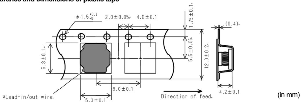
Dimension of the Cavity is measured at the bottom side.
