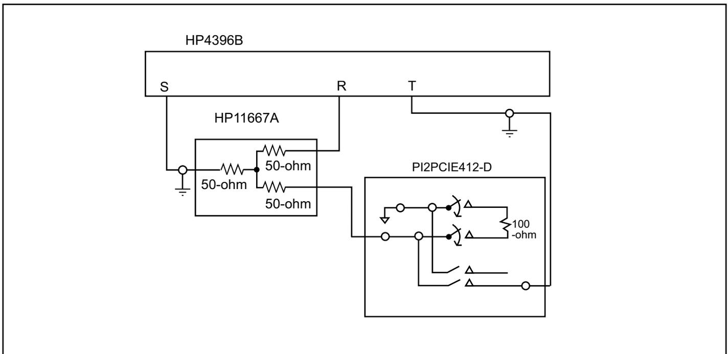
**Fig 2. Off-isolation setup**
