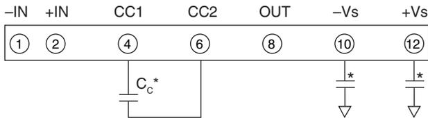
\* 0.01µF or greater ceramic power supply bypassing required. CC = 10pF minimum, 1kV NPO (COG).
