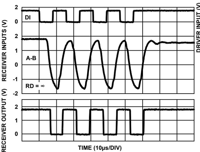
FIGURE 9. ISL32613E AND ISL32611E PERFORMANCE WITH V<sub>CC</sub> = 1.8V, 128kbps, 2000' (610m) CAT 5 CABLE
