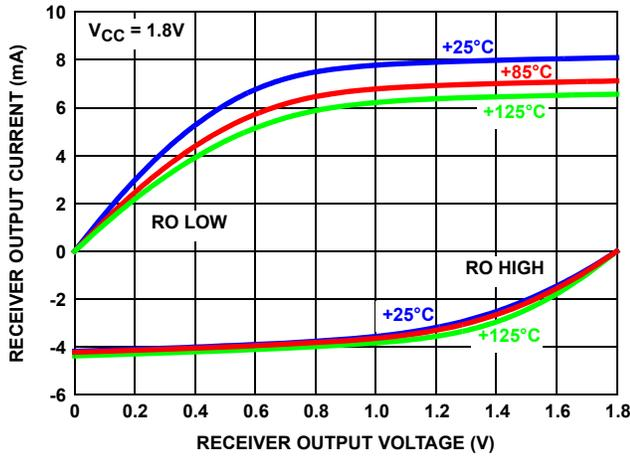
FIGURE 5. RECEIVER OUTPUT CURRENT vs RECEIVER OUTPUT VOLTAGE (V<sub>CC</sub> = 1.8V)
