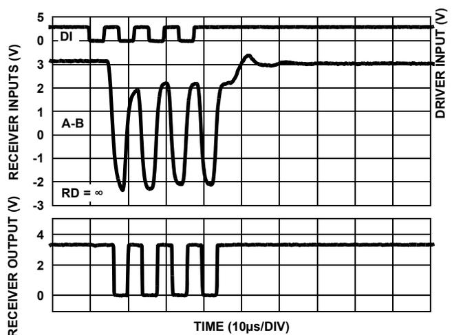
FIGURE 10. ISL32613E AND ISL32611E PERFORMANCE WITH V<sub>CC</sub> = 3.3V, 256kbps, 3000' (915m) CAT 5 CABLE
