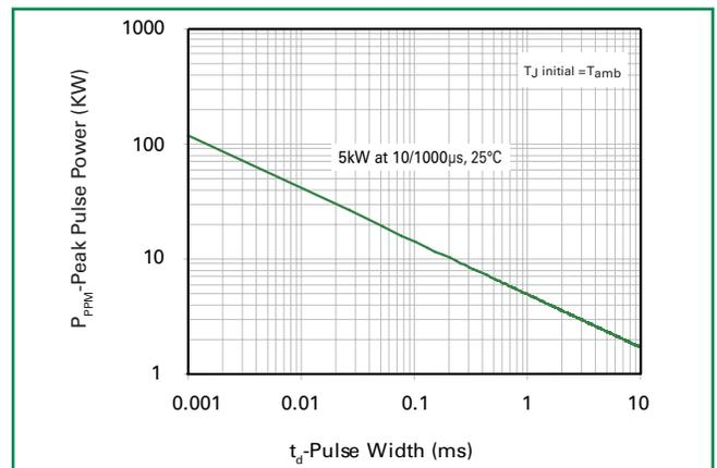
**Figure 3 - Peak Pulse Power Derating Curve**
