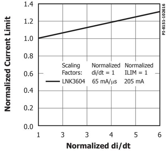
Figure 23. Reduced Current Limit vs. di/dt.
