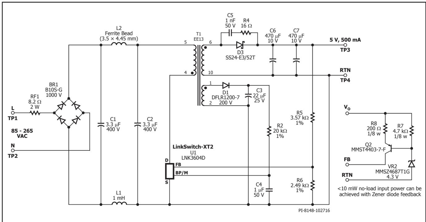
Figure 8. 2.5 W Universal Input Design using LNK3604.
