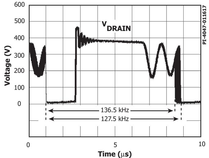
Figure 5. Frequency Jitter.
