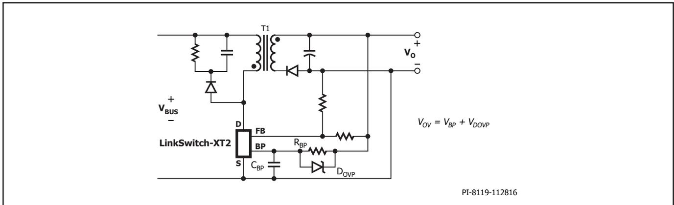
Figure 6. Non-Isolated Flyback Converter with Output Overvoltage Protection.
