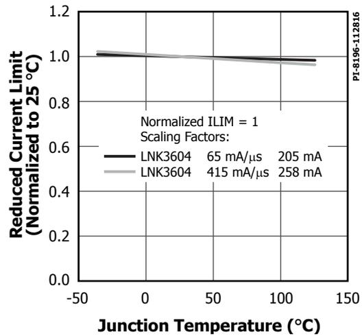
Figure 21. Reduced Current Limit vs. Junction Temperature.
