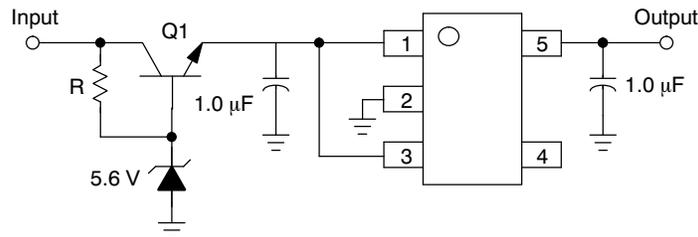
**Figure 22. Input Voltages Greater than 6.0 V**
