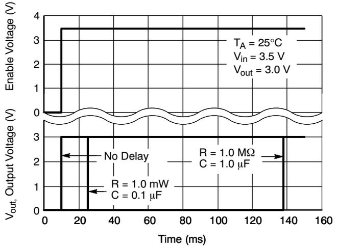
**Figure 21. Delayed Turn-on**
