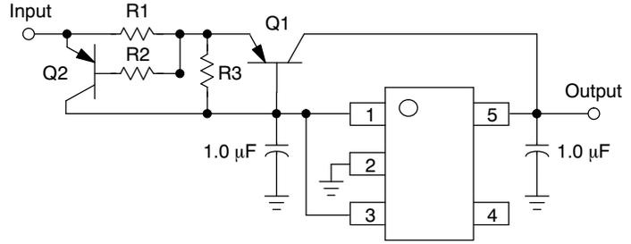
**Figure 19. Current Boost Regulator with Short Circuit Limit**
