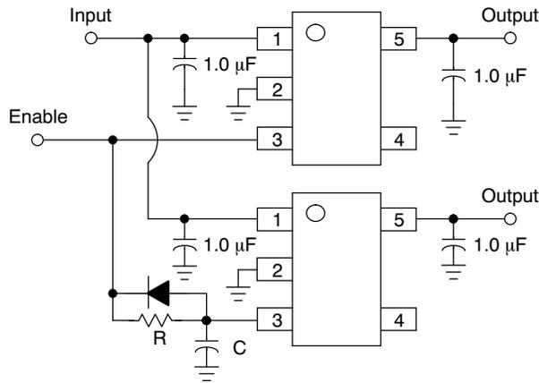
**Figure 20. Delayed Turn-on**
