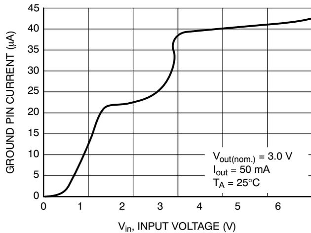
Figure 6. Ground Pin Current vs. Input Voltage
