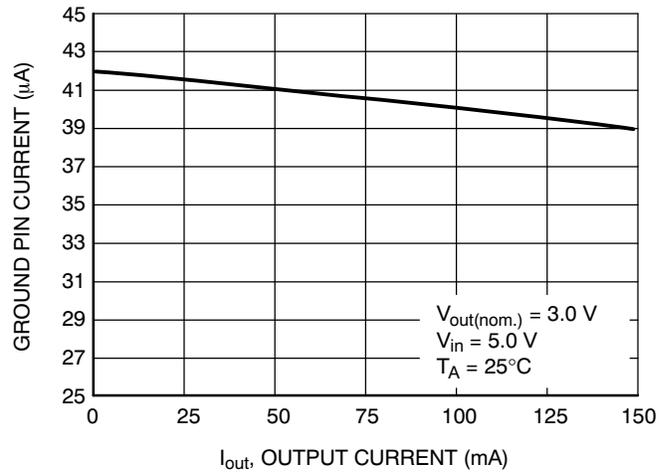
Figure 5. Ground Pin Current vs. Output Current
