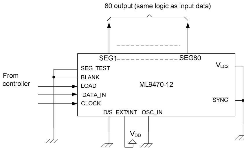
\*The output logic can be reversed with respect to the input data by setting OSC\_IN to "H" level.
