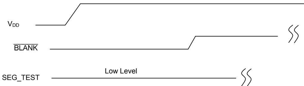
\* After  $V_{DD}$  is applied,  $\overline{BLANK}$  and  $SEG\_TEST$  should be applied to 'L' level to make all SEGMENTS off until first group of display data is latched.
