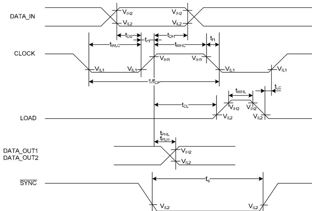
( $V_{IH} = 0.8V_{DD}$   $V_{IL} = 0.2V_{DD}$ )
