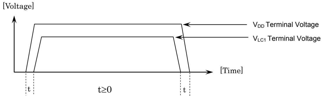
\*  $V_{LC1}$  and  $V_{LC2}$  are applied when  $V_{DD}$  is applied to external bias resistor.
