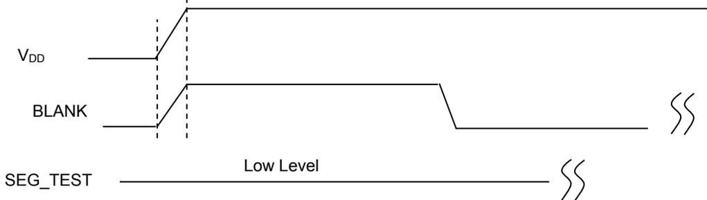
\* When  $V_{DD}$  is applied,  $\overline{BLANK}$  should be applied to 'H' level at the same time, and  $SEG\_TEST$  should be applied to 'L' level to make all SEGMENTS off until first group of display data is latched.
