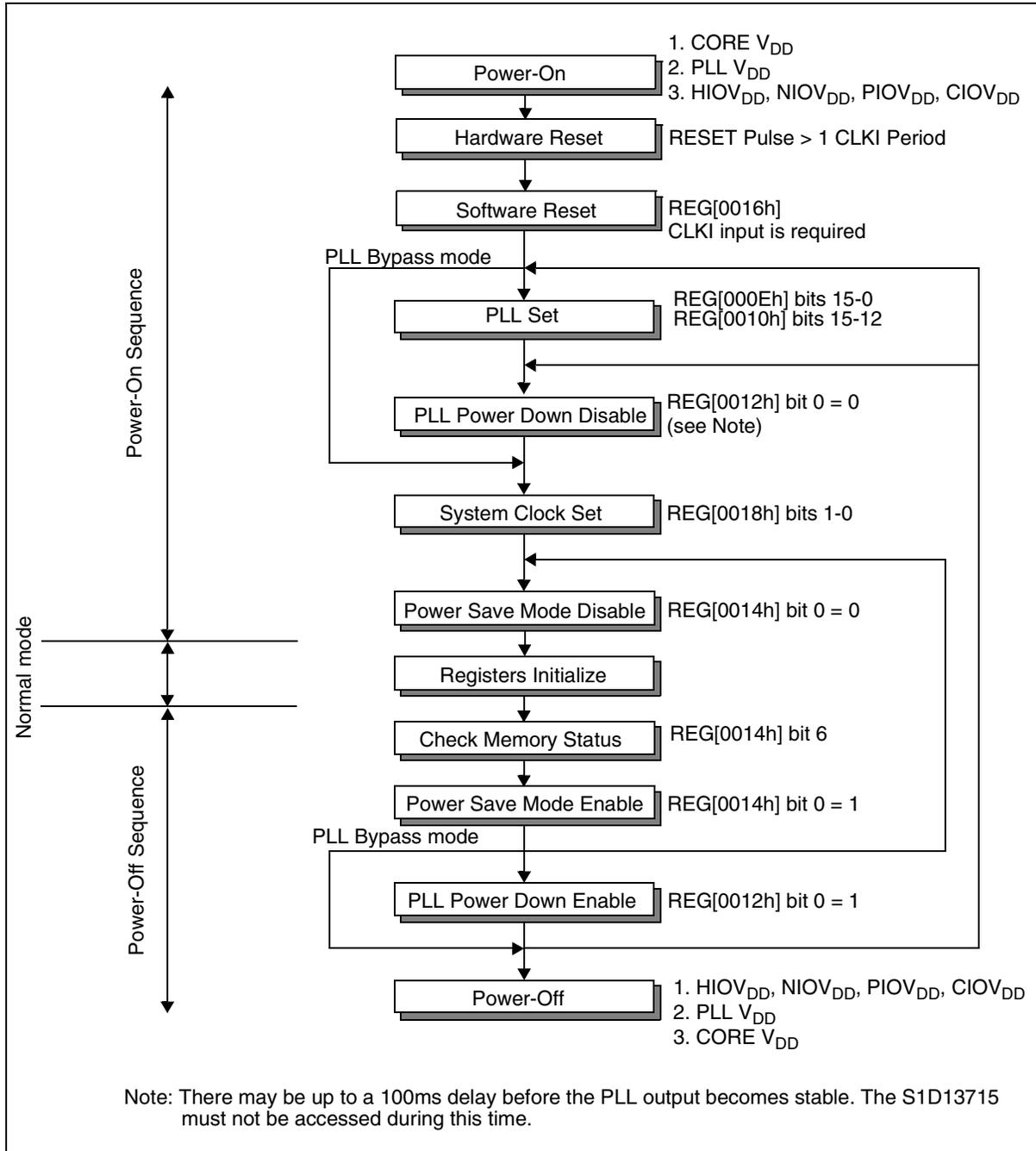
Figure 11-1: Power-On/Power-Off Sequence
