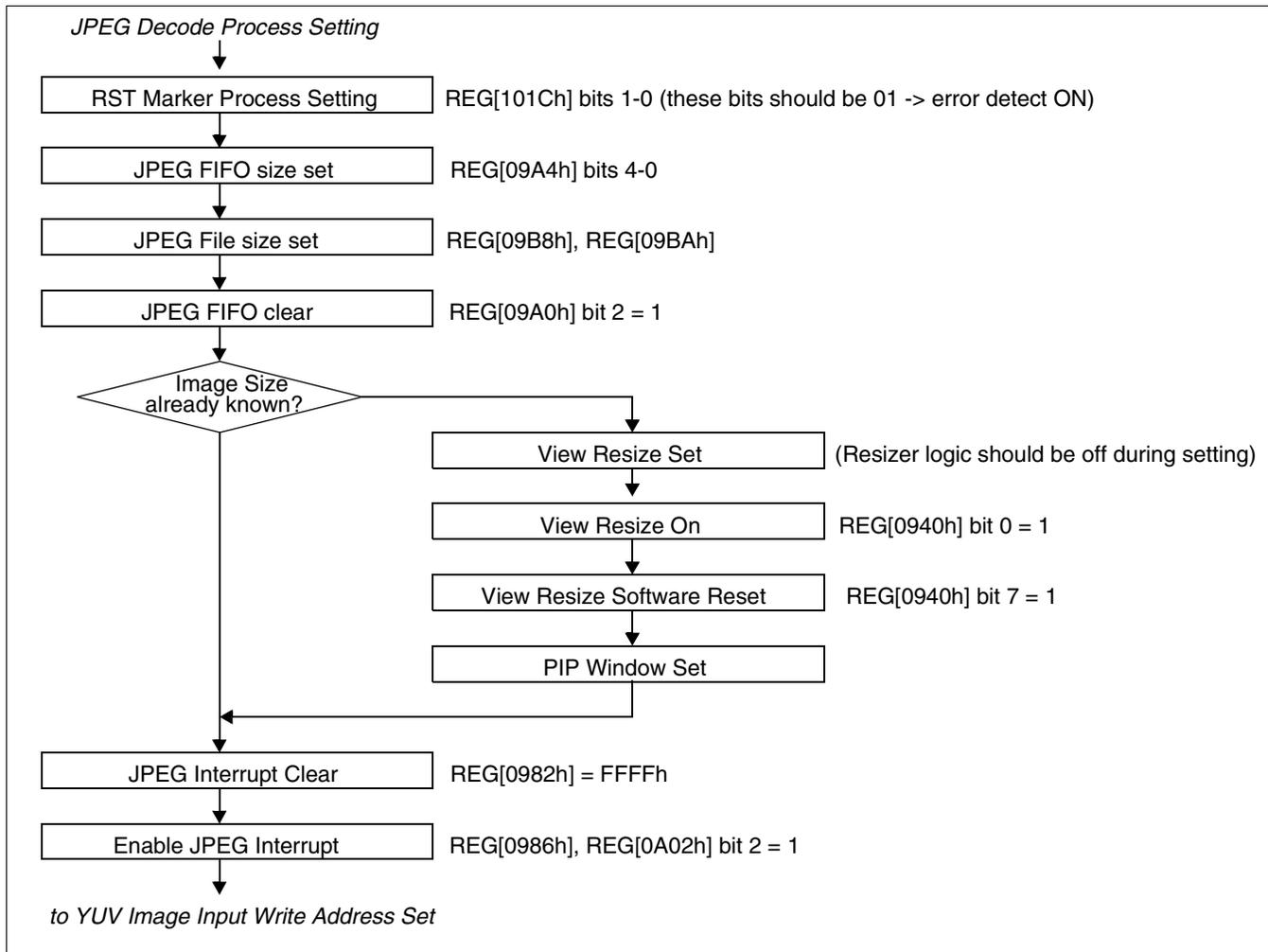
Figure 19-16: JPEG Decoding Process (3 of 6)
