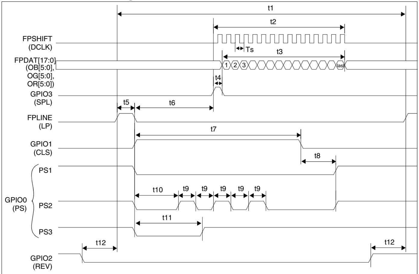
Figure 7-33: HR-TFT Panel Horizontal Timing
