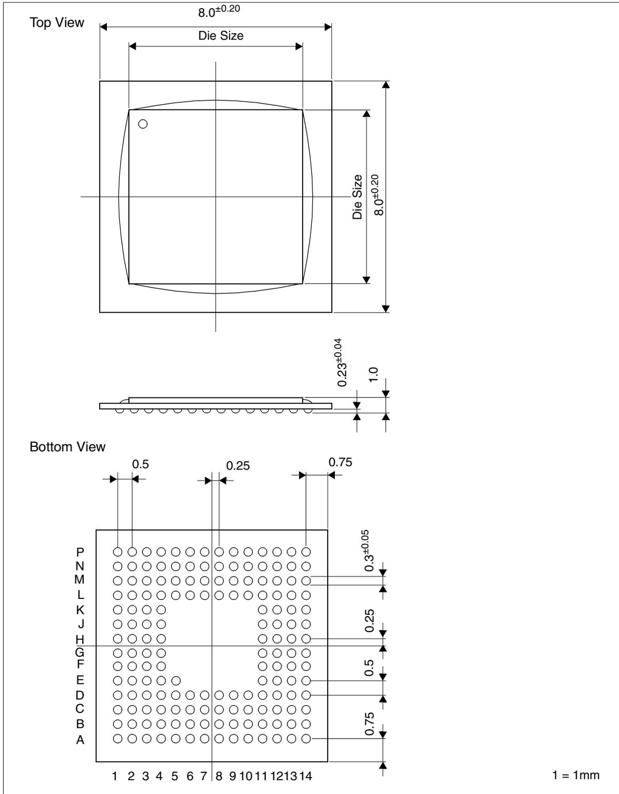
Figure 22-2: S1D13715 FCBGA 160-Pin Package
