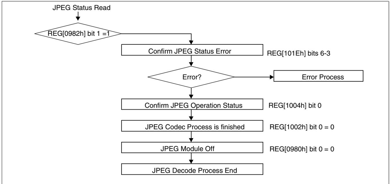
Figure 19-19: JPEG Decoding Process (6 of 6)
