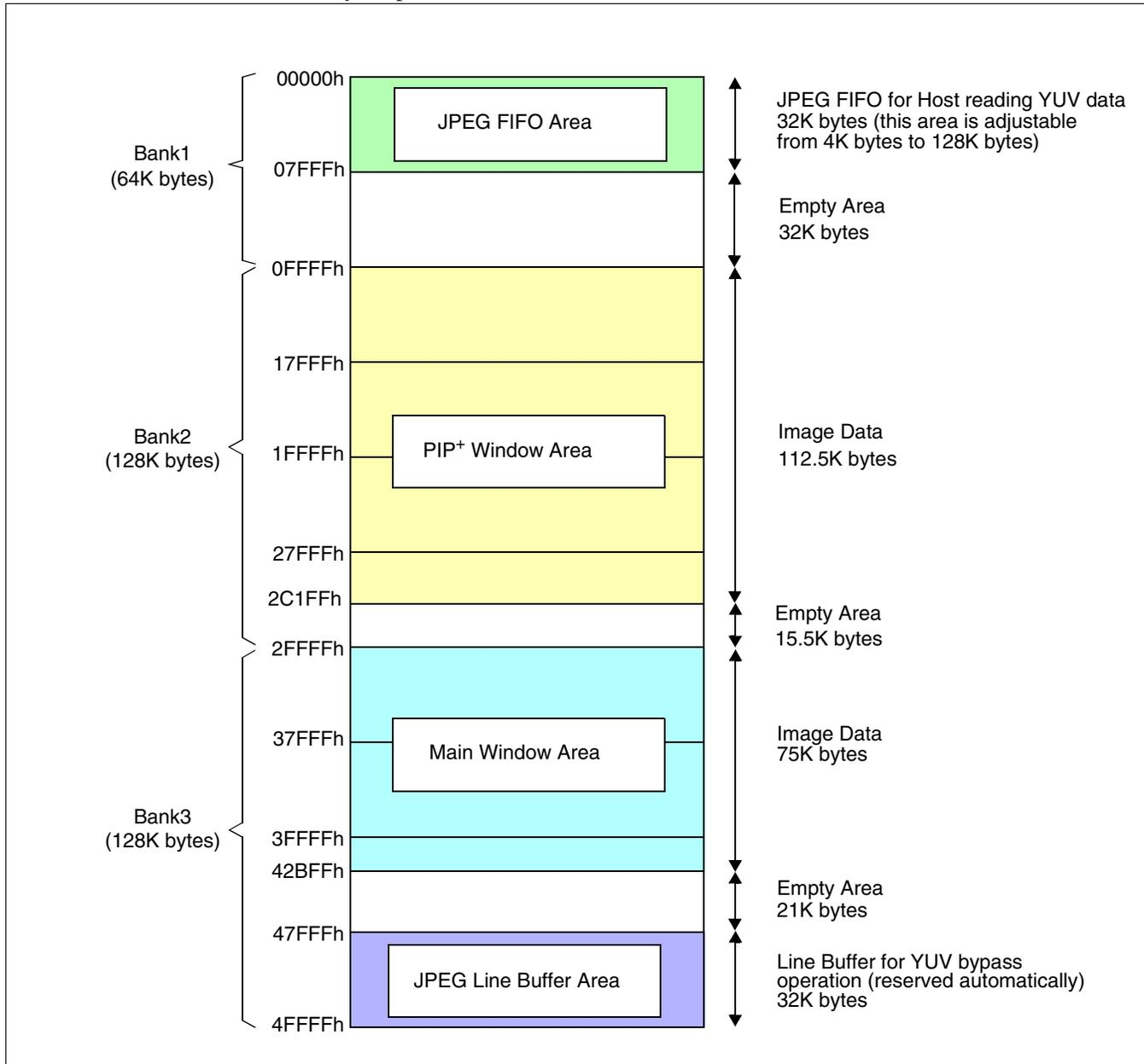
Figure 8-8: Memory Map for Main Window, PIP+ Window, Overlay, and YUV
