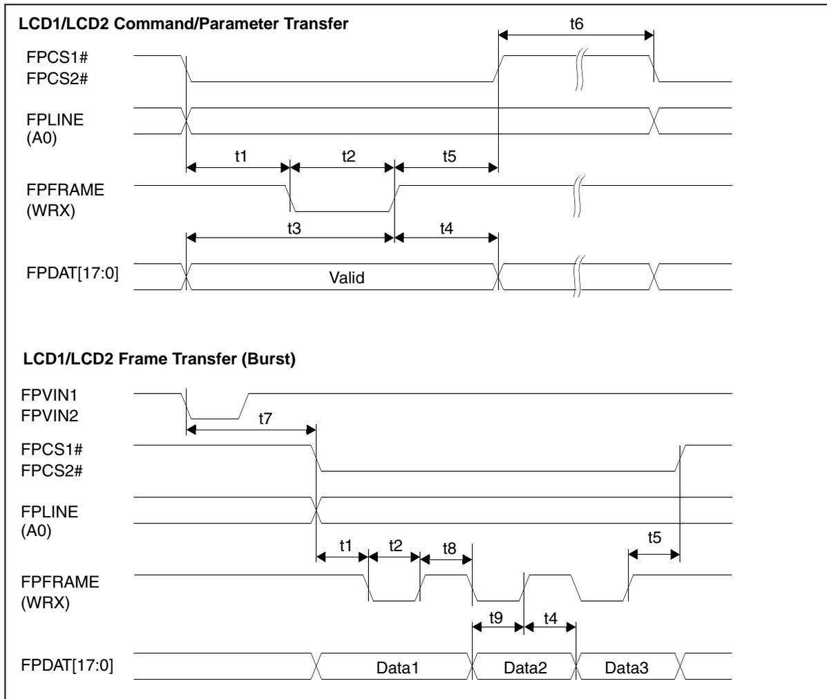
Figure 7-45: LCD1, LCD2 Parallel Interface Timing (80)
