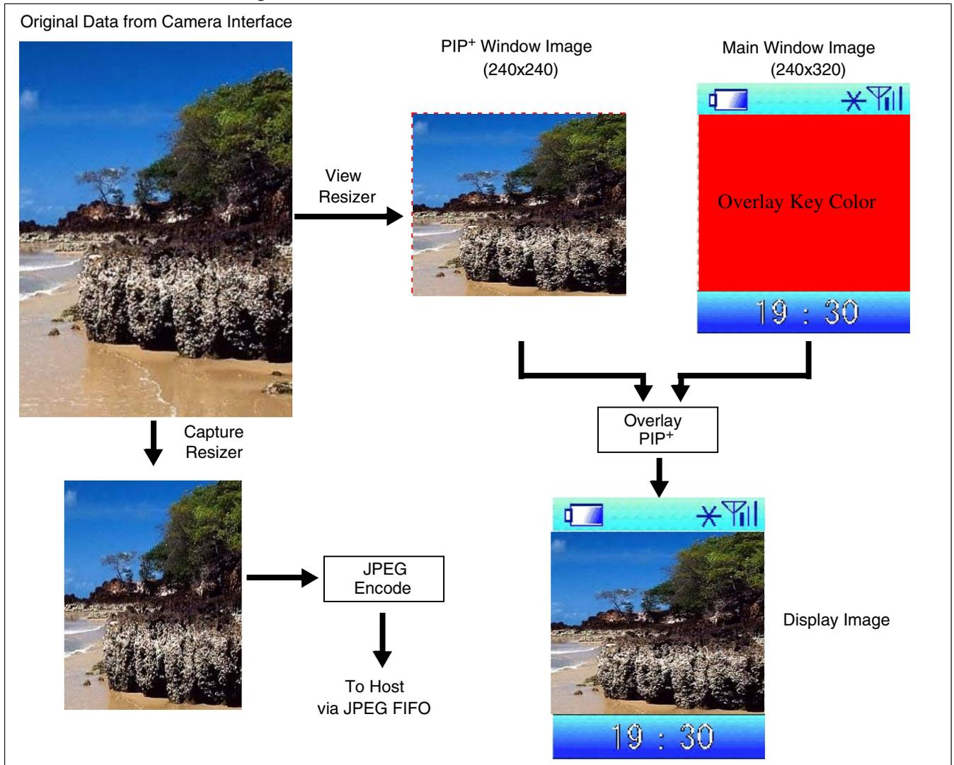
Figure 8-9: Main Window, PIP+ Window, Overlay, and JPEG
