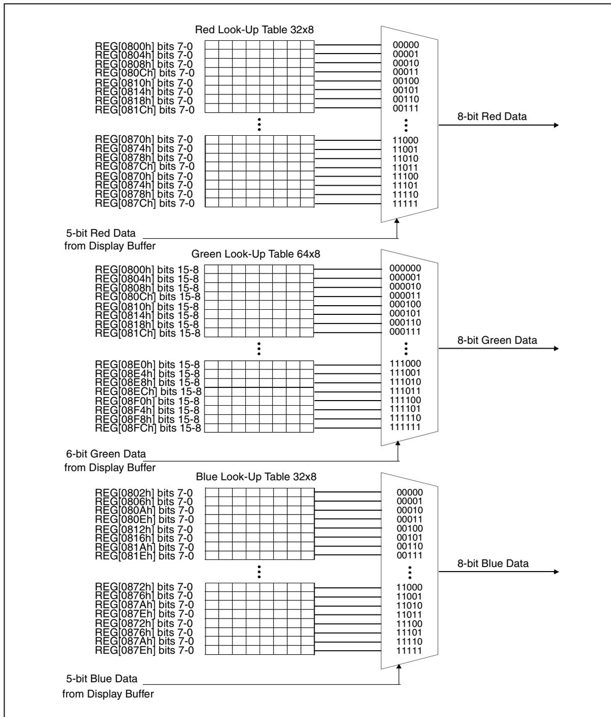
Figure 12-4: LUT2 (PIP+ Window) for 16 Bpp Architecture
