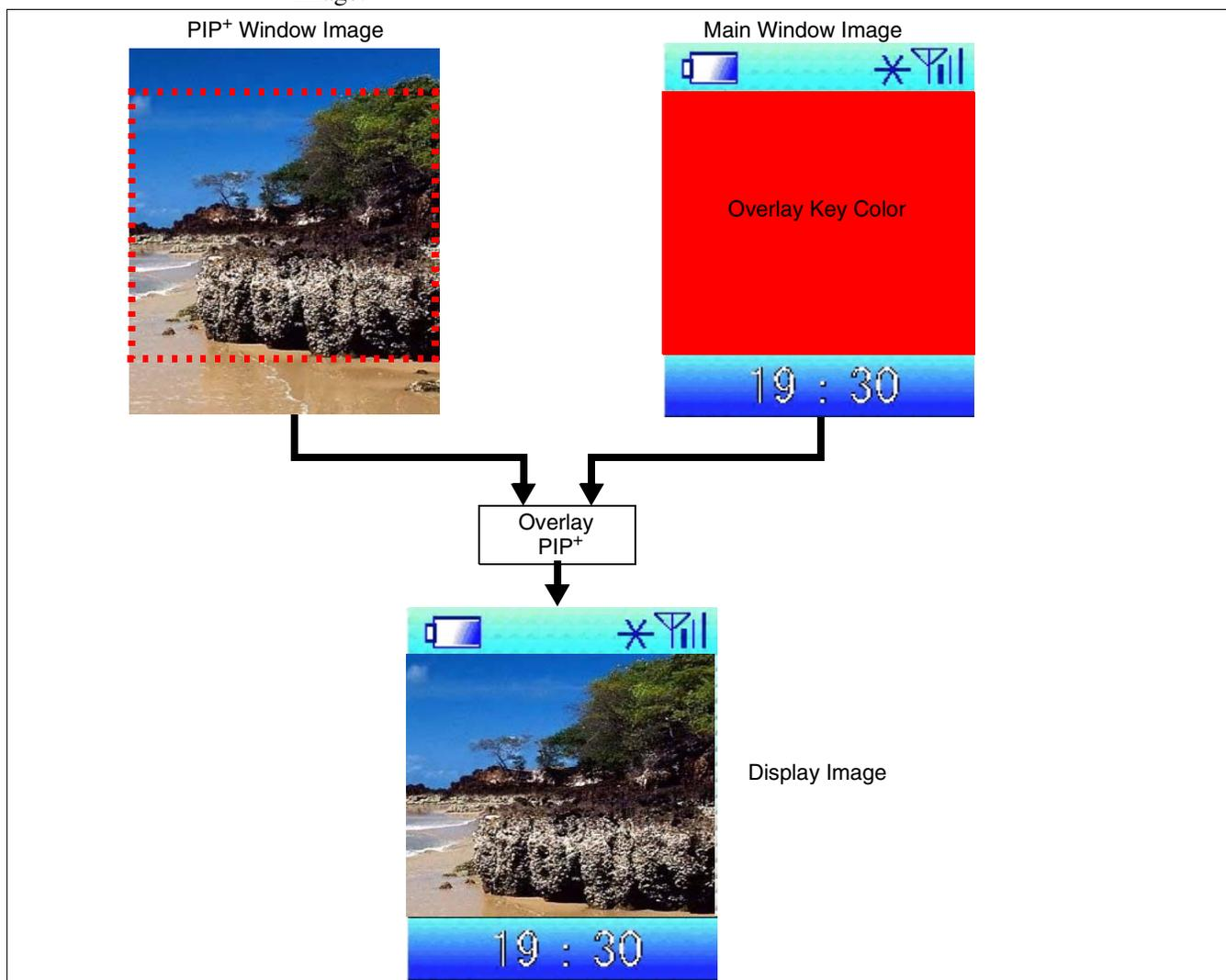
Figure 8-5: Main Window, PIP+ Window, and Overlay Display
