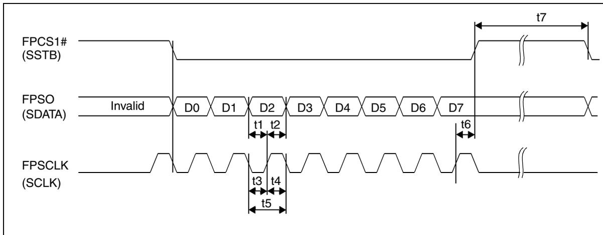
Figure 7-43: LCD1 a-Si TFT Serial Interface Timing
