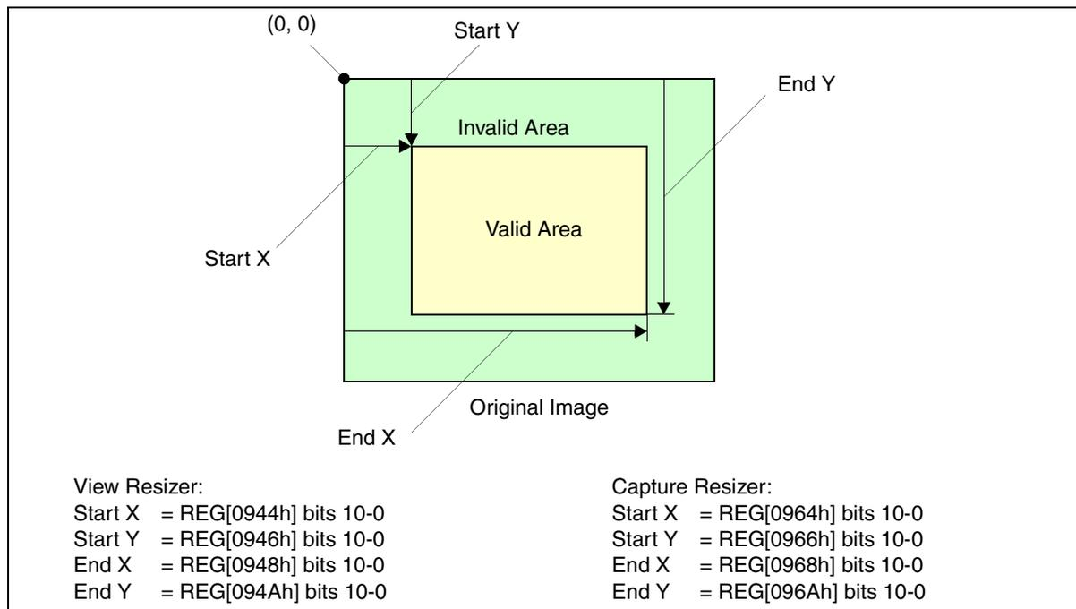
Figure 17-1: Trimming Function
