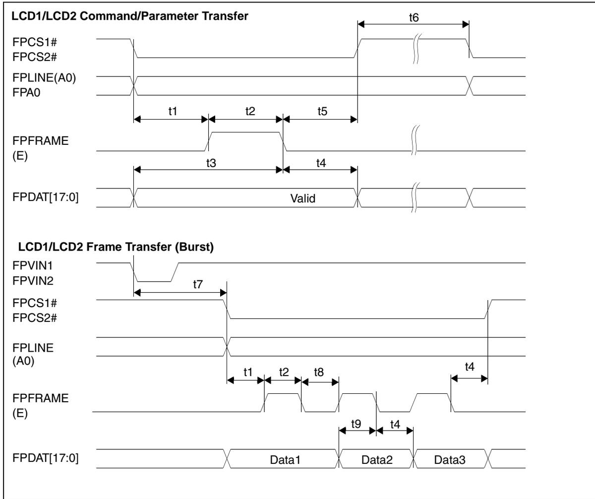
Figure 7-46: LCD1, LCD2 Parallel Interface Timing (68)
