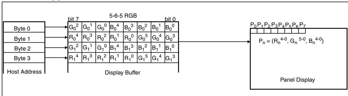
Figure 13-6: LUT Bypass for 16 Bpp mode
