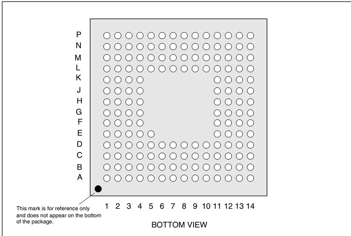
Figure 5-2: S1D13715 FCBGA-160 Pin Mapping
