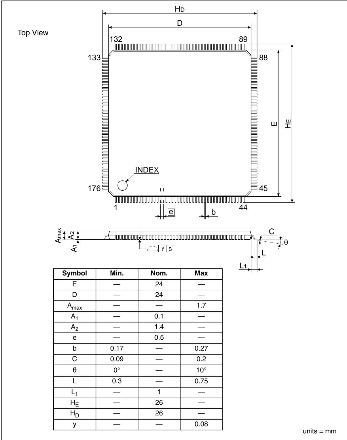
Figure 22-3: SID13715 QFP21 176-Pin Package
