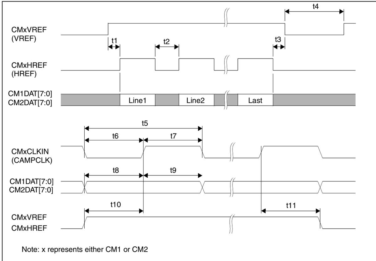
Figure 7-48: S1D13715B01 Camera Interface Timing
