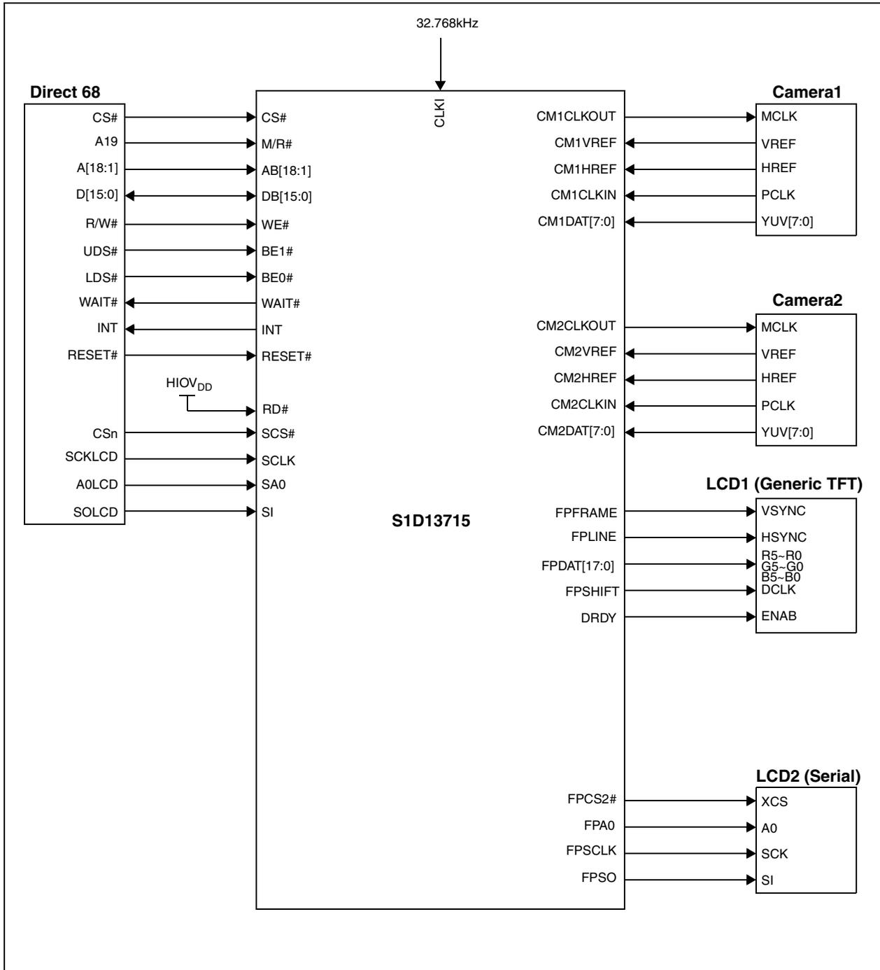
Figure 3-1: SID13715 System Diagram 1
