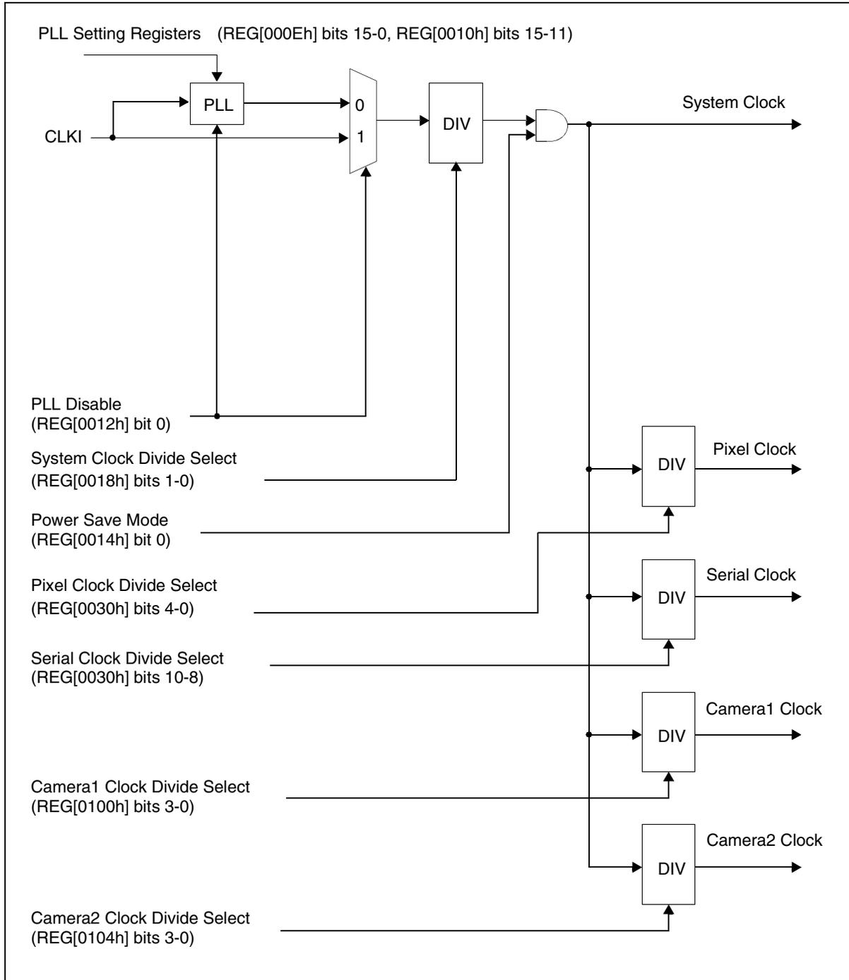
Figure 9-1: Clock Diagram
