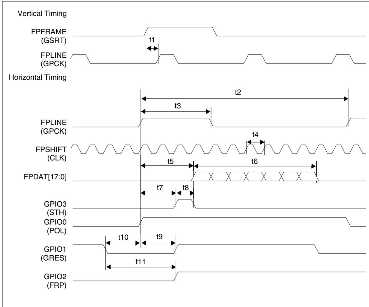
Figure 7-35: Casio TFT Horizontal Timing
