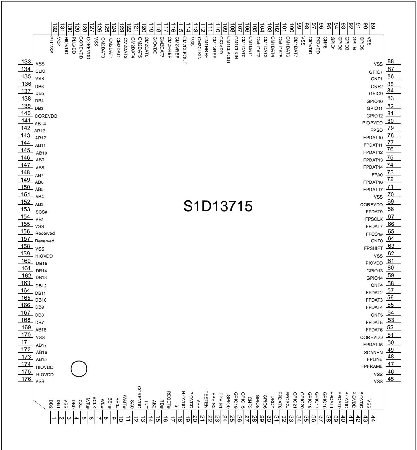
Figure 5-3: S1D13715 QFP21-176 Pin Mapping (Top View)
