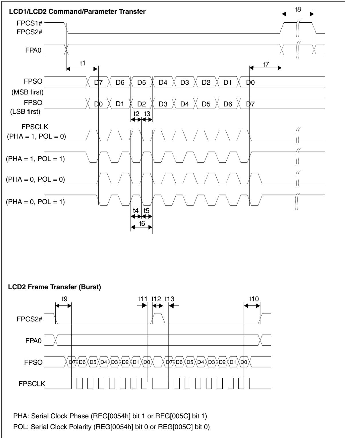
Figure 7-41: LCD1 ND-TFD, LCD2 8-Bit Serial Interface Timing
