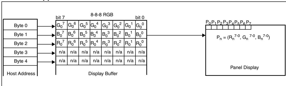
Figure 13-7: LUT Bypass for 32 bpp Mode
