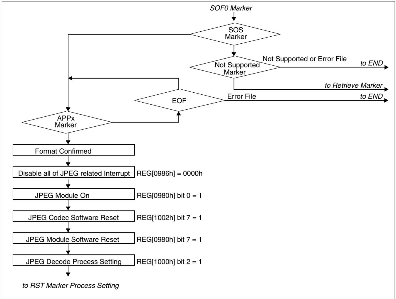
Figure 19-15: JPEG Decoding Process (2 of 6)
