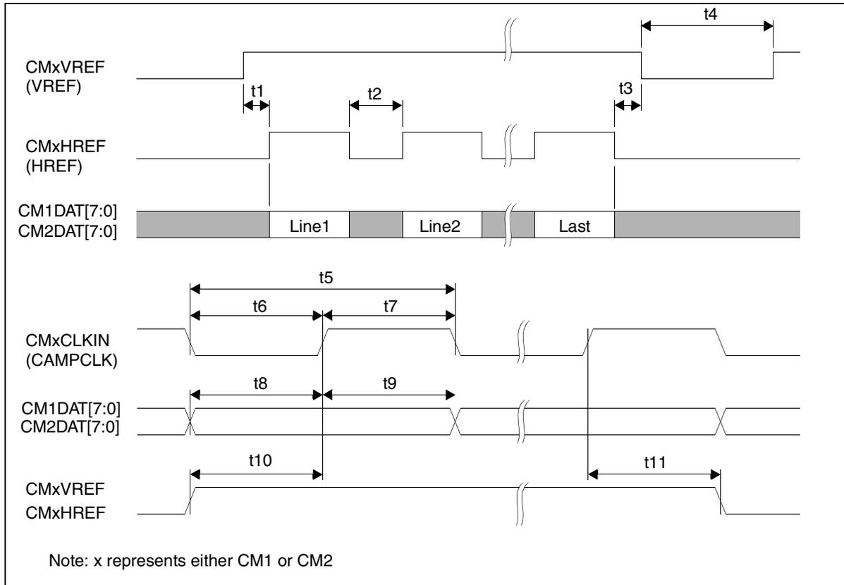
Figure 7-47: S1D13715B00 Camera Interface Timing
