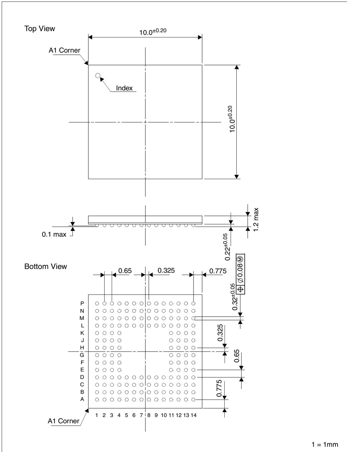
Figure 22-1: SID13715 PFBGA 160-pin Package
