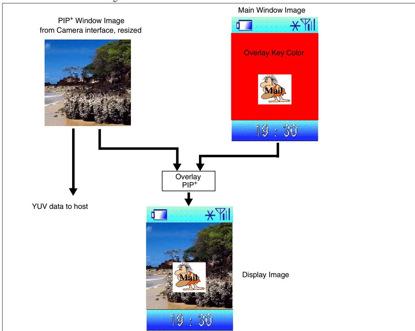
Figure 8-7: Main Window, PIP+ Window, Overlay, and YUV
