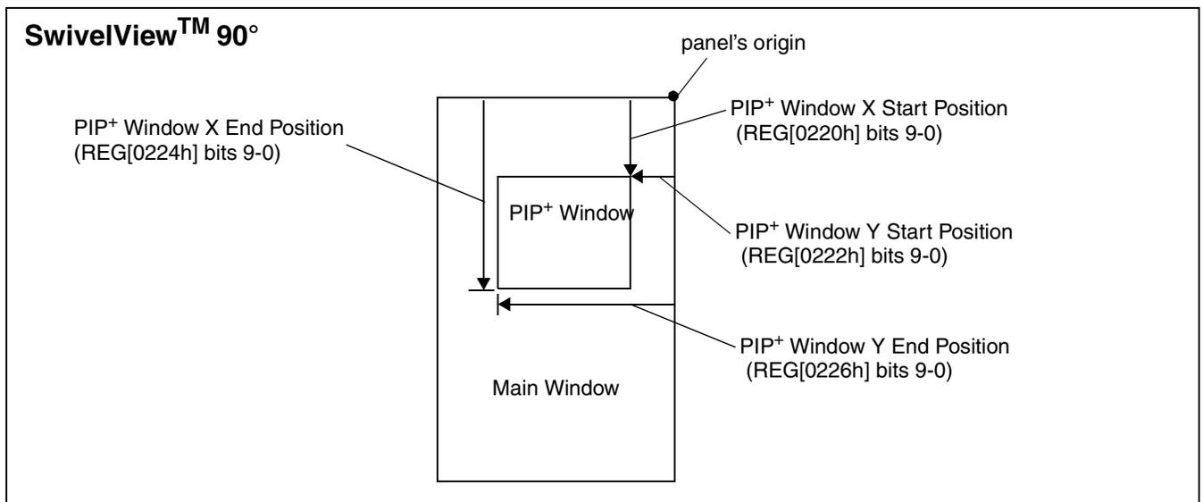
Figure 15-2: PIP<sup>+</sup> with SwivelView 90° Enabled
