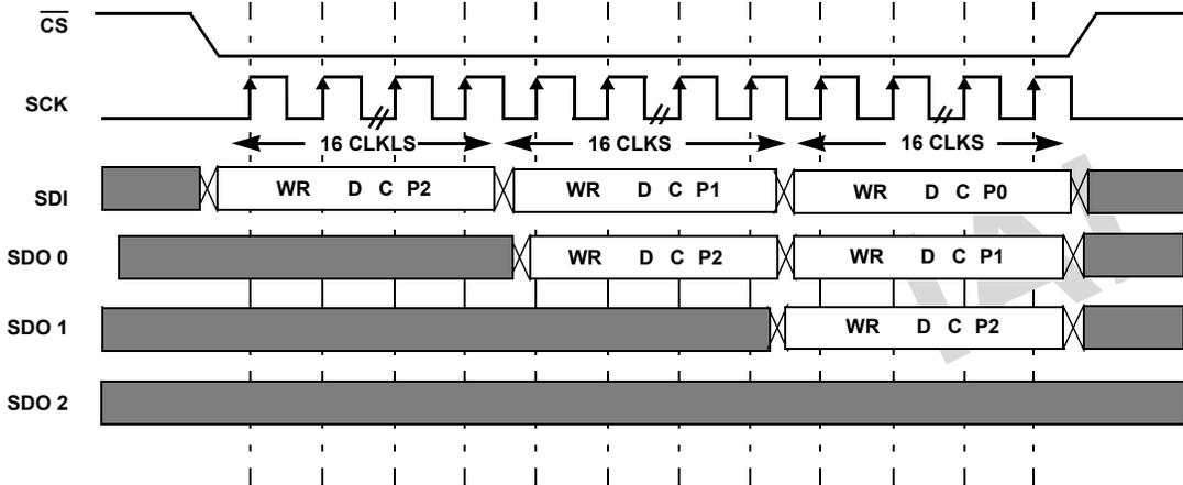
FIGURE 19. DAISY CHAIN WRITE SEQUENCE OF N = 3 DCP
