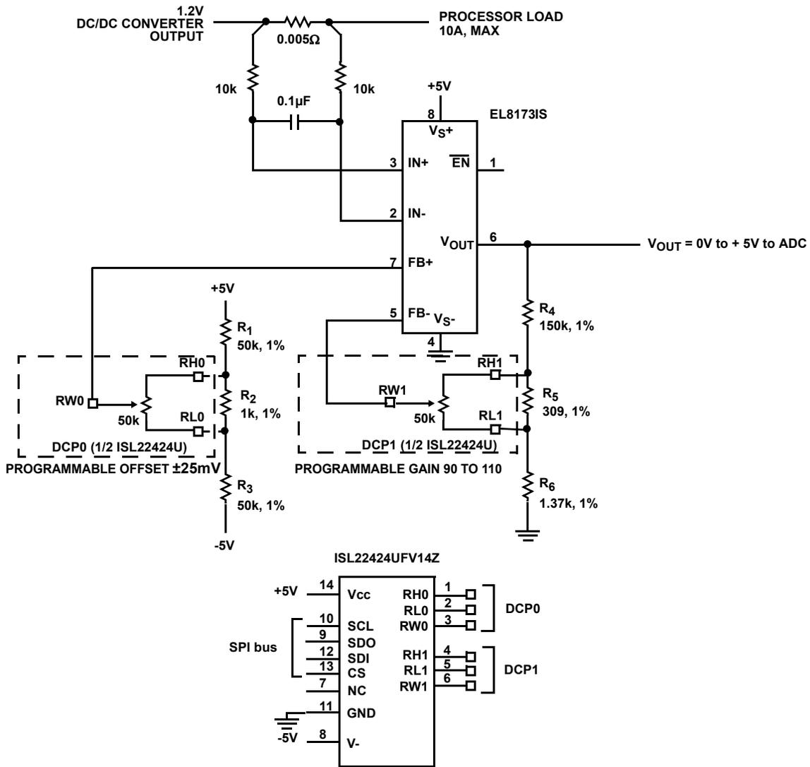
FIGURE 22. CURRENT SENSING WITH GAIN AND OFFSET CONTROL
