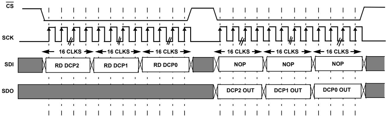
FIGURE 21. DAISY CHAIN READ SEQUENCE OF N = 3 DCP
