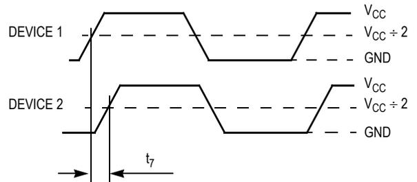
Figure 4. Device-to-Device Skew
