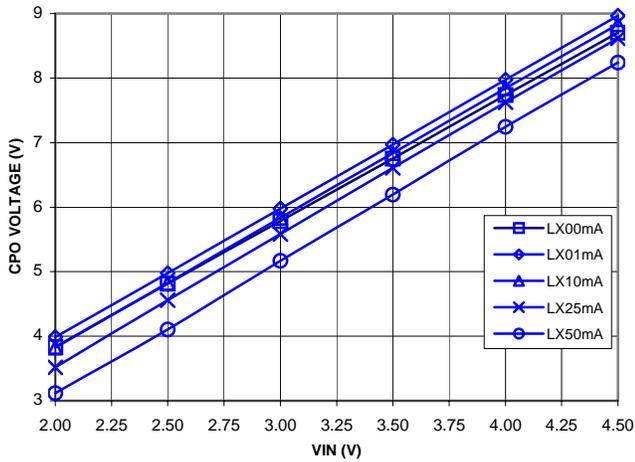
**Figure 11 – CPO Voltage vs. Input Voltage;**
