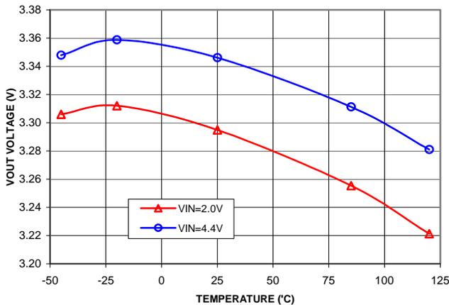
**Figure 9 – LX1882-33 Output Voltage vs. Temperature;**
