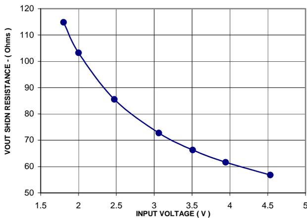
**Figure 13 –  $V_{\text{OUT}}$  Shutdown Resistance vs. Input Voltage;**
