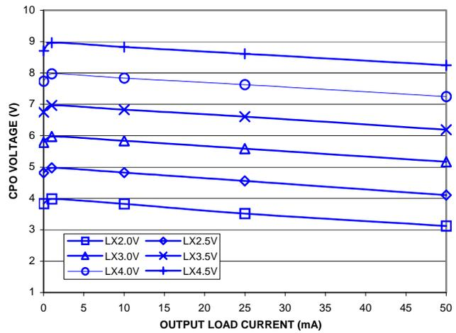
**Figure 12 – CPO Voltage vs. Load Current;**
