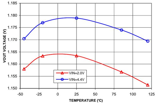
**Figure 10 – LX1882-00 Output Voltage vs. Temperature;**
