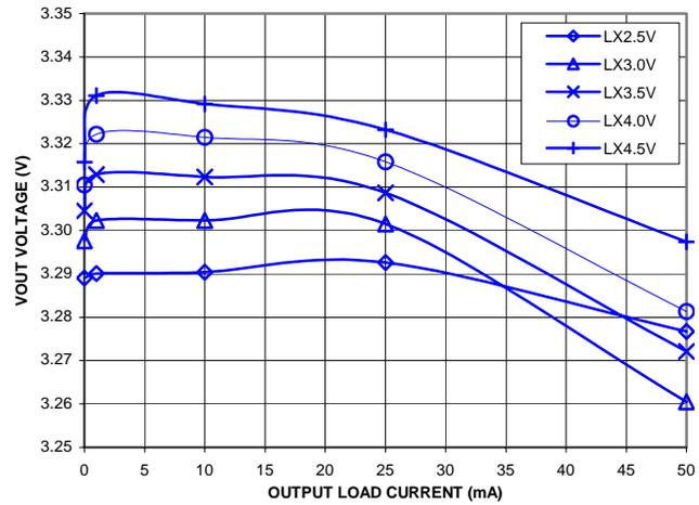
**Figure 8 – LX1882-33 Output Voltage vs. Load Current;**
