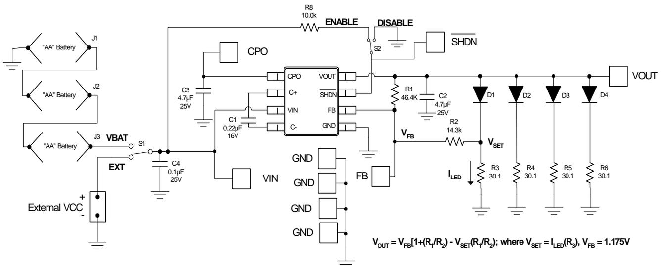
Figure 6 – LX1882-00 Evaluation Board Schematic; LED Driver Application
