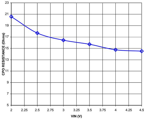
**Figure 7 – CPO Output Resistance vs. Input Voltage;**
