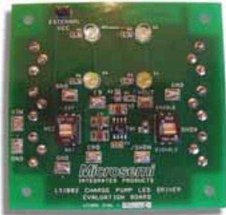
**Figure 4.** LX1882 LED Driver Evaluation Board (Top View)
