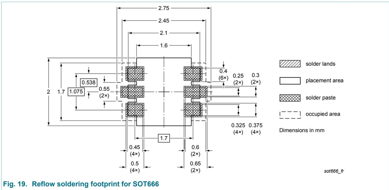
Fig. 19. Reflow soldering footprint for SOT666
