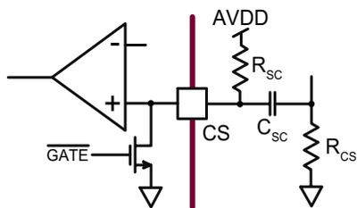
Figure 1: Slope Compensation
