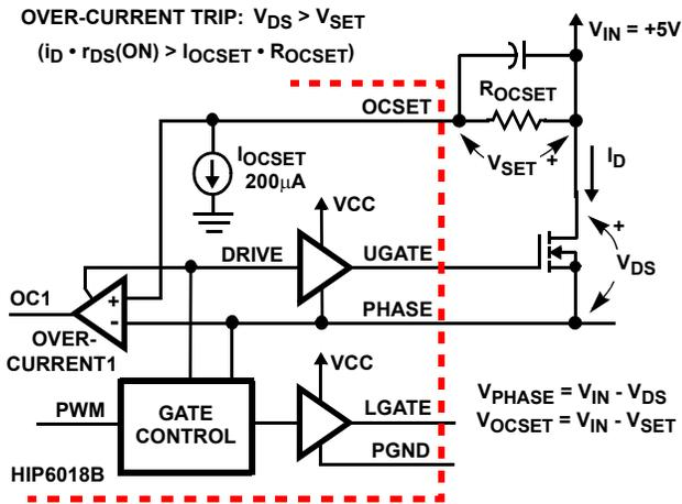
FIGURE 9. OVER-CURRENT DETECTION
