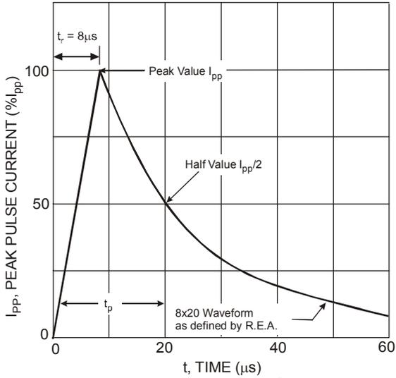
Figure 3 Pulse Waveform
