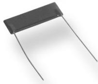
The HBS is a high voltage plate resistor offering resistance values up to 1 Teraohm and working voltages up to 30 KV. A tough lacquer coating encapsulates the product so that excellent TCR's and VCR's are maintained. This is a sister product to the HB Series, effectively extending the value range that is available. Further options are also available with the ability to produce custom designs relatively quickly where quantities justify.
