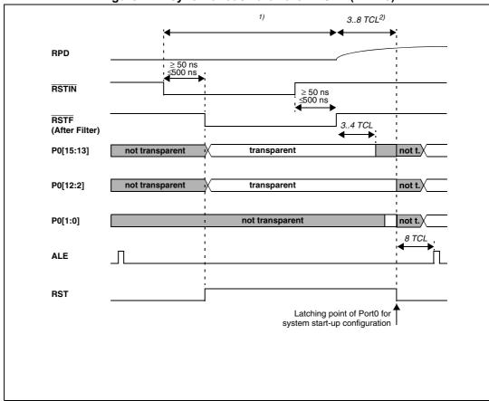
Figure 27. Asynchronous hardware RESET (EA = 0)
