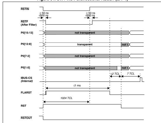
Figure 34. SW / WDT bidirectional RESET (EA=1)
