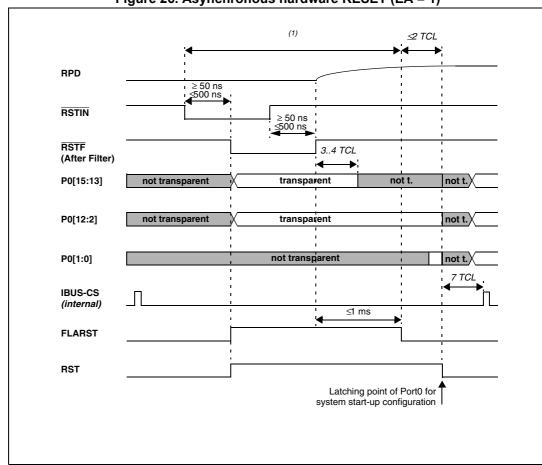
Figure 26. Asynchronous hardware RESET (EA = 1)
