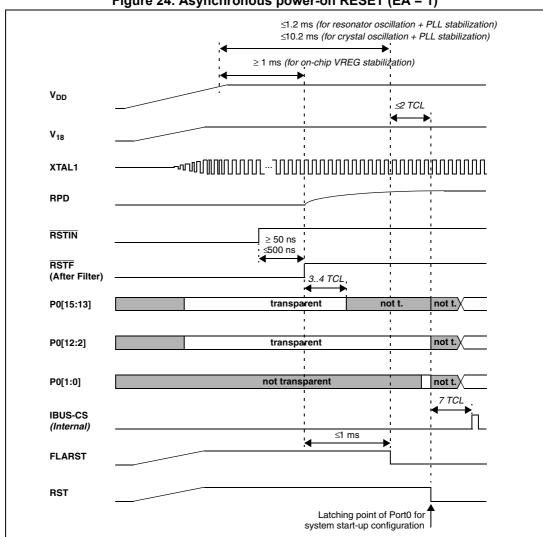
Figure 24. Asynchronous power-on RESET (EA = 1)
