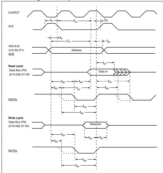
Figure 63. Demultiplexed bus with ALE and R/W CS
