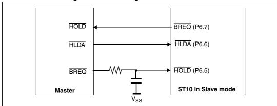
Figure 72. Connecting an ST10 in slave mode
