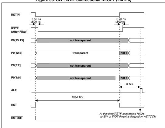
Figure 35. SW / WDT bidirectional RESET ( $\overline{EA} = 0$ )
