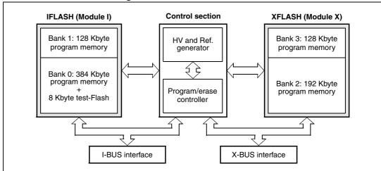
Figure 4. Flash modules structure
