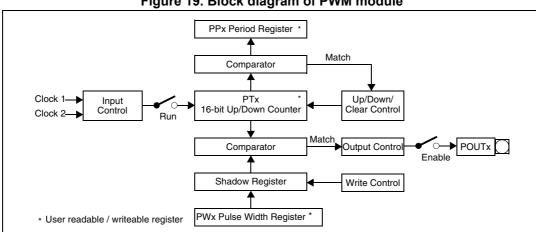
Figure 19. Block diagram of PWM module
