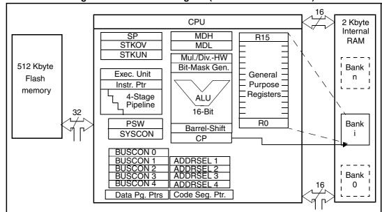
Figure 14. CPU Block Diagram (MAC Unit not included)
