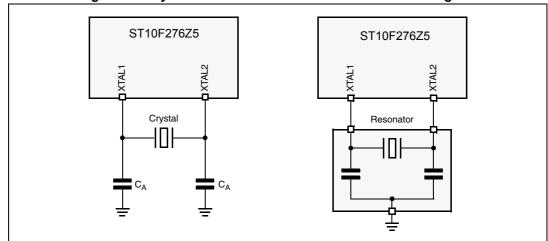
Figure 54. Crystal oscillator and resonator connection diagram
