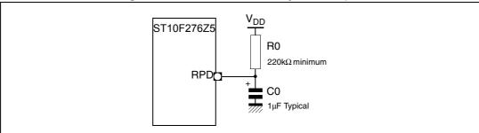
Figure 43. External RC circuitry on RPD pin
