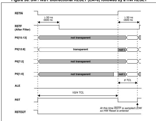
Figure 36. SW / WDT bidirectional RESET (EA=0) followed by a HW RESET
