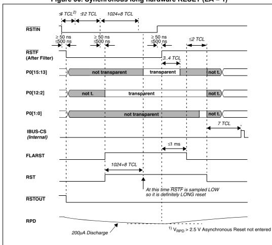
Figure 30. Synchronous long hardware RESET (EA = 1)
