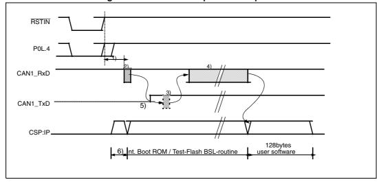
Figure 11. CAN bootstrap loader sequence
