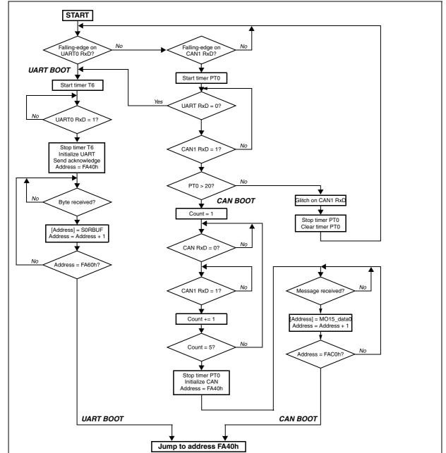
Figure 5. ST10F276Z5 new standard bootstrap loader program flow
