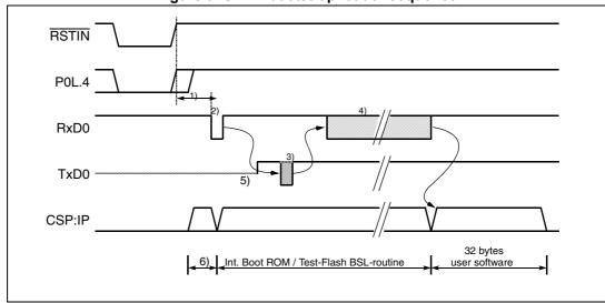
Figure 9. UART bootstrap loader sequence
