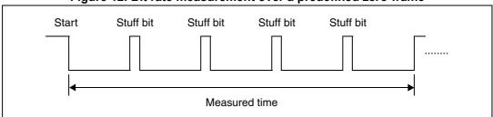
Figure 12. Bit rate measurement over a predefined zero-frame
