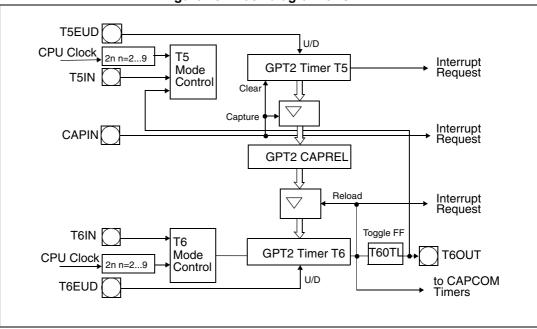
Figure 18. Block diagram of GPT2
