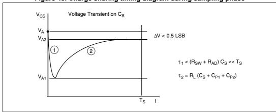
Figure 48. Charge sharing timing diagram during sampling phase
