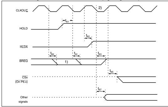
Figure 67. External bus arbitration (regaining the bus)
