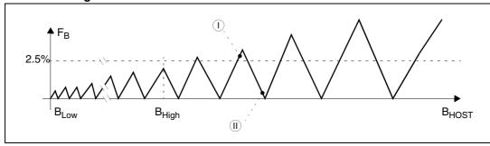
Figure 10. Baud rate deviation between host and ST10F276Z5
