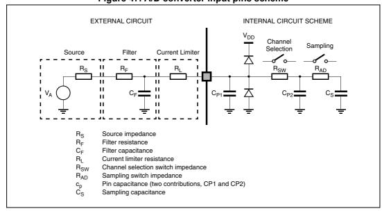
Figure 47. A/D converter input pins scheme
