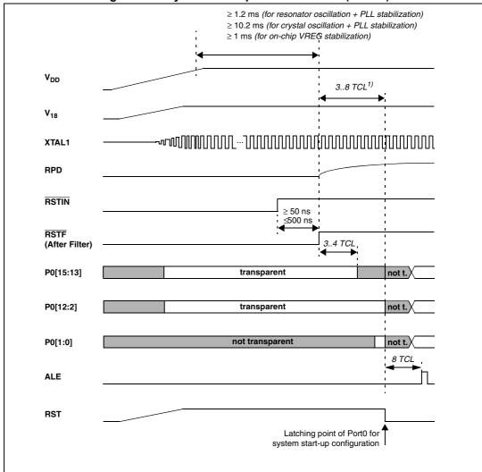
Figure 25. Asynchronous power-on RESET ( $\overline{EA} = 0$ )
