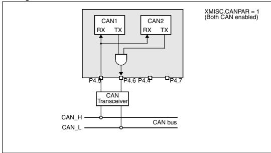
P4.4 and P4.7 when not used as CAN functions can be used as general purpose I/O while they cannot be used as external bus address lines.
