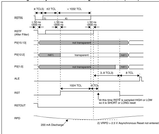
Figure 29. Synchronous short / long hardware RESET ( $\overline{EA} = 0$ )
