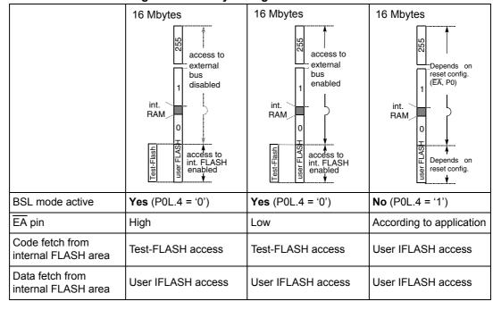
Figure 8. Memory configuration after reset
