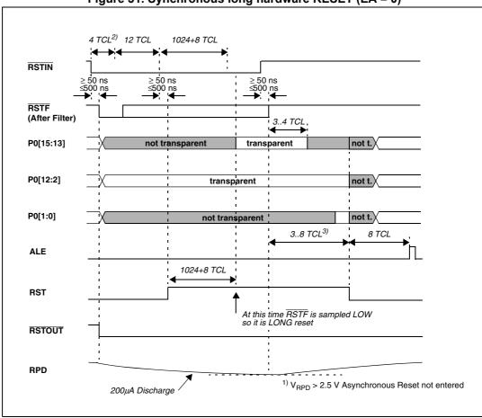
Figure 31. Synchronous long hardware RESET ( $\overline{EA} = 0$ )
