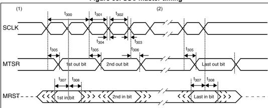
Figure 68. SSC master timing
