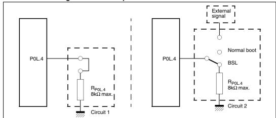
Figure 7. Hardware provisions to activate the BSL
