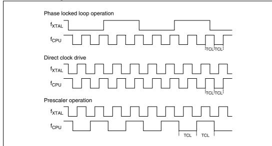
Figure 52. Generation mechanisms for the CPU clock
