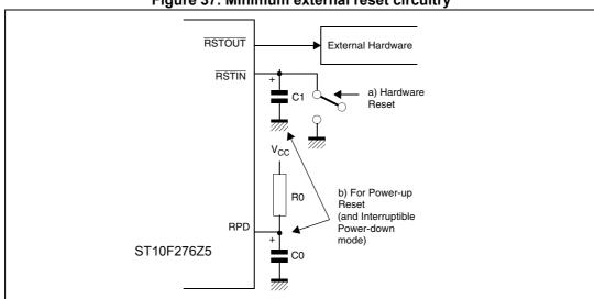
Figure 37. Minimum external reset circuitry
