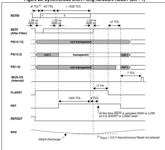
Figure 28. Synchronous short / long hardware RESET ( $\overline{EA} = 1$ )
