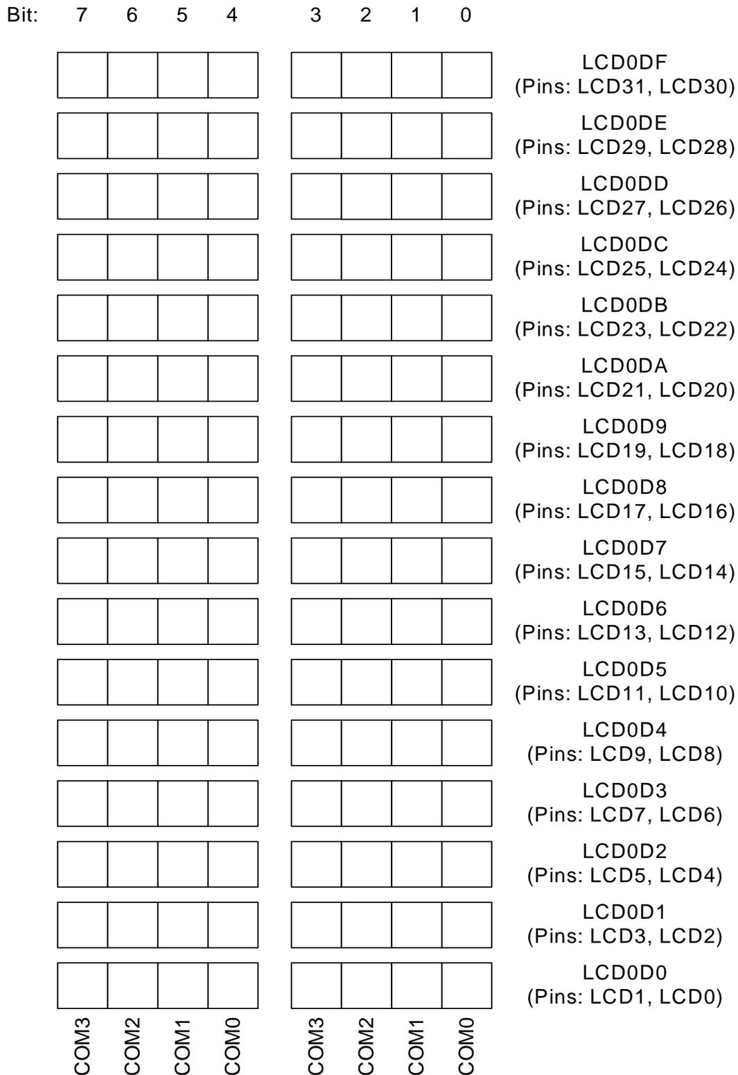
Figure 26.2. LCD Data Register to LCD Pin Mapping
