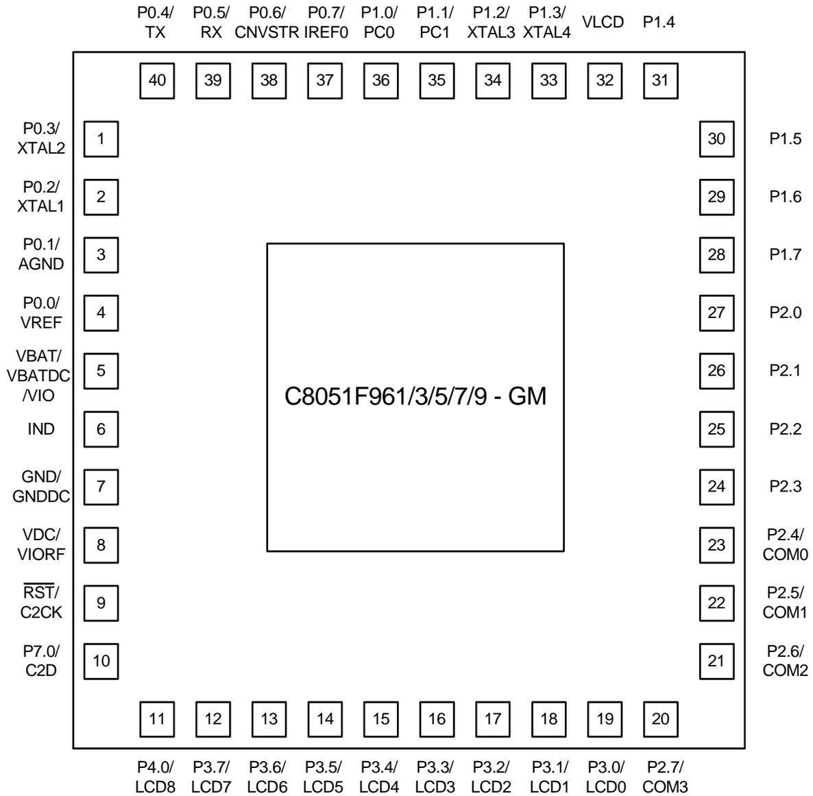
**Figure 3.2. QFN-40 Pinout Diagram (Top View)**
