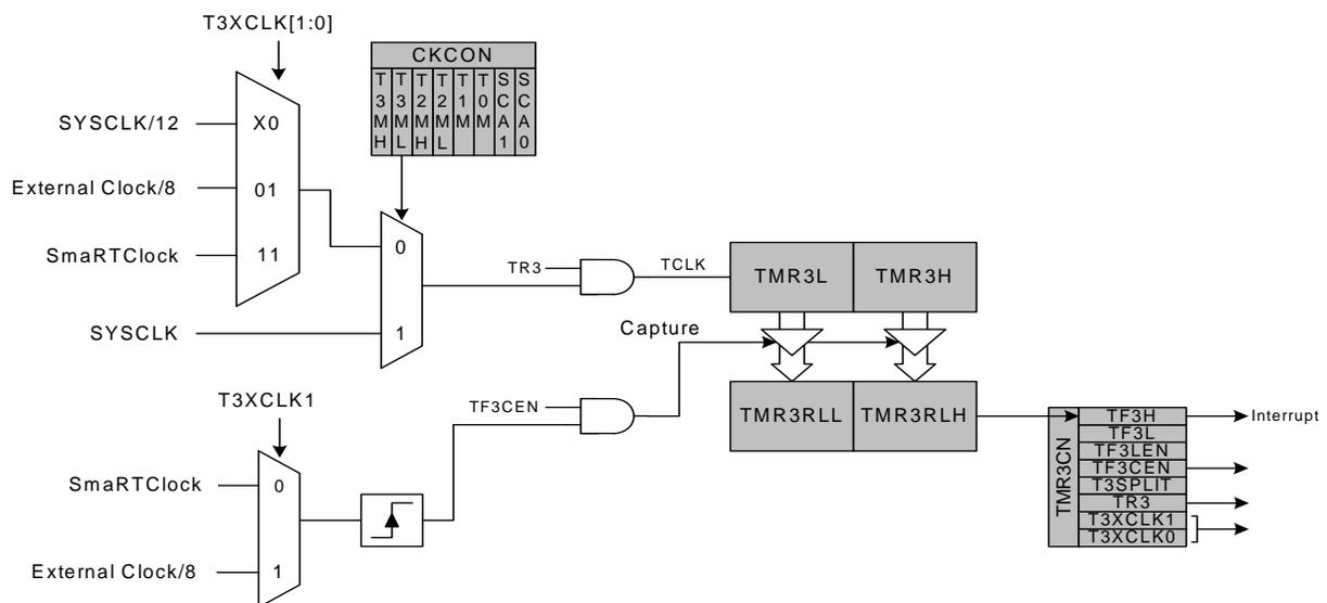
**Figure 32.9. Timer 3 Capture Mode Block Diagram**
