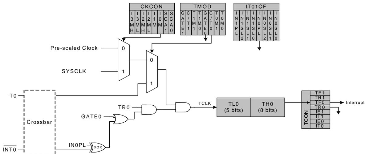
**Figure 32.1. T0 Mode 0 Block Diagram**
