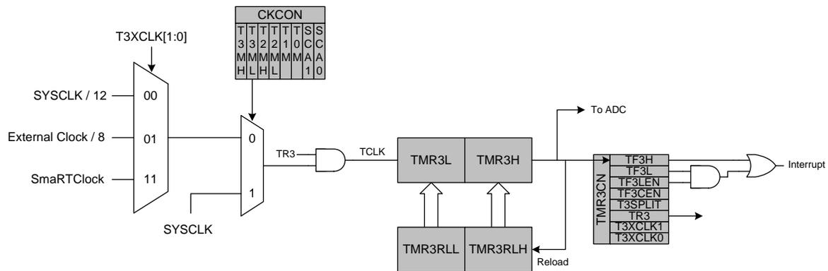
Figure 32.7. Timer 3 16-Bit Mode Block Diagram
