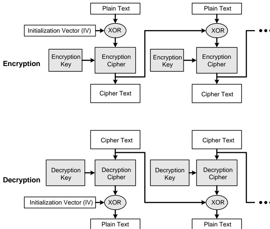
Figure 14.4. Cipher Block Chaining Mode
