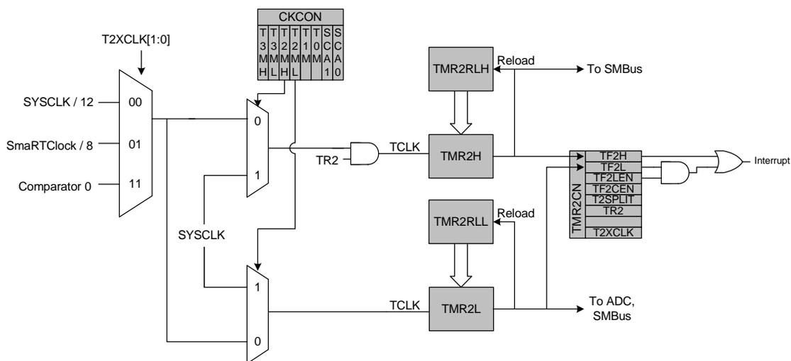
Figure 32.5. Timer 2 8-Bit Mode Block Diagram
