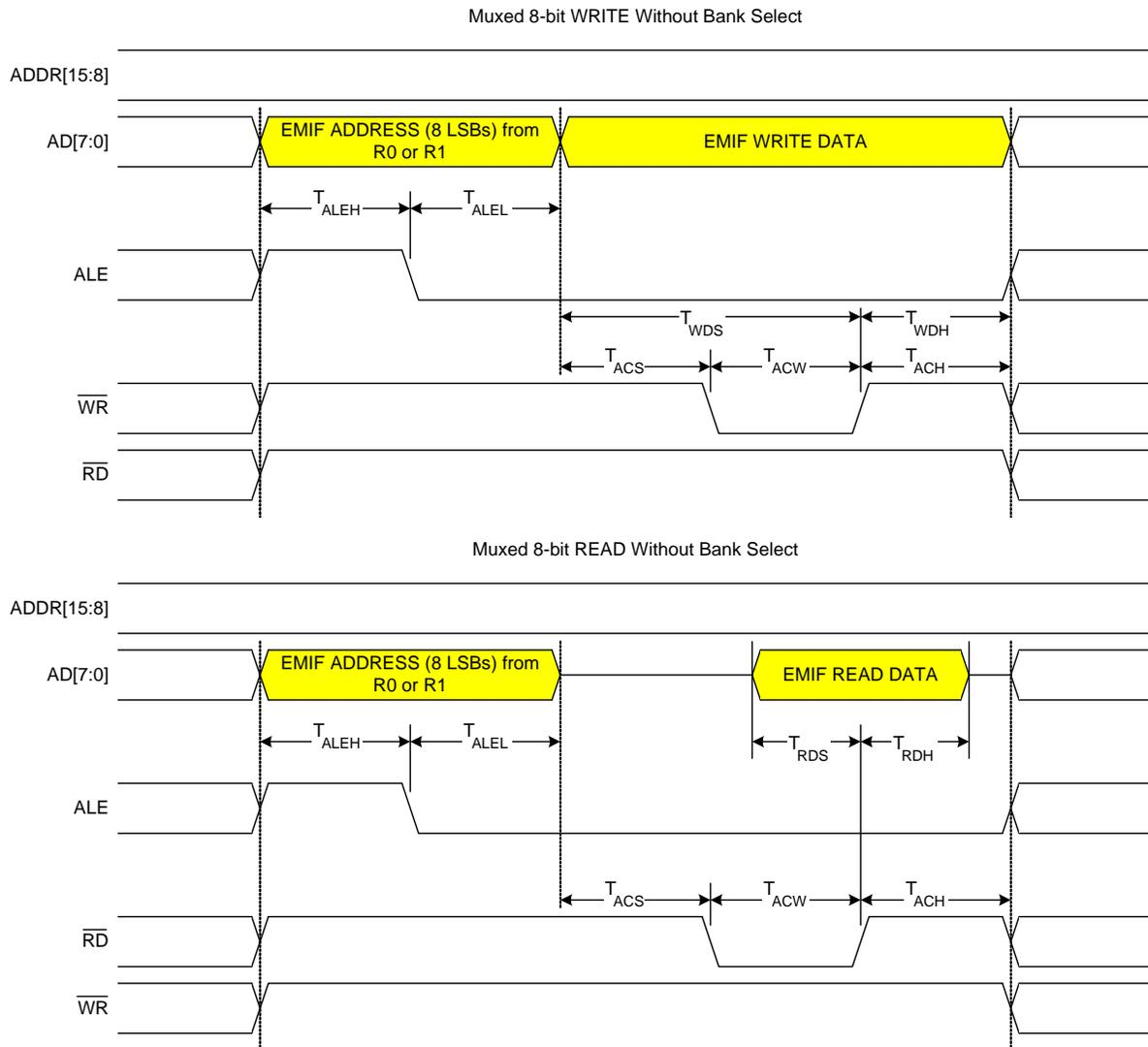
**Figure 10.8. Multiplexed 8-bit MOVX without Bank Select Timing**
