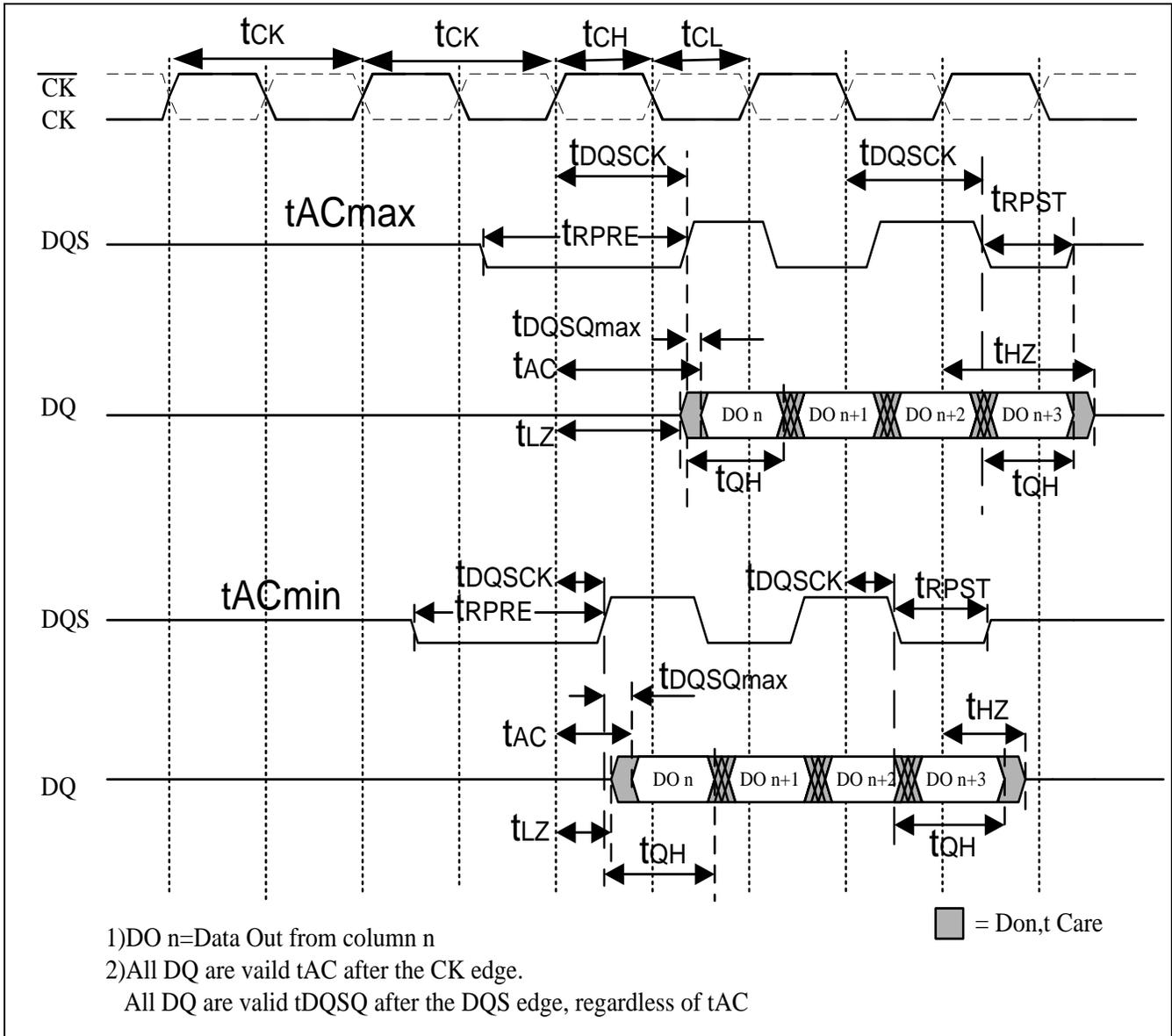
During Read bursts, DQS is driven by the LPDDR SDRAM along with the output data. The initial Low state of the DQS is known as the read preamble; the Low state coincident with last data-out element is known as the read post-amble. The first data-out element is edge aligned with the first rising edge of DQS and the successive data-out elements are edge aligned to successive edges of DQS. This is shown in following figure with a CAS latency of 2 and 3.
