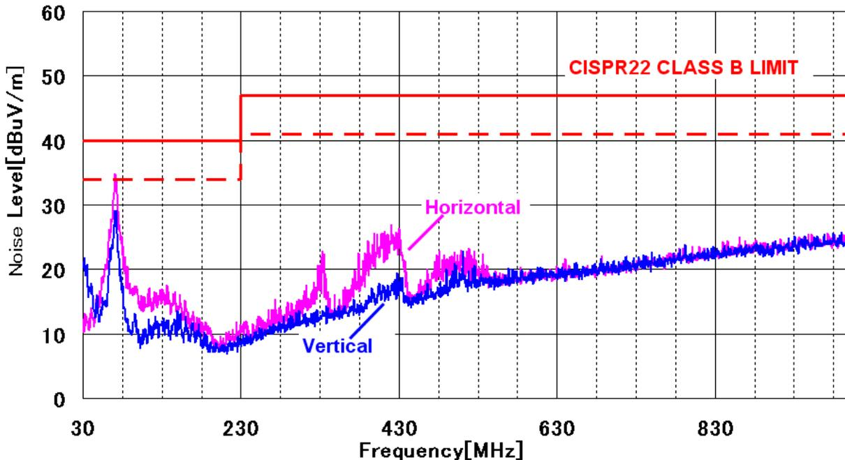
**Figure 4: EMI Test Data of MP7752 EVB**
