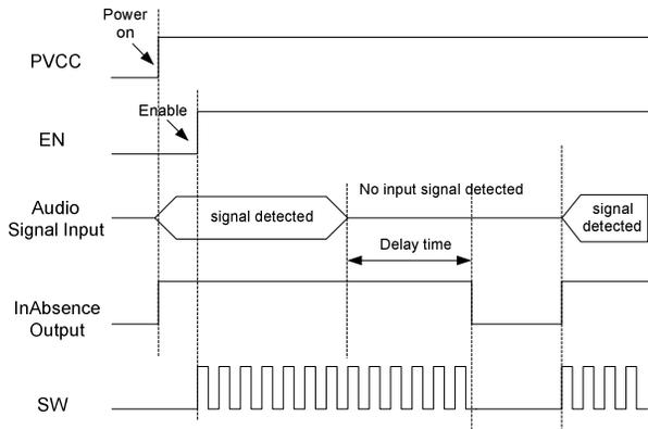
Figure 1b: enable on with audio signal present
