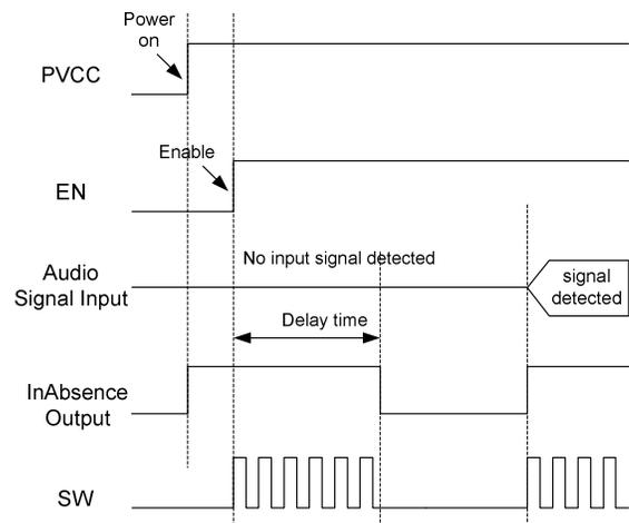
**Figure 1a: enable on with no signal detected**
