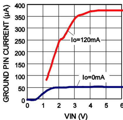
**Ground Pin Current vs. Output Current**
