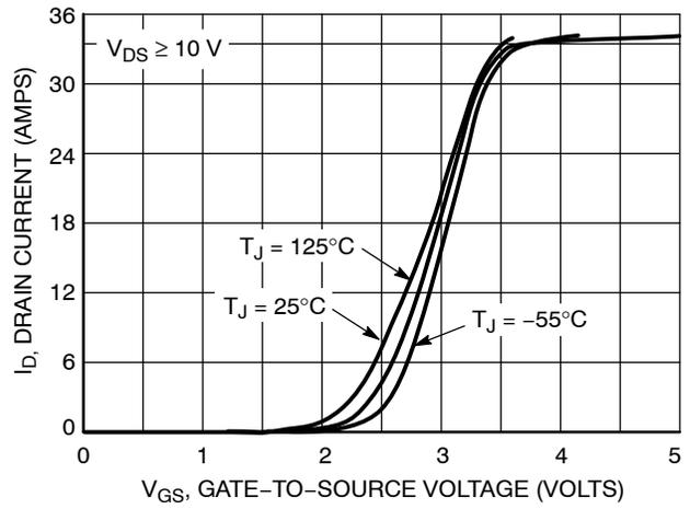
Figure 2. Transfer Characteristics
