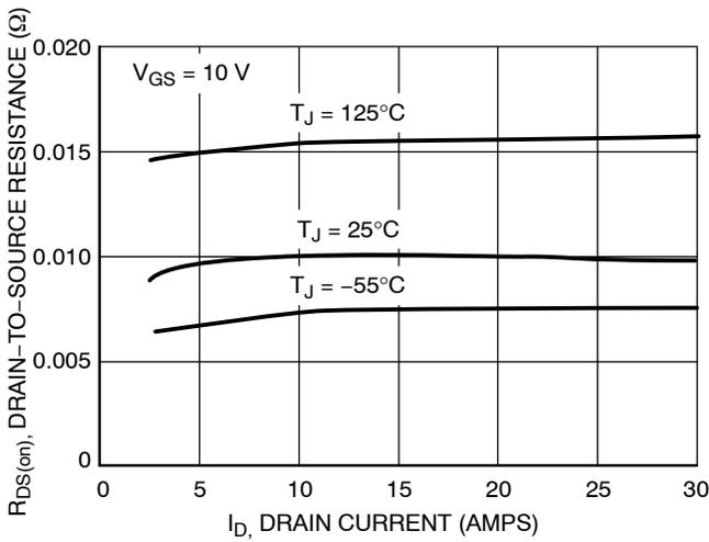
Figure 3. On-Resistance vs. Drain Current and Temperature
