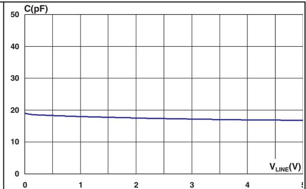
Figure 11. Junction capacitance versus reverse applied voltage (typical values, reverse)
