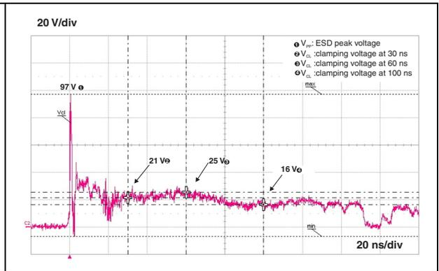
Figure 13. ESD response to IEC 61000-4-2 (-30 kV contact discharge)
