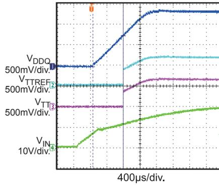
**V<sub>TT</sub>&V<sub>TTREF</sub> Shutdown through V<sub>IN</sub>**
