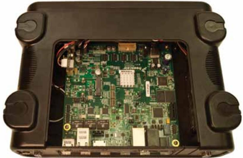
The P1010 RDB platform features 1 GB of DDR3 SDRAM, 32 MB NOR flash and 32 MB NAND flash, and can boot securely from either NOR or NAND flash memory. Other boot options (i.e. SD/MMC, SPI) also supported. It supports three Gigabit-capable ports via an SGMII or RGMII PHYs, as well as a single-port USB and associated PHY.
