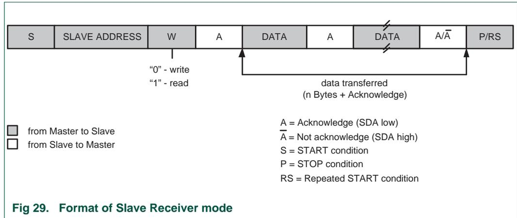
Fig 29. Format of Slave Receiver mode
