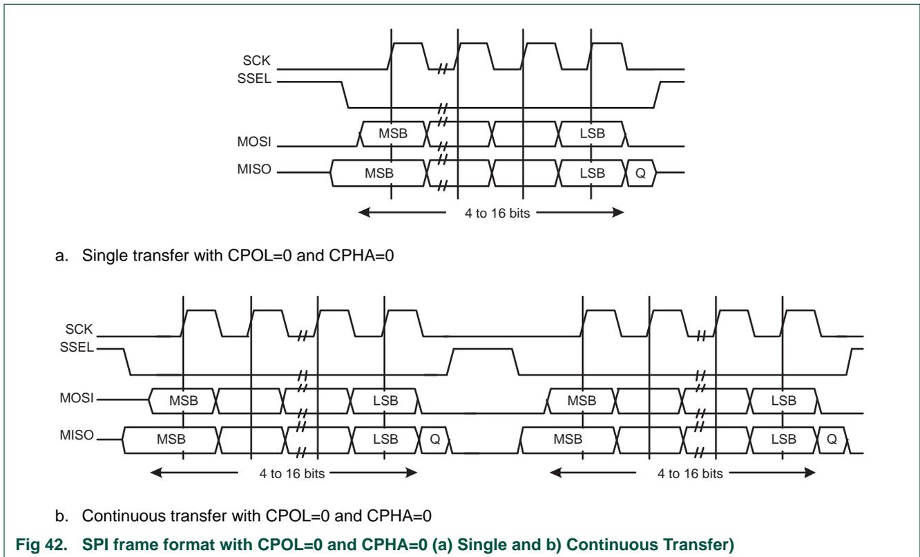
**Fig 42. SPI frame format with CPOL=0 and CPHA=0 (a) Single and b) Continuous Transfer)**
