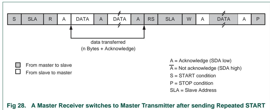
Fig 28. A Master Receiver switches to Master Transmitter after sending Repeated START
