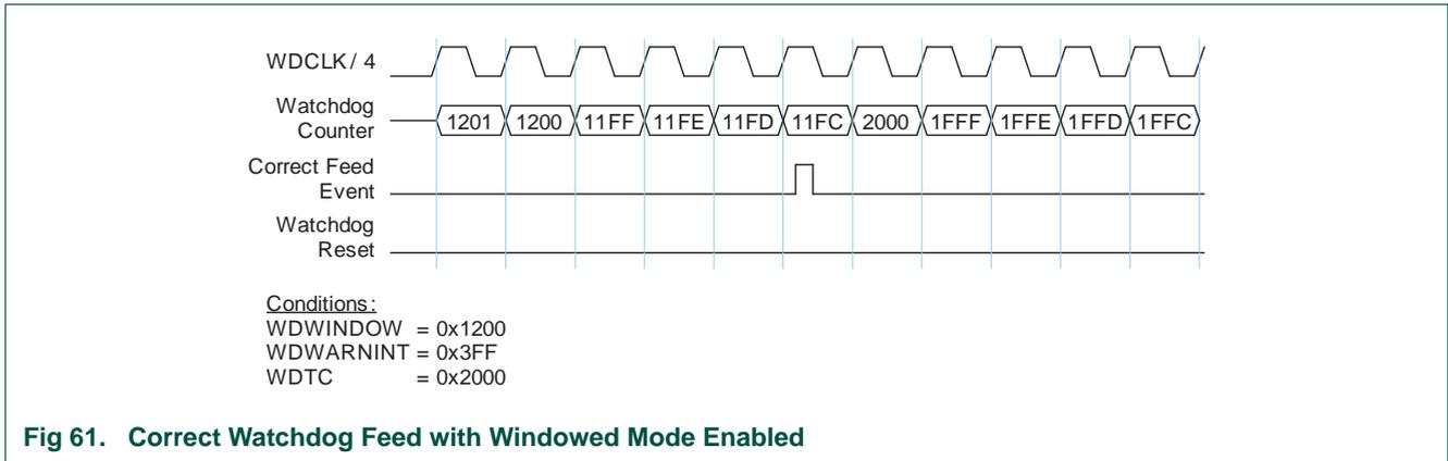
Fig 61. Correct Watchdog Feed with Windowed Mode Enabled
