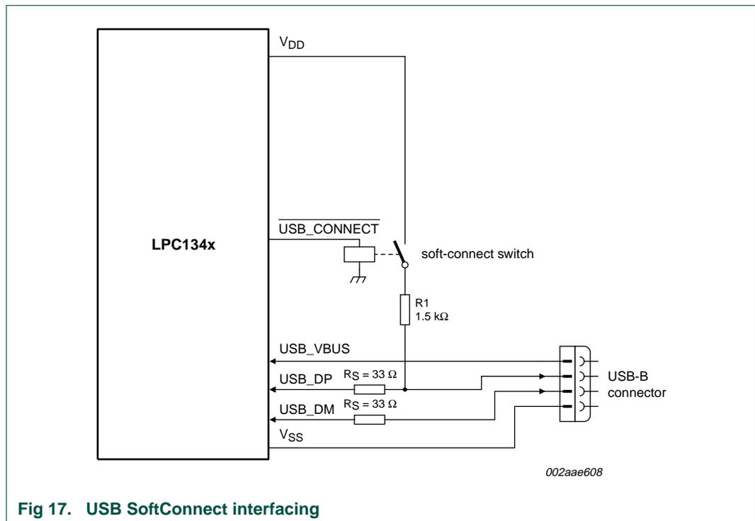
Fig 17. USB SoftConnect interfacing
