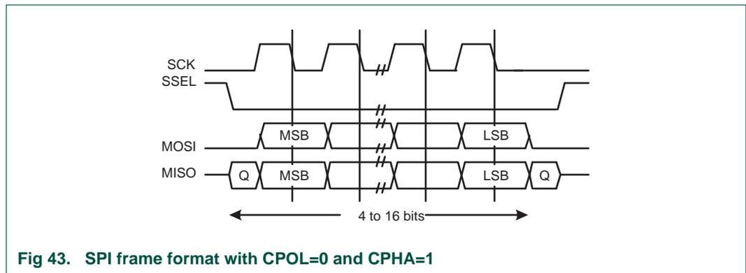
**Fig 43. SPI frame format with CPOL=0 and CPHA=1**
