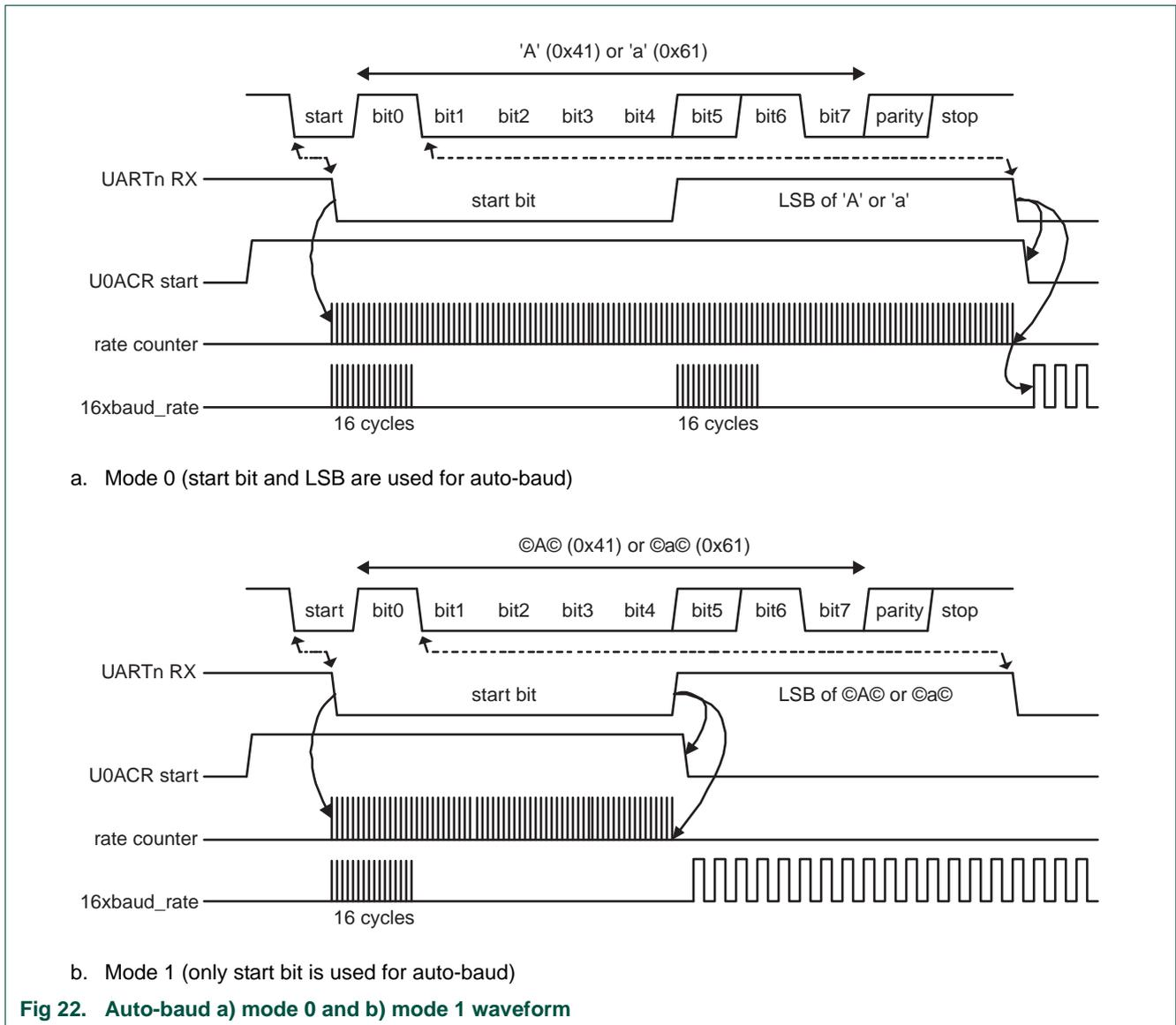
Fig 22. Auto-baud a) mode 0 and b) mode 1 waveform
