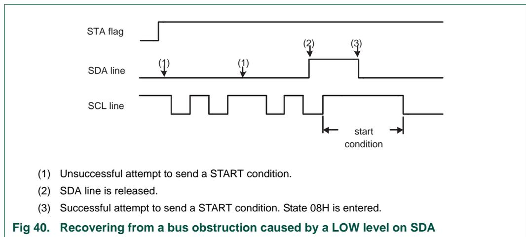
**Fig 40. Recovering from a bus obstruction caused by a LOW level on SDA**
