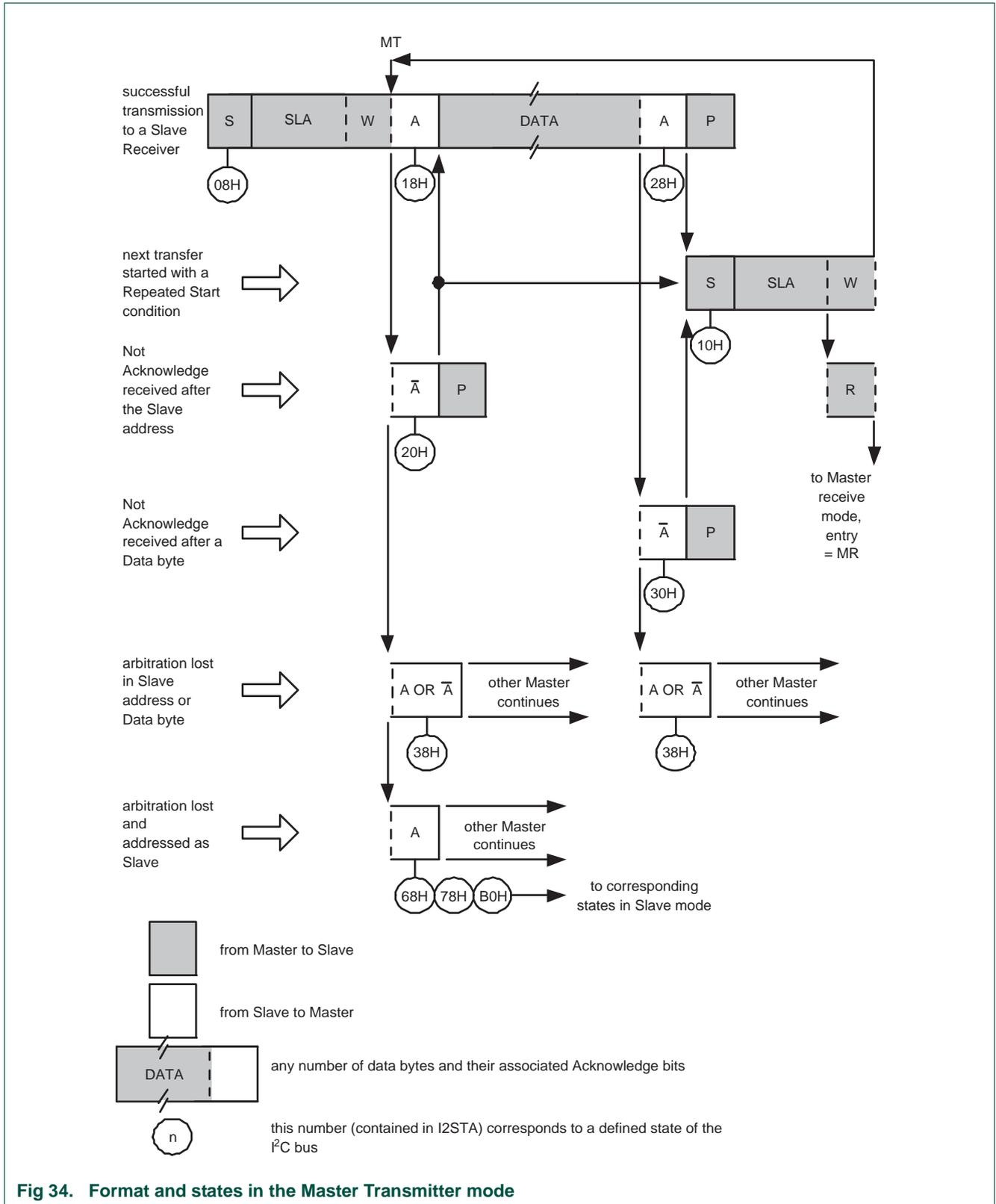
Fig 34. Format and states in the Master Transmitter mode
