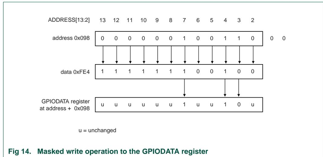
Fig 14. Masked write operation to the GPIODATA register
