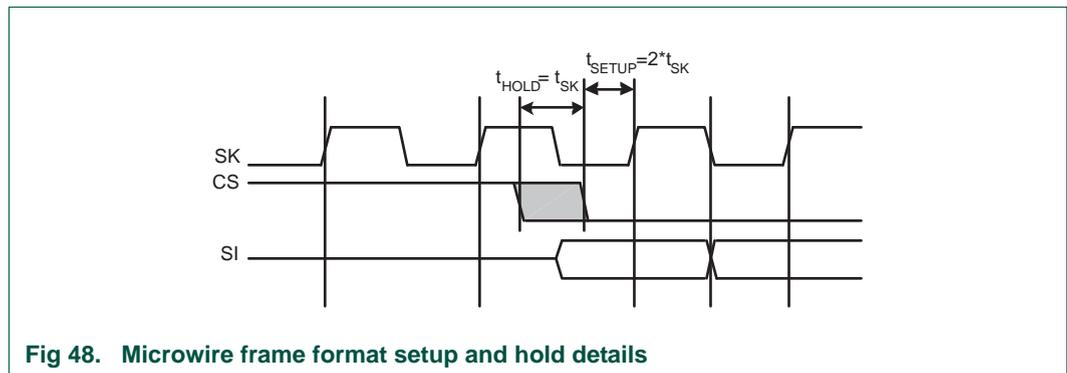
Fig 48. Microwire frame format setup and hold details
