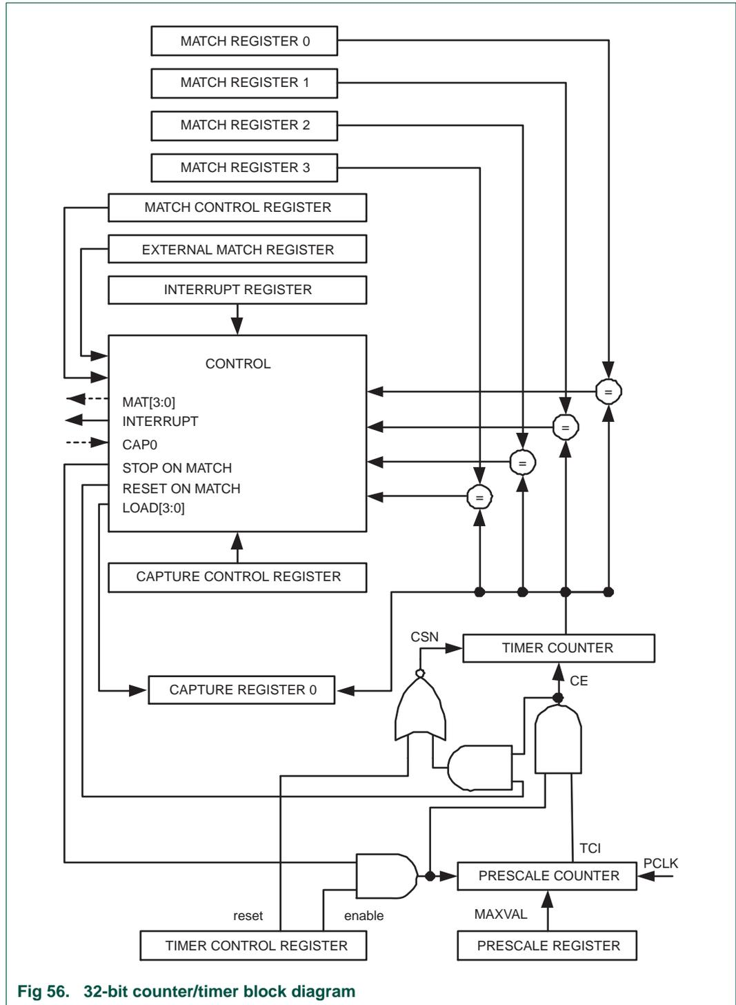
Fig 56. 32-bit counter/timer block diagram
