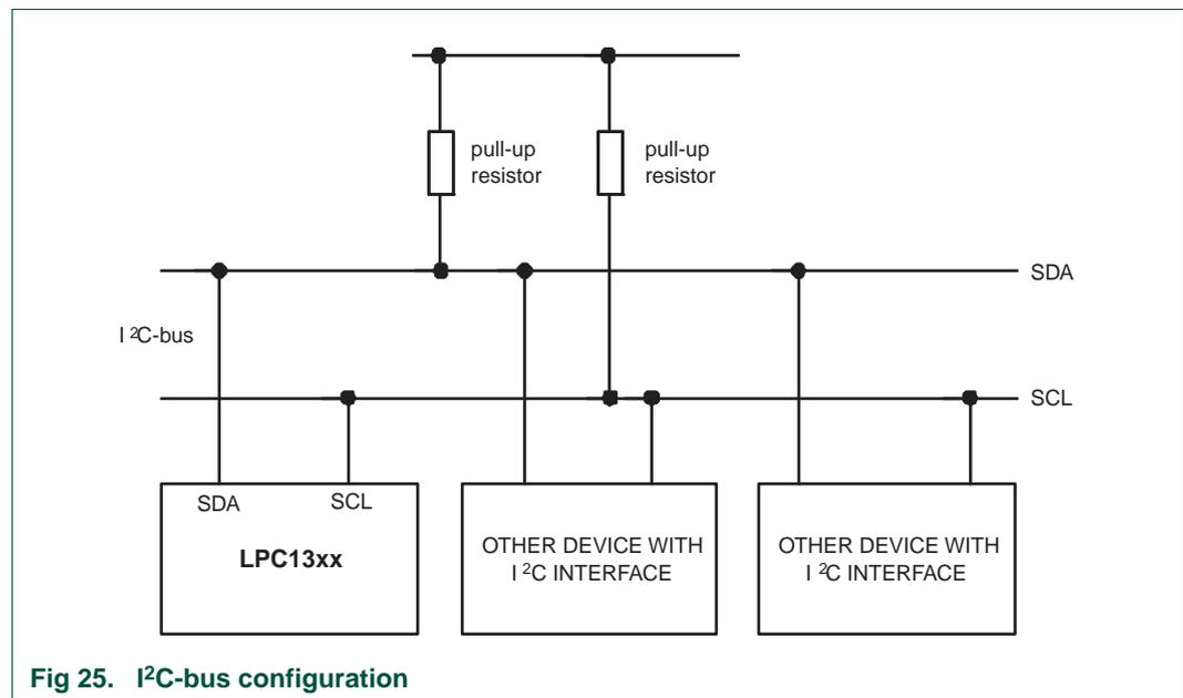
Fig 25. I<sup>2</sup>C-bus configuration
