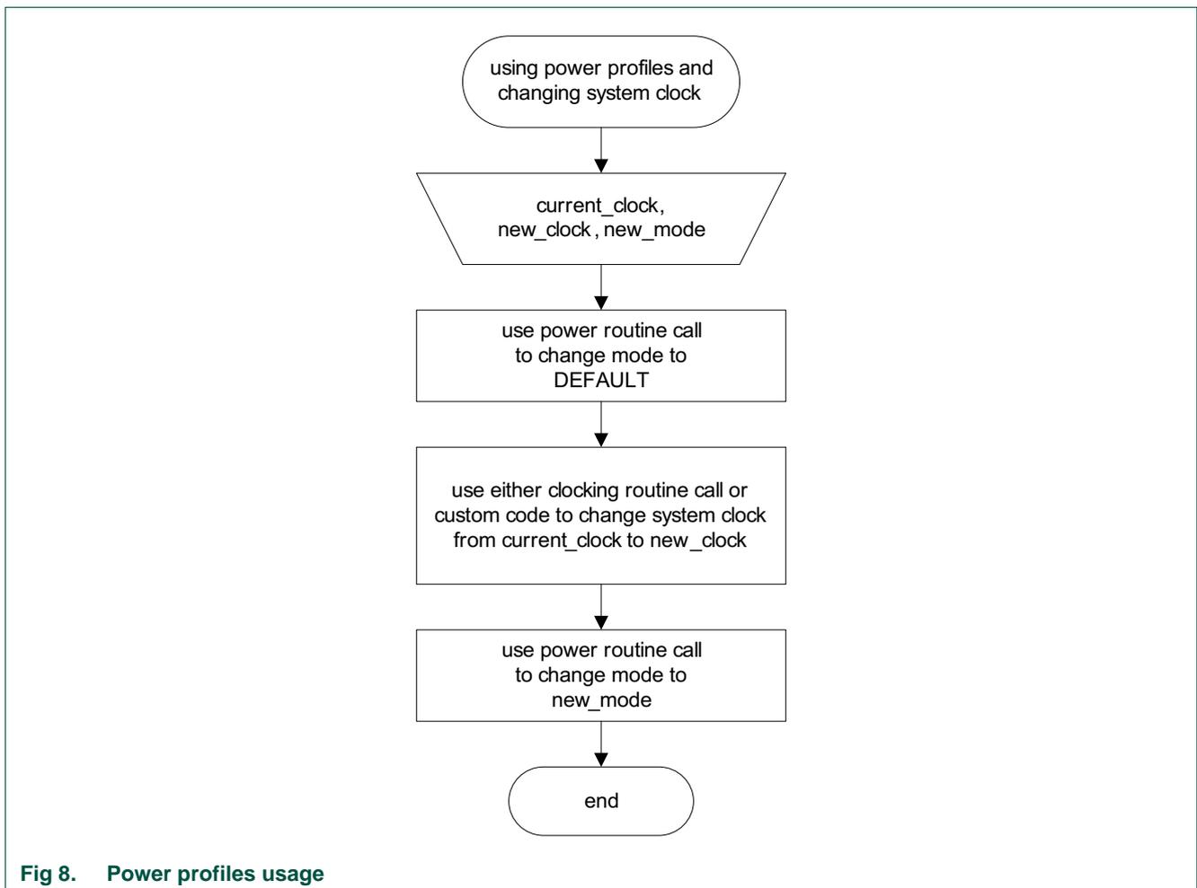
Fig 8. Power profiles usage
