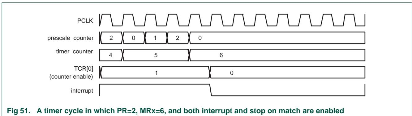
**Fig 51. A timer cycle in which PR=2, MRx=6, and both interrupt and stop on match are enabled**
