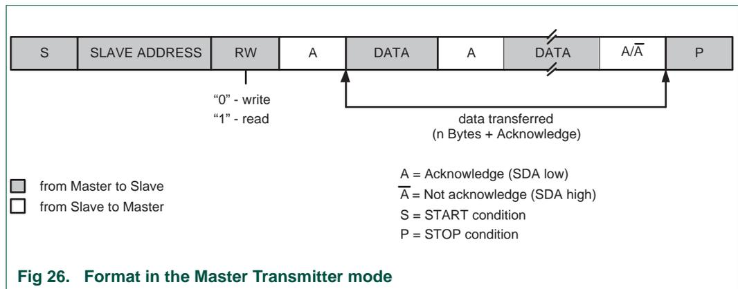
**Fig 26. Format in the Master Transmitter mode**
