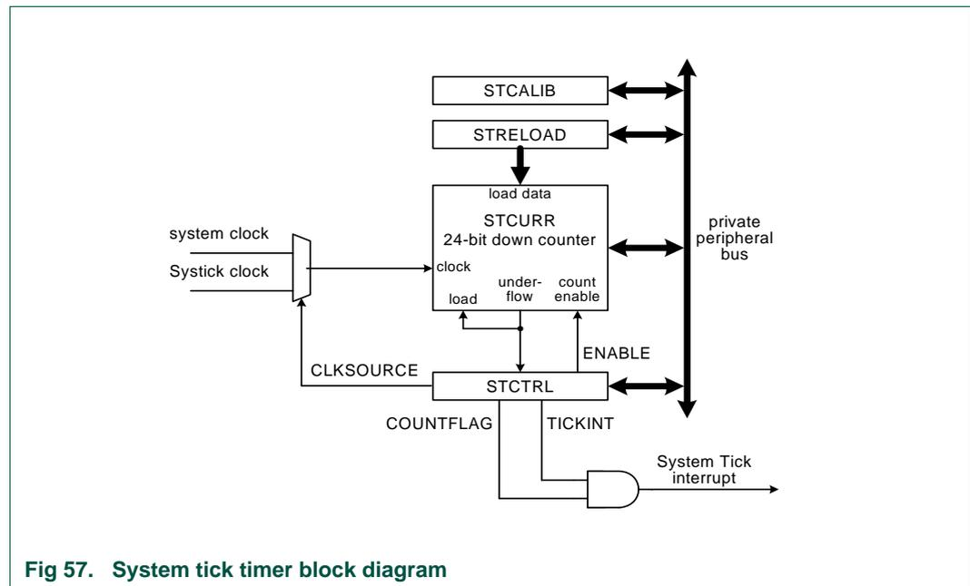
Fig 57. System tick timer block diagram
