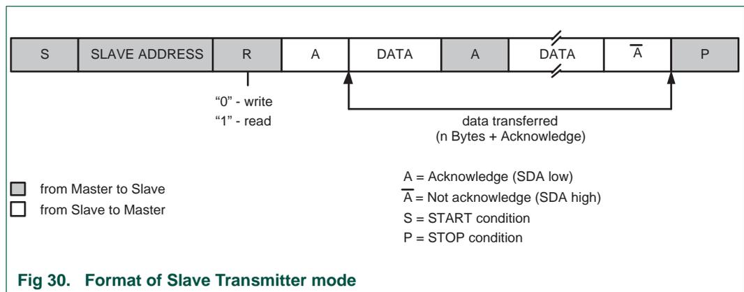
Fig 30. Format of Slave Transmitter mode
