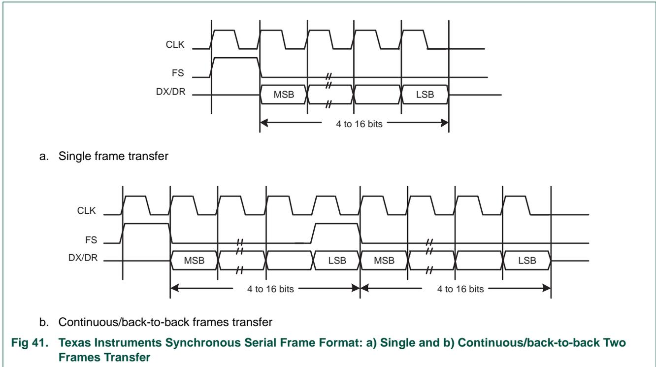
**Fig 41. Texas Instruments Synchronous Serial Frame Format: a) Single and b) Continuous/back-to-back Two Frames Transfer**
