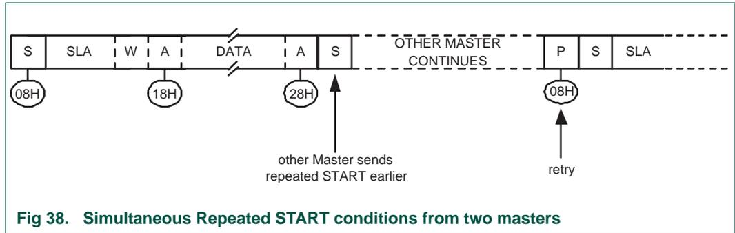
Fig 38. Simultaneous Repeated START conditions from two masters
