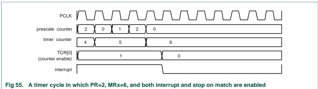
**Fig 55. A timer cycle in which PR=2, MRx=6, and both interrupt and stop on match are enabled**
