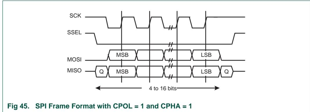
Fig 45. SPI Frame Format with CPOL = 1 and CPHA = 1
