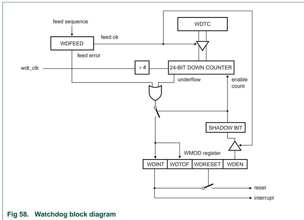
**Fig 58. Watchdog block diagram**
