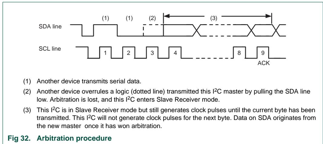
The synchronization logic will synchronize the serial clock generator with the clock pulses on the SCL line from another device. If two or more master devices generate clock pulses, the “mark” duration is determined by the device that generates the shortest “marks,” and the “space” duration is determined by the device that generates the longest “spaces”. [Figure 33](#) shows the synchronization procedure.
