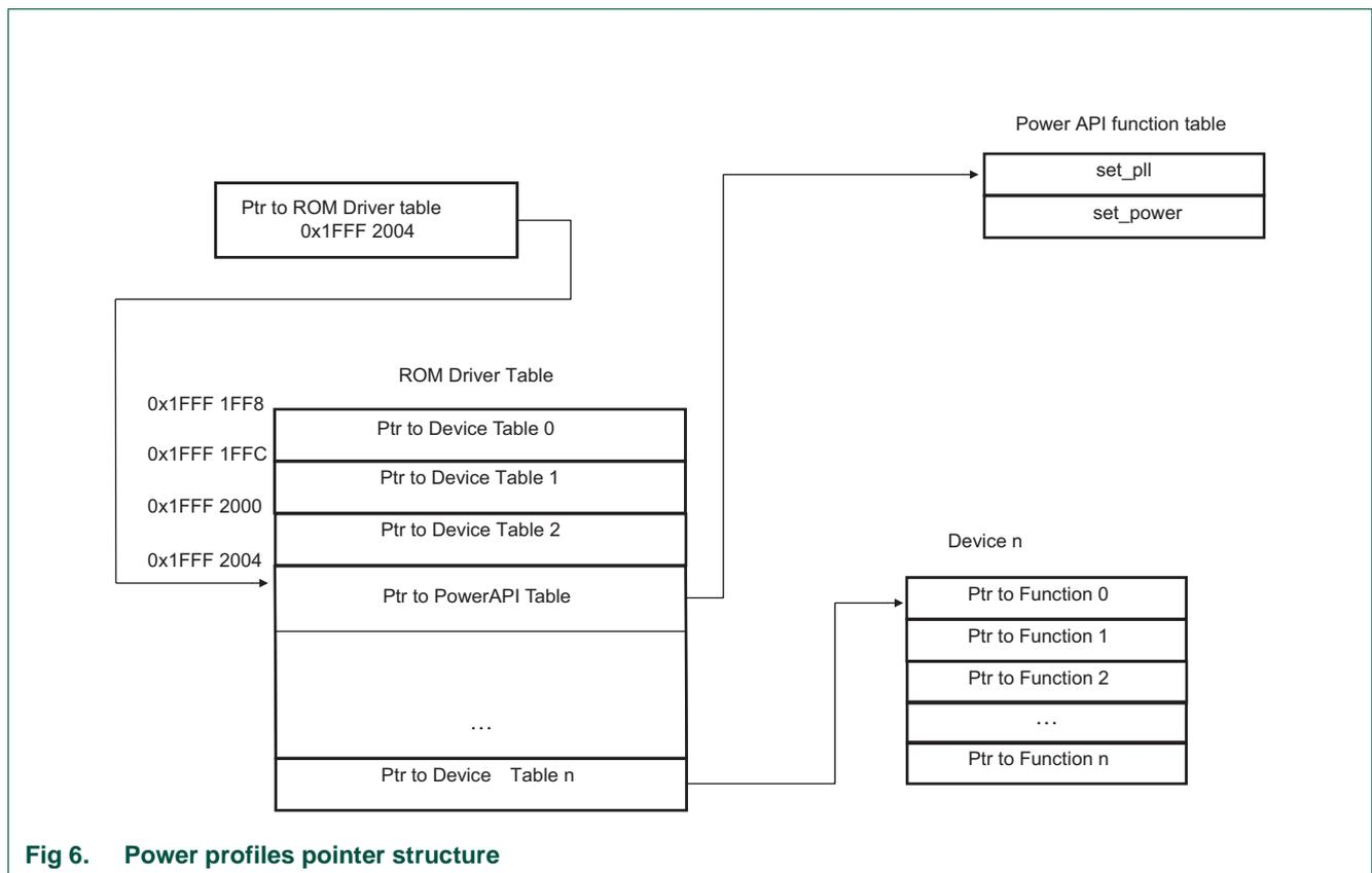
Fig 6. Power profiles pointer structure
