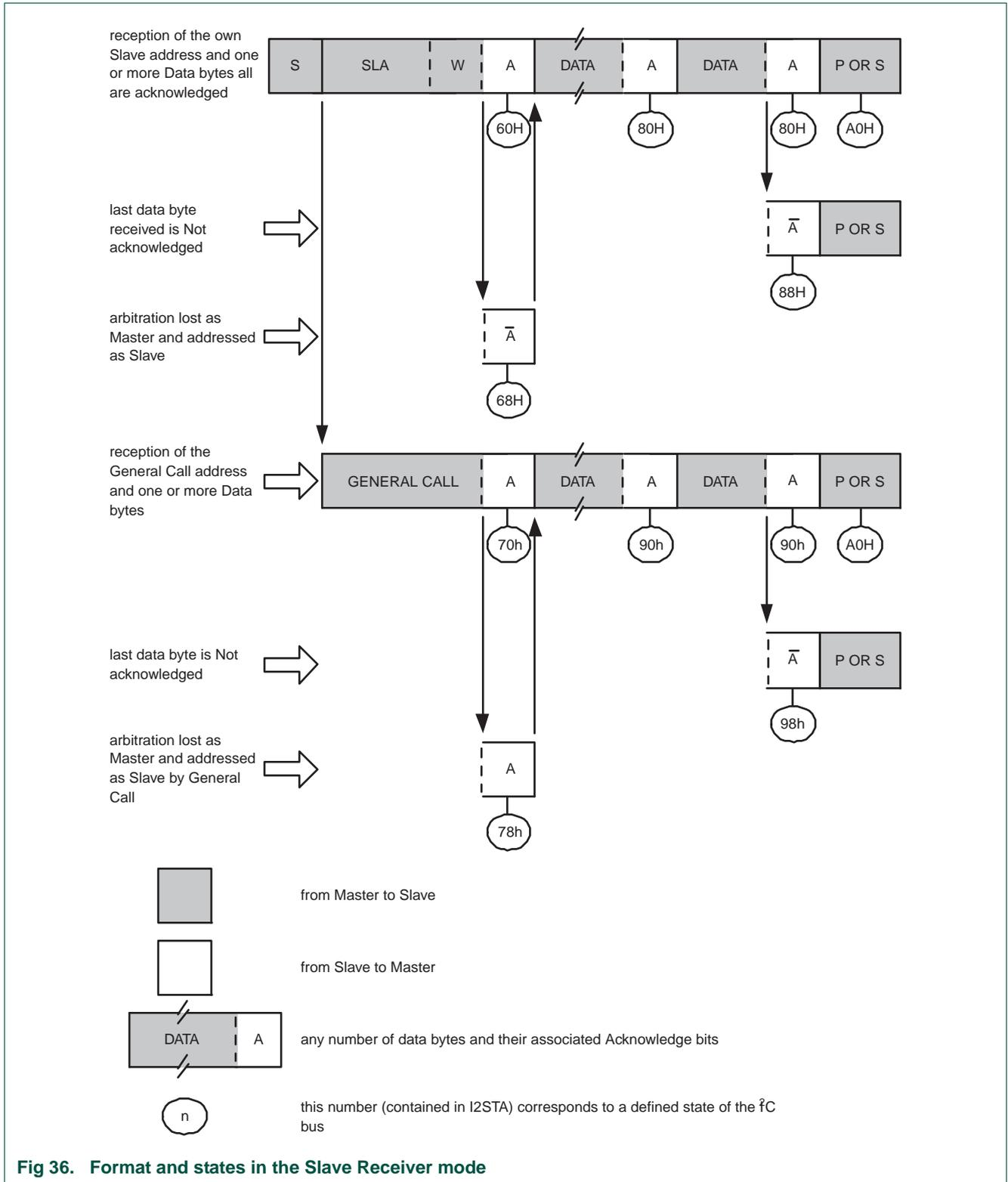
Fig 36. Format and states in the Slave Receiver mode
