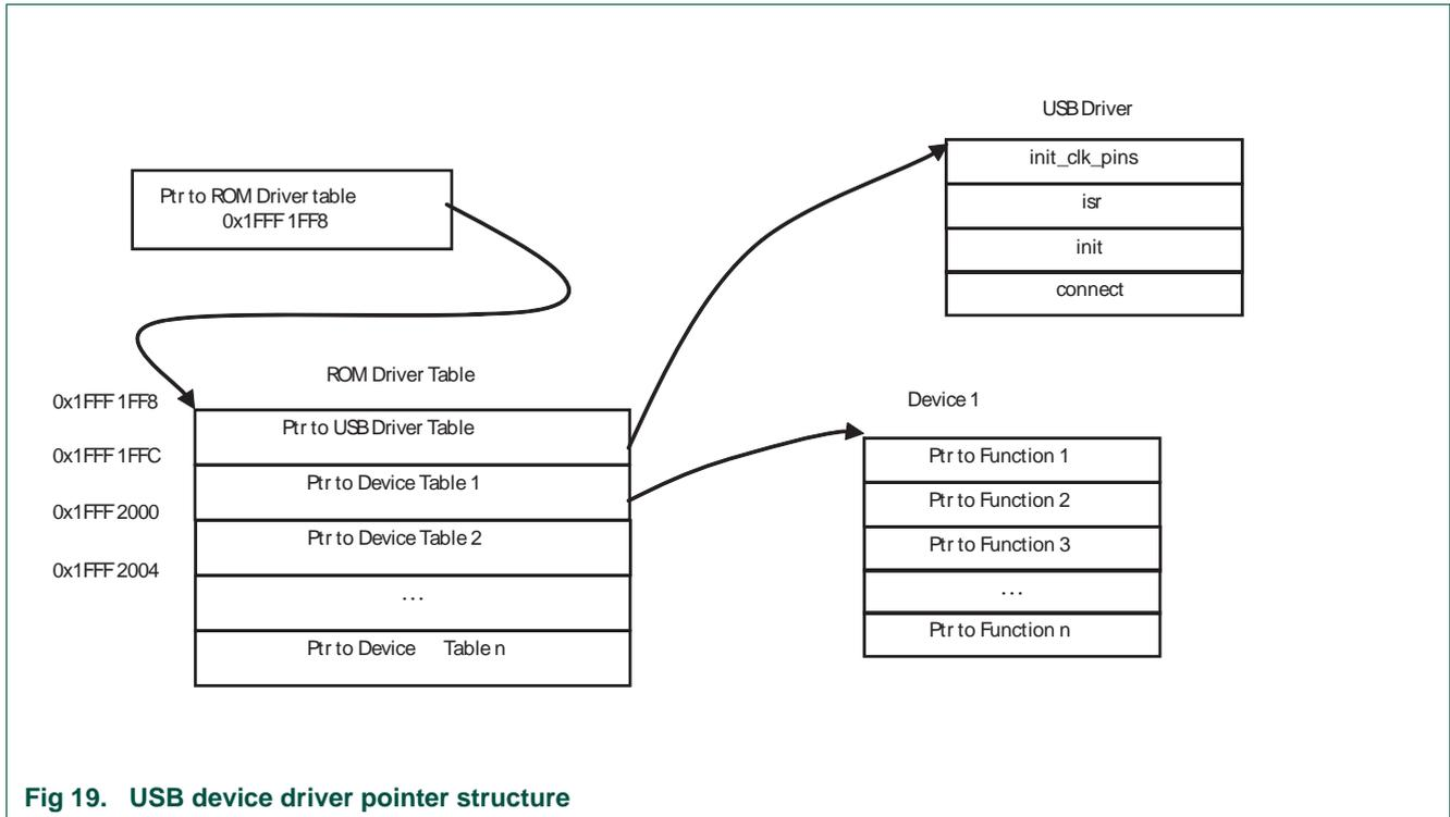
Fig 19. USB device driver pointer structure
