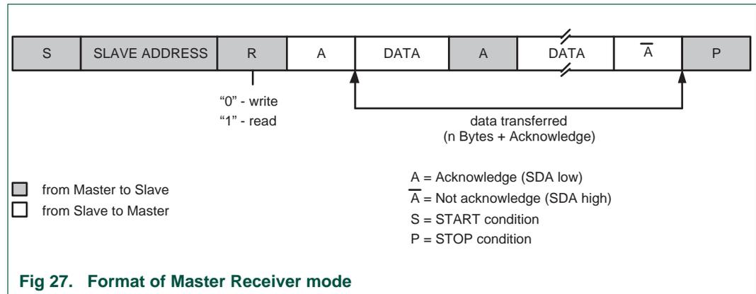
Fig 27. Format of Master Receiver mode
