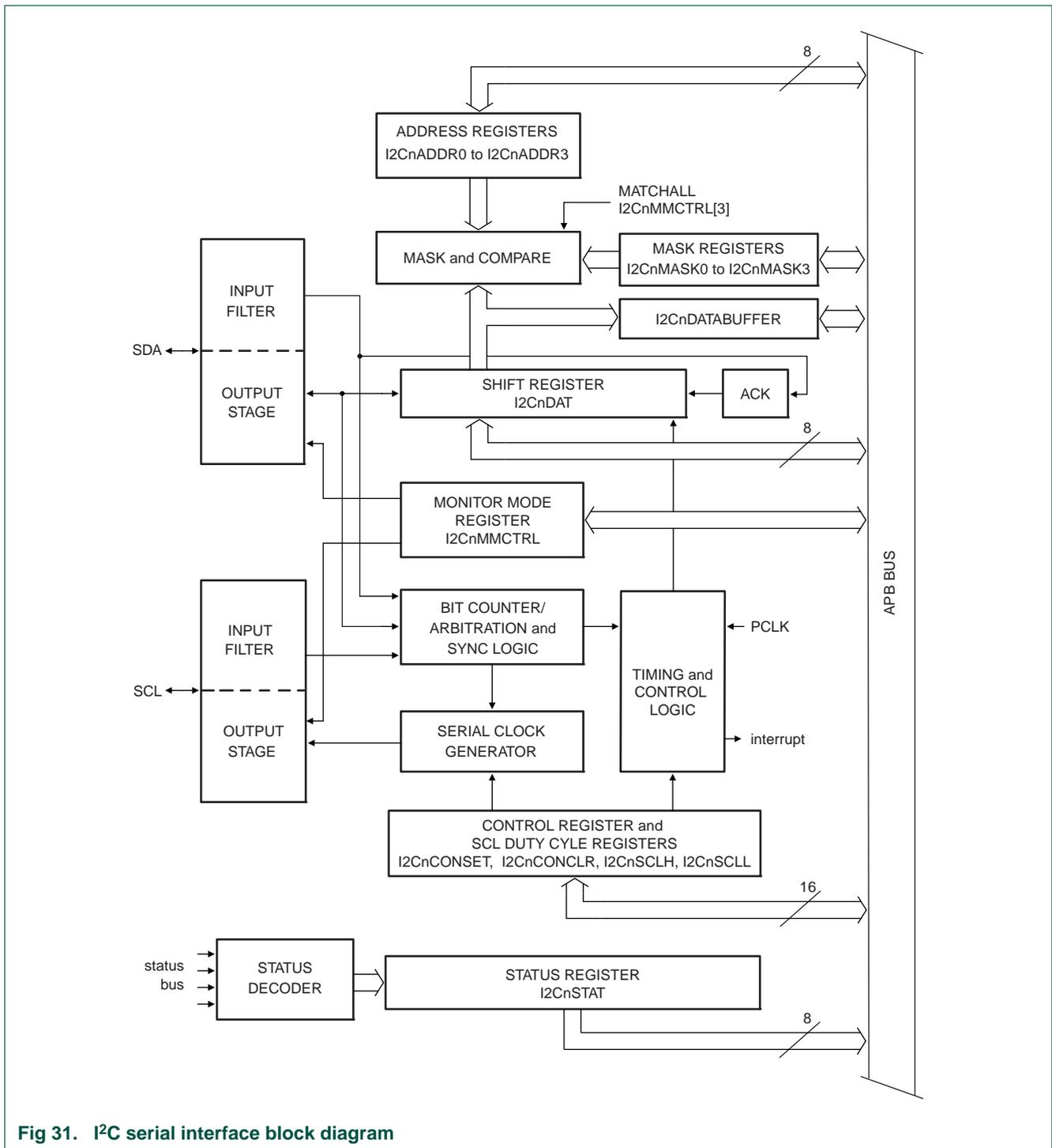
Fig 31. I2C serial interface block diagram
