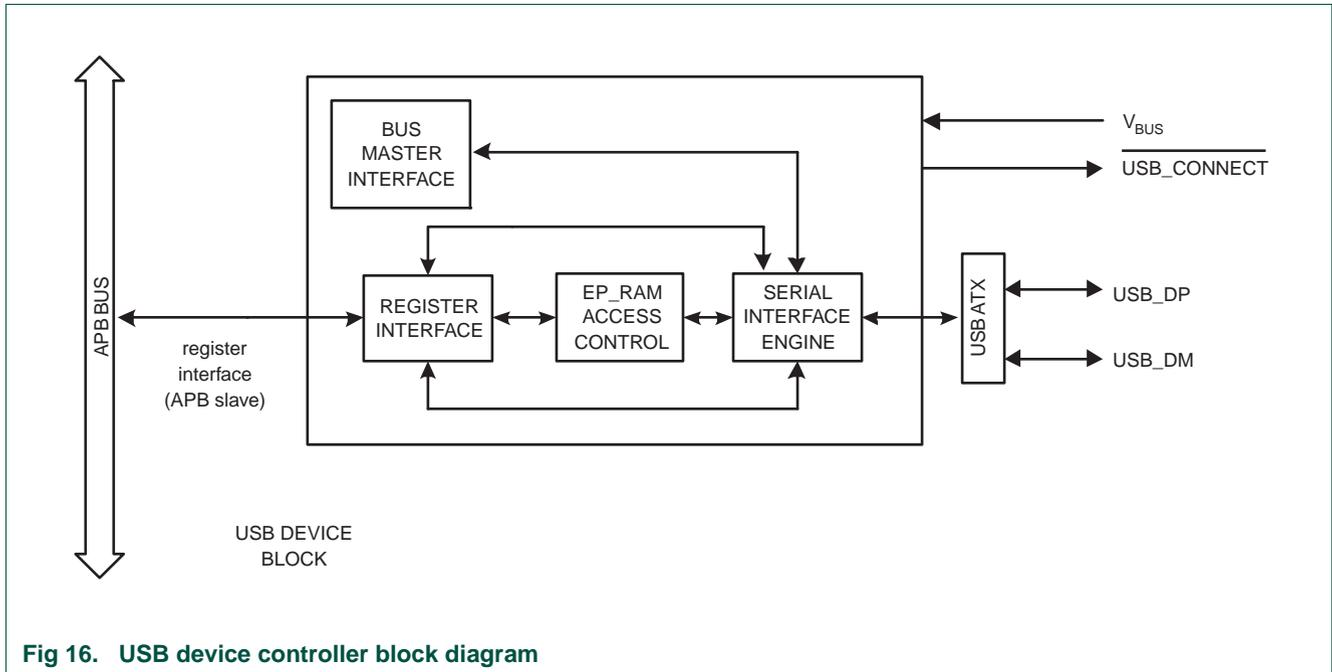
Fig 16. USB device controller block diagram
