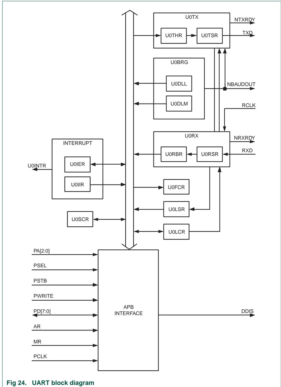
Fig 24. UART block diagram
