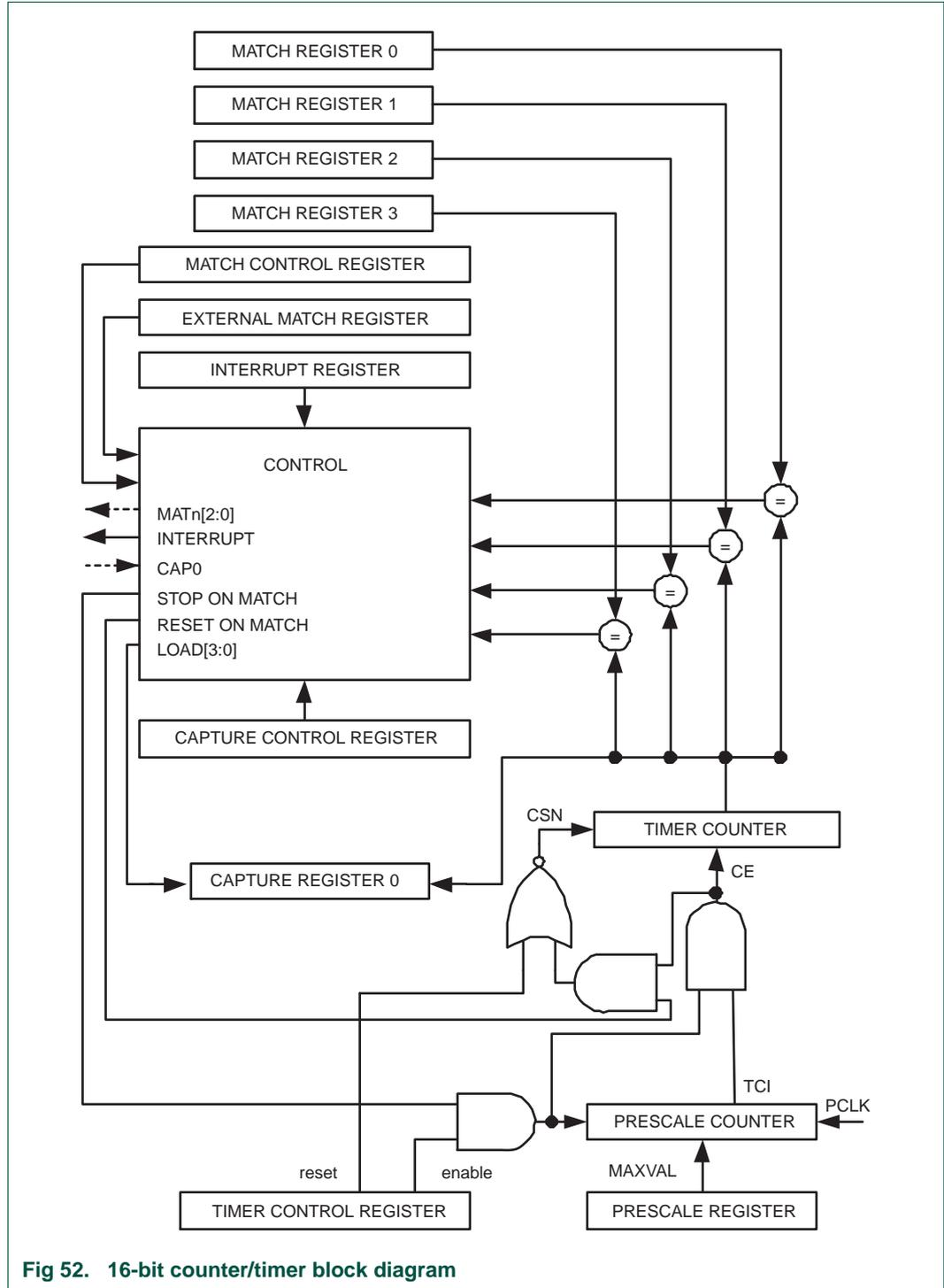
Fig 52. 16-bit counter/timer block diagram
