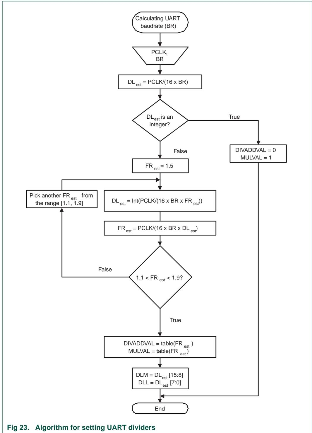
Fig 23. Algorithm for setting UART dividers
