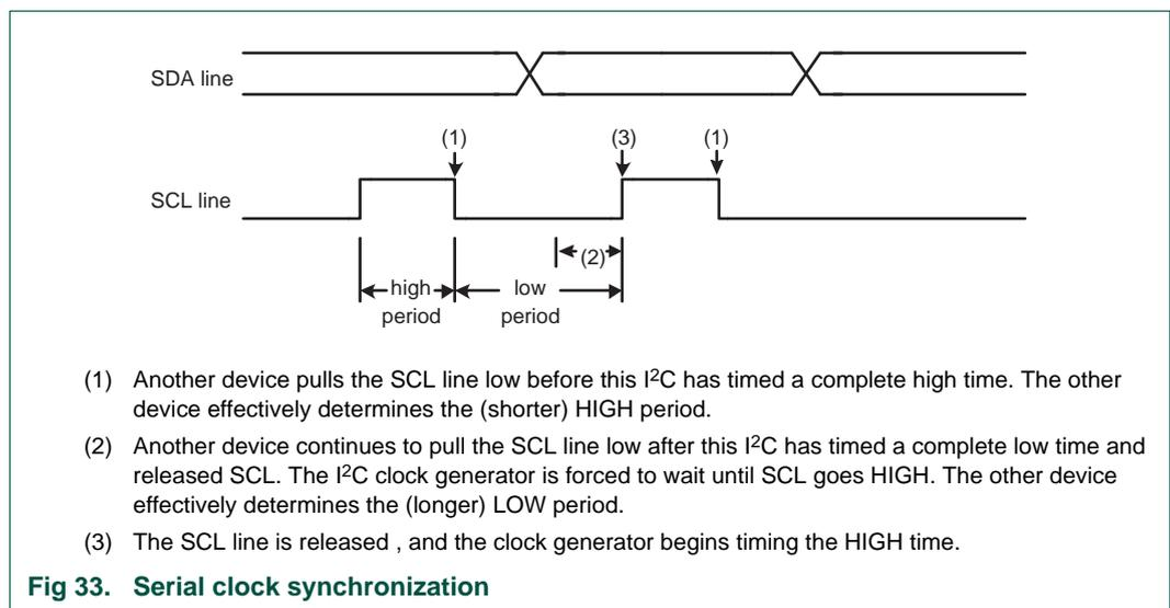
A slave may stretch the space duration to slow down the bus master. The space duration may also be stretched for handshaking purposes. This can be done after each bit or after a complete byte transfer. the I<sup>2</sup>C block will stretch the SCL space duration after a byte has been transmitted or received and the acknowledge bit has been transferred. The serial interrupt flag (SI) is set, and the stretching continues until the serial interrupt flag is cleared.
