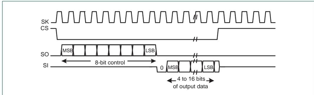
**Fig 46. Microwire frame format (single transfer)**
