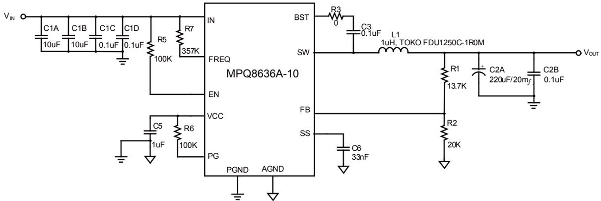
**Figure 10 — Typical Application Circuit with No External Ramp**
