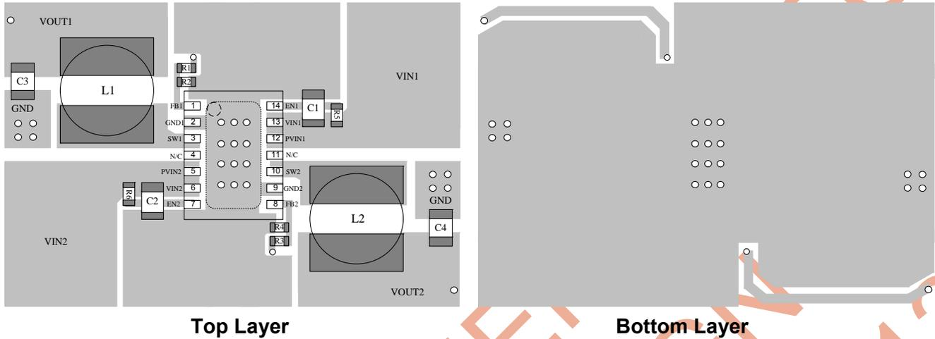
**Figure 3 -PCB Layout**
