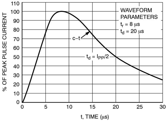
Figure 1. Pulse Waveform,  $8 \times 20 \mu\text{s}$
