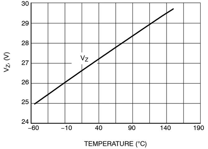
Figure 4. Typical  $V_Z$  @ 1.0 mA vs. Temperature
