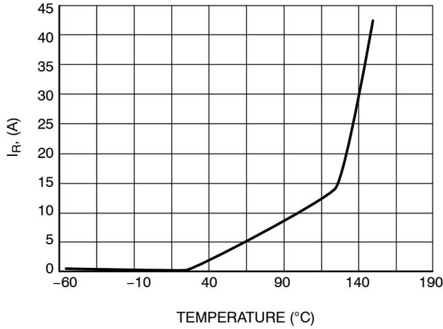
Figure 3. Typical Leakage vs. Temperature
