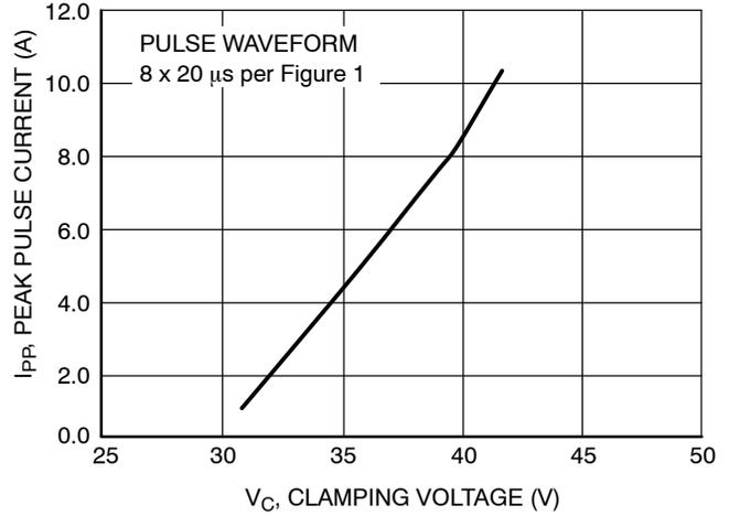
Figure 2. Clamping Voltage vs Peak Pulse Current
