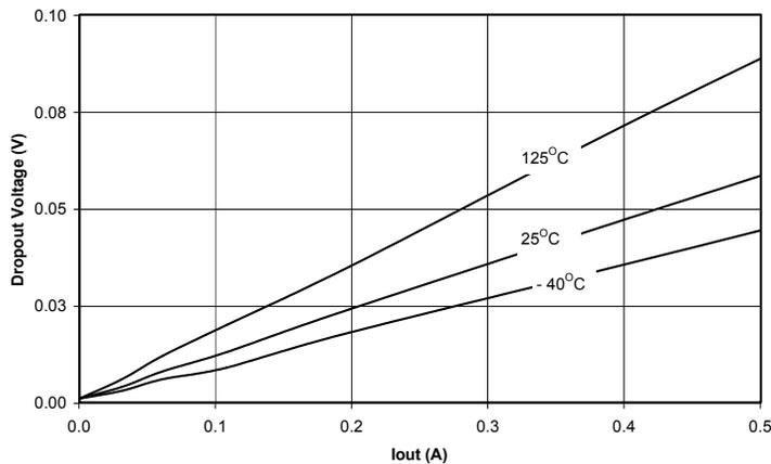
SC4213H Typical Dropout Voltage at Vout = 3.3V
