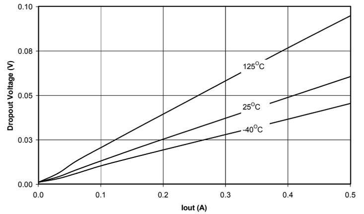
SC4213H Typical Dropout Voltage at Vout = 1.6V
