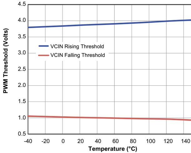
Fig 12. PWM Input Tristate Threshold vs. Temperature
