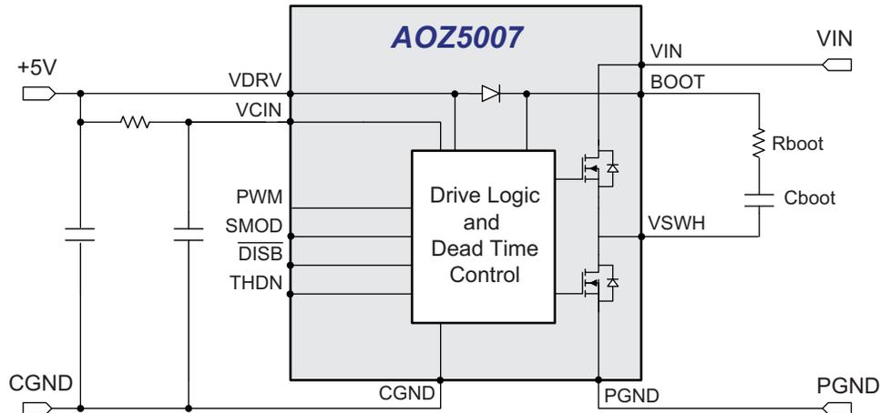
Figure 17. Applying VDRV and Generating BOOT Supply
