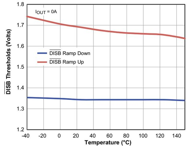
Fig 15. SMOD Input Threshold vs. Temperature
