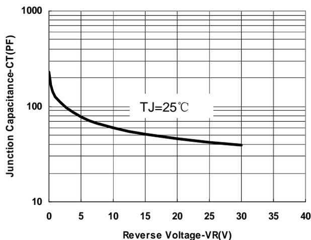
**Fig.1-Typical Junction Capacitance Vs.Reverse Voltage**
