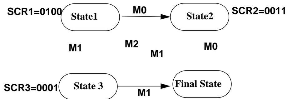
This scenario is currently not possible using 2 comparators only. S12SDBGV2 makes it possible with 2 comparators, State 3 allowing a M0 to return to state 2, whilst a M2 leads to final state as shown.
