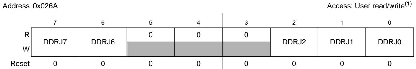
**Figure 2-49. Port J Data Direction Register (DDRJ)**
