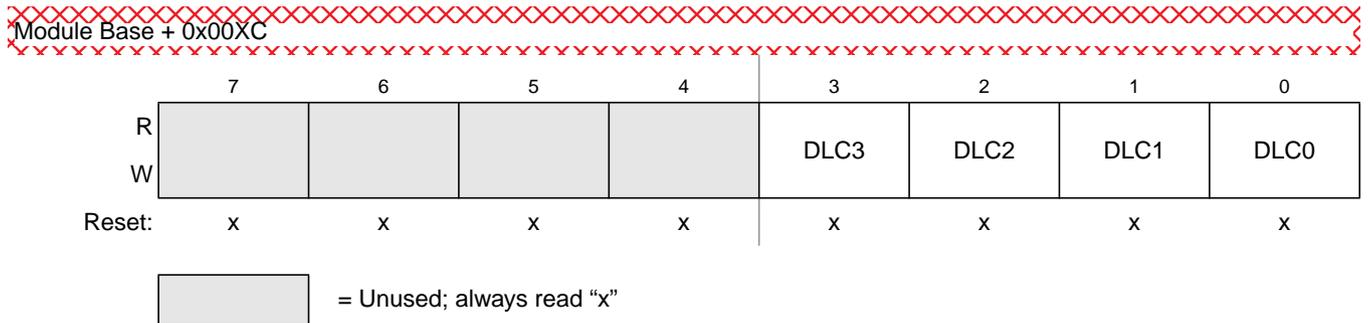
Figure 8-35. Data Length Register (DLR) — Extended Identifier Mapping
