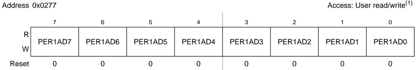
Figure 2-62. Port AD Pull Up Enable Register (PER1AD)
