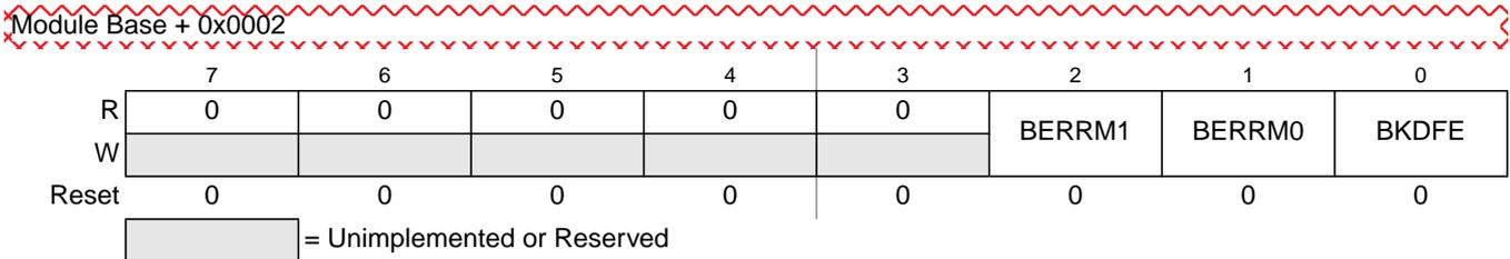
**Figure 11-8. SCI Alternative Control Register 2 (SCIACR2)**
