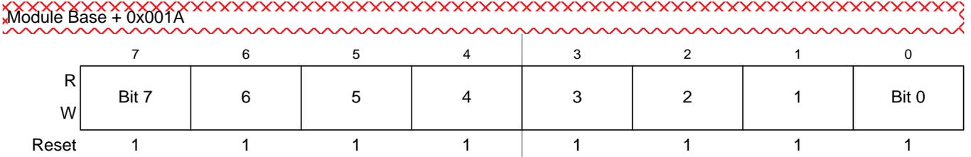
Figure 10-29. PWM Channel Duty Registers (PWMDTY2)
