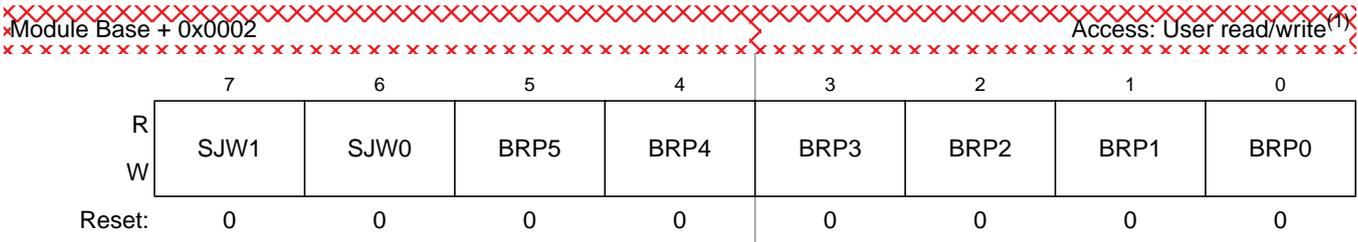
**Figure 8-6. MSCAN Bus Timing Register 0 (CANBTR0)**
