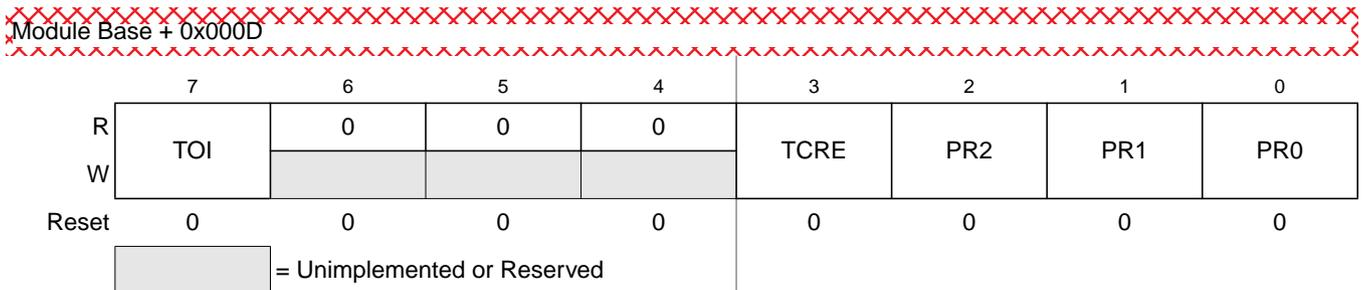
Figure 14-19. Timer System Control Register 2 (TSCR2)
