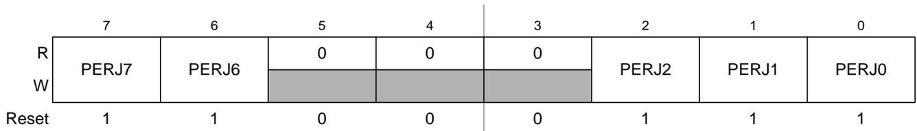
Figure 2-51. Port J Pull Device Enable Register (PERJ)
