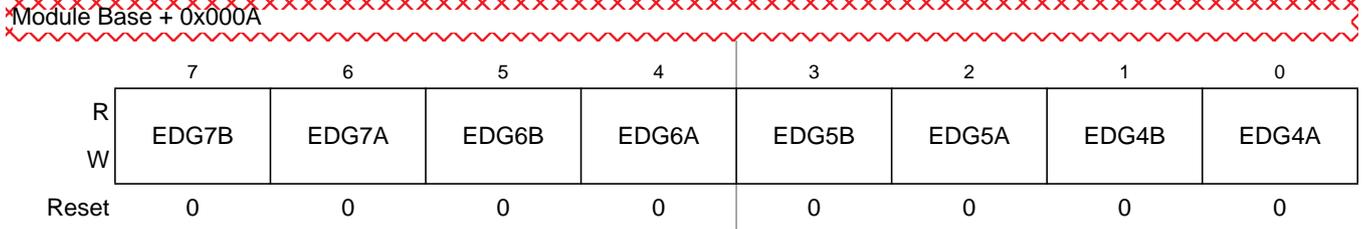
Figure 14-16. Timer Control Register 3 (TCTL3)
