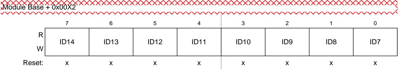
**Figure 8-28. Identifier Register 2 (IDR2) — Extended Identifier Mapping**
