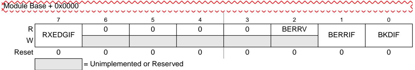
Figure 11-6. SCI Alternative Status Register 1 (SCIASR1)
