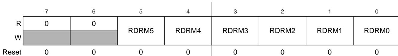
**Figure 2-33. Port M Reduced Drive Register (RDRM)**
