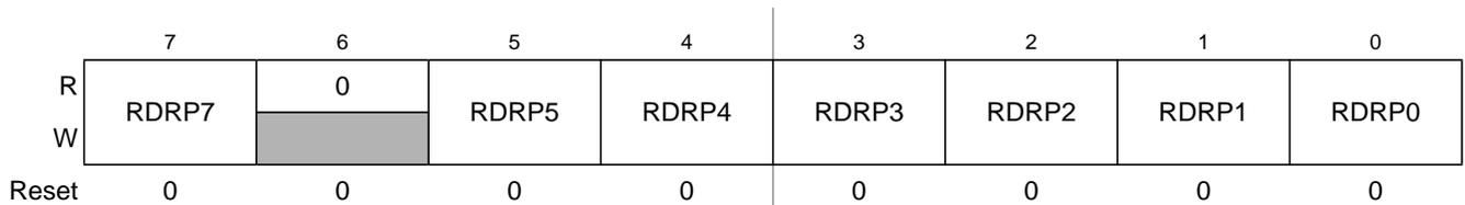
**Figure 2-41. Port P Reduced Drive Register (RDRP)**
