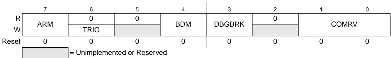
**Figure 6-3. Debug Control Register (DBGC1)**
