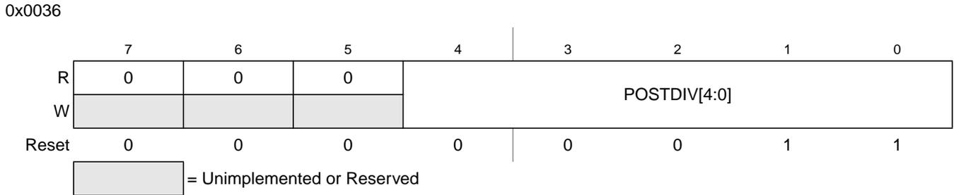
**Figure 7-6. S12CPMU Post Divider Register (CPMUPOSTDIV)**
