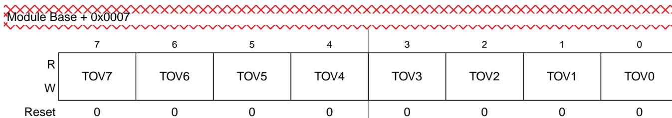
**Figure 14-13. Timer Toggle On Overflow Register 1 (TTOV)**
