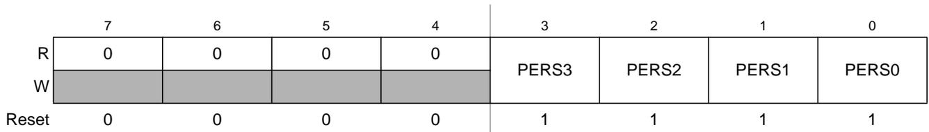
**Figure 2-26. Port S Pull Device Enable Register (PERS)**
