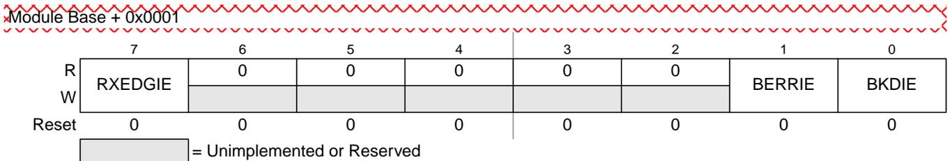
Figure 11-7. SCI Alternative Control Register 1 (SCIACR1)
