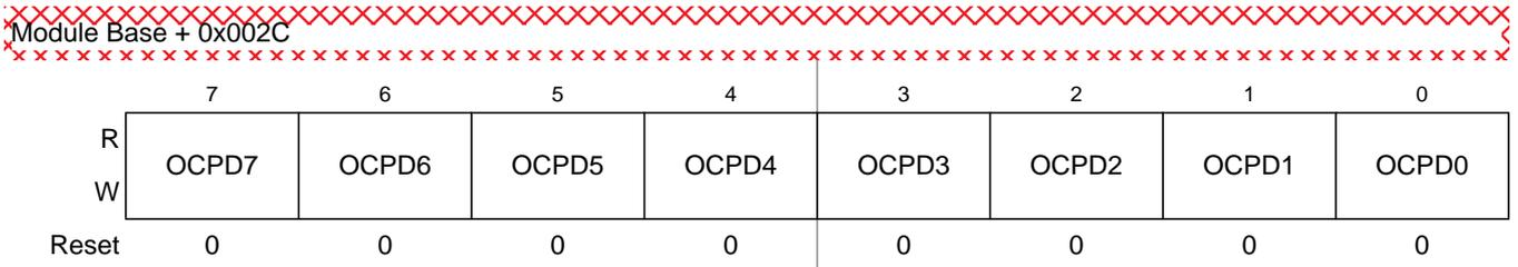
Figure 14-28. Ouput Compare Pin Disconnect Register (OCPD)
