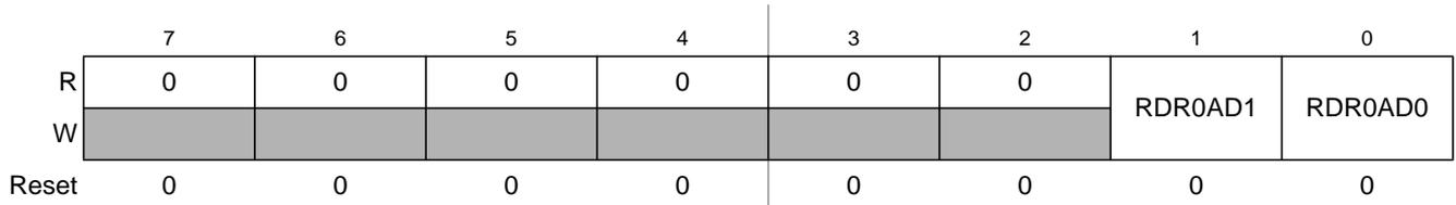
Figure 2-59. Port AD Reduced Drive Register (RDR0AD)
