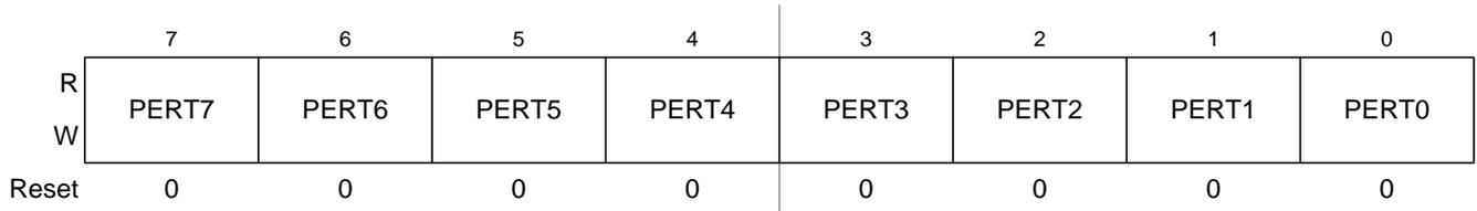
Figure 2-18. Port T Pull Device Enable Register (PERT)
