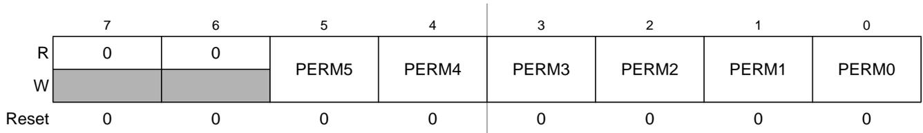
**Figure 2-34. Port M Pull Device Enable Register (PERM)**
