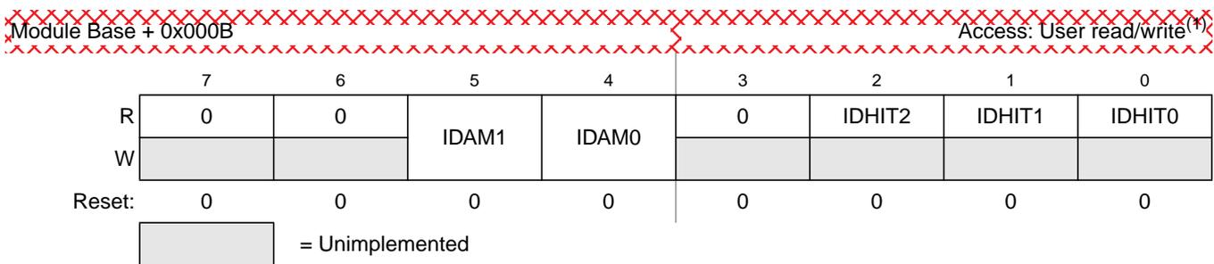
**Figure 8-15. MSCAN Identifier Acceptance Control Register (CANIDAC)**
