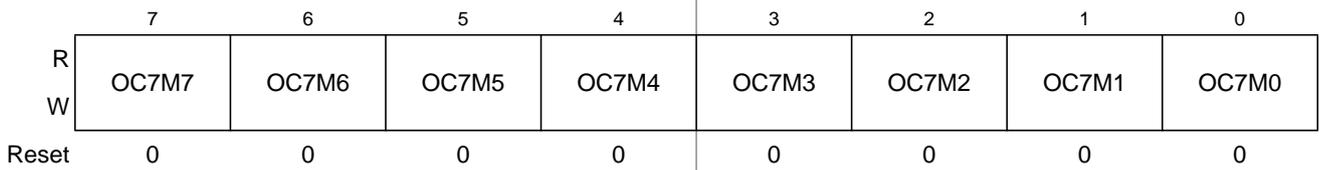
**Figure 14-8. Output Compare 7 Mask Register (OC7M)**
