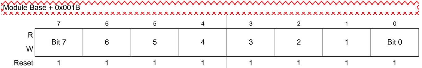
Figure 10-30. PWM Channel Duty Registers (PWMDTY3)
