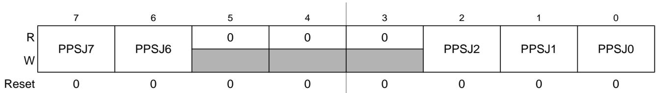
**Figure 2-52. Port J Polarity Select Register (PPSJ)**
