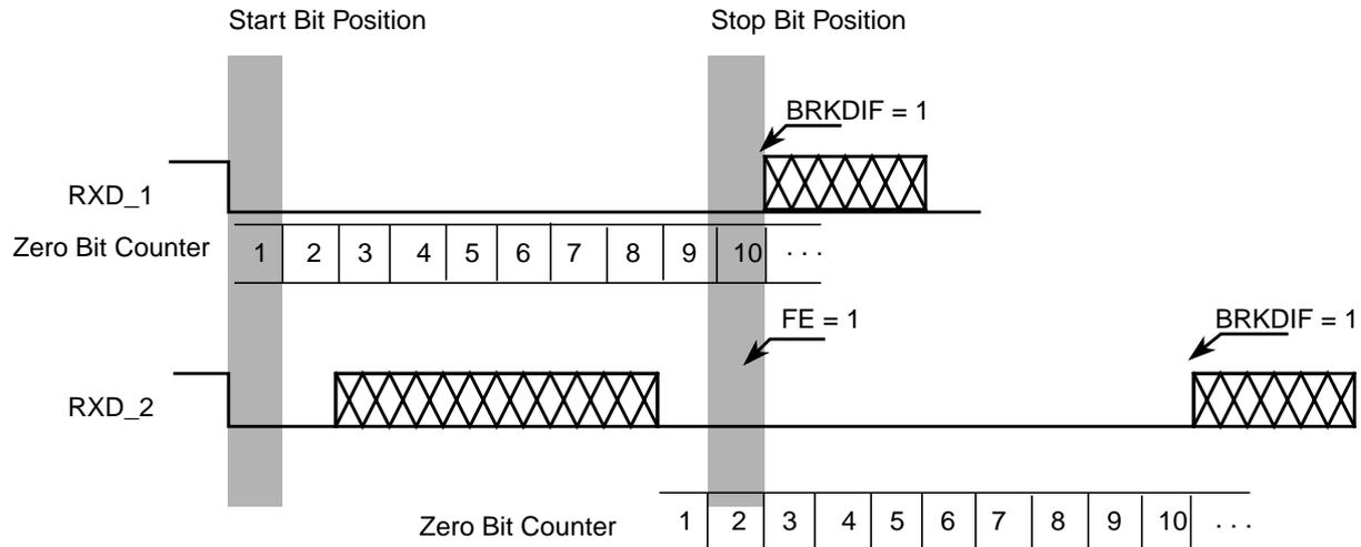
Figure 11-17. Break Detection if BRKDFE = 1 (M = 0)
