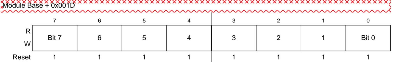
**Figure 10-32. PWM Channel Duty Registers (PWMDTY5)**
