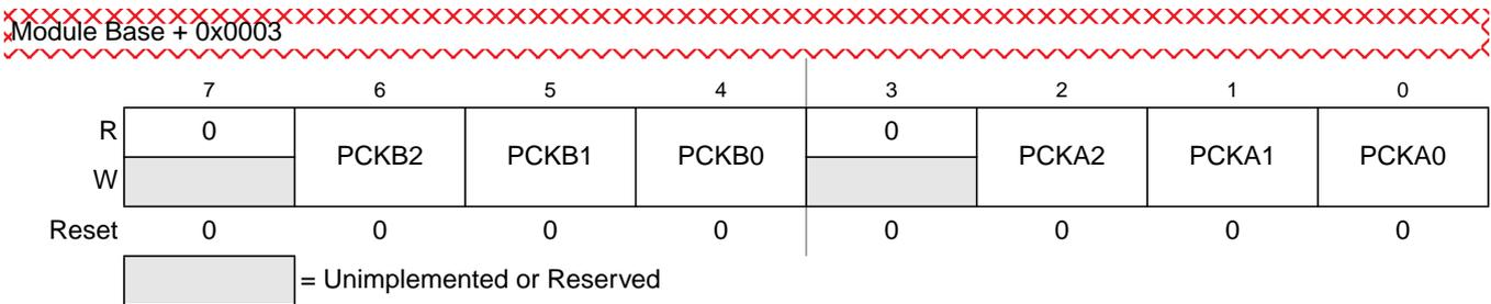
**Figure 10-6. PWM Prescaler Clock Select Register (PWMPRCLK)**
