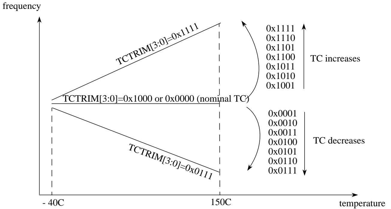
**Figure 7-27. Influence of TCTRIM[3:0] on the Temperature Coefficient**
