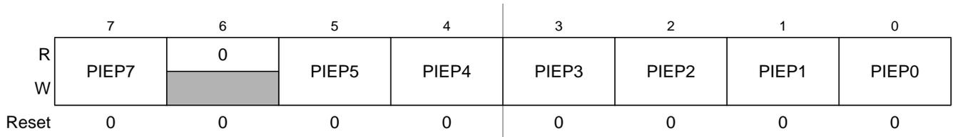
**Figure 2-44. Port P Interrupt Enable Register (PIEP)**
