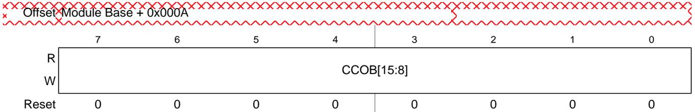
Figure 13-16. Flash Common Command Object High Register (FCCOBHI)
