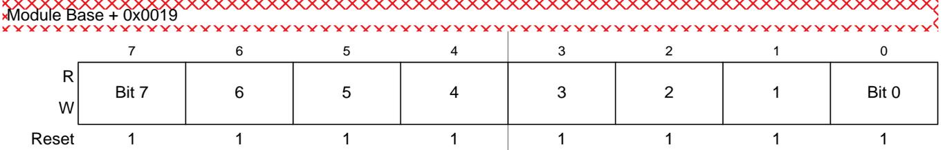
Figure 10-28. PWM Channel Duty Registers (PWMDTY1)
