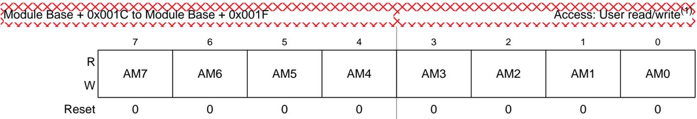
**Figure 8-23. MSCAN Identifier Mask Registers (Second Bank) — CANIDMR4–CANIDMR7**
