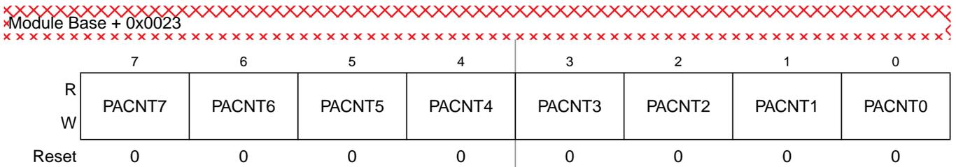
**Figure 14-27. Pulse Accumulator Count Register Low (PACNTL)**
