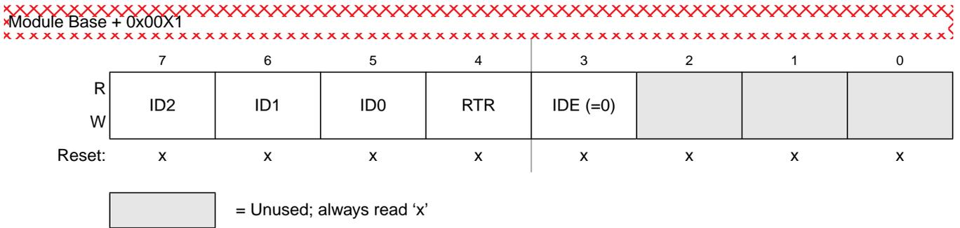
Figure 8-31. Identifier Register 1 — Standard Mapping
