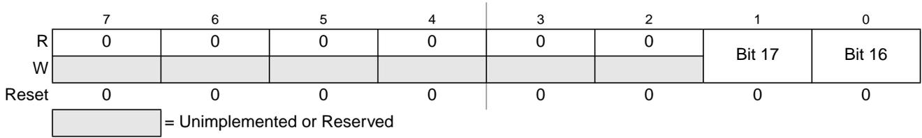
**Figure 6-16. Debug Comparator Address High Register (DBGXAH)**
