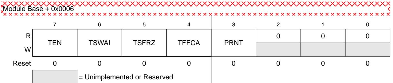
Figure 14-12. Timer System Control Register 1 (TSCR1)
