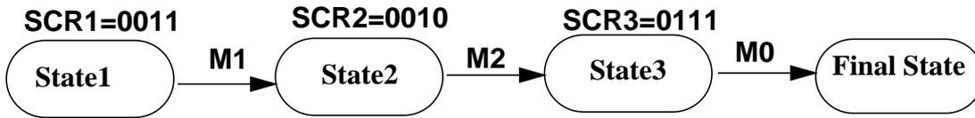
Scenario 1 is possible with S12SDBGV1 SCR encoding
