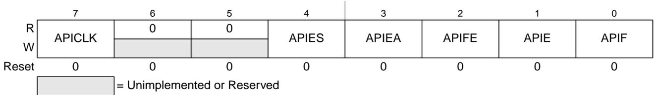
**Figure 7-18. Autonomous Periodical Interrupt Control Register (CPMUAPICTL)**
