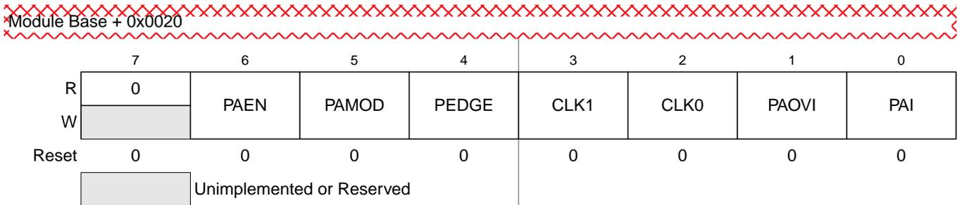
**Figure 14-24. 16-Bit Pulse Accumulator Control Register (PACTL)**
