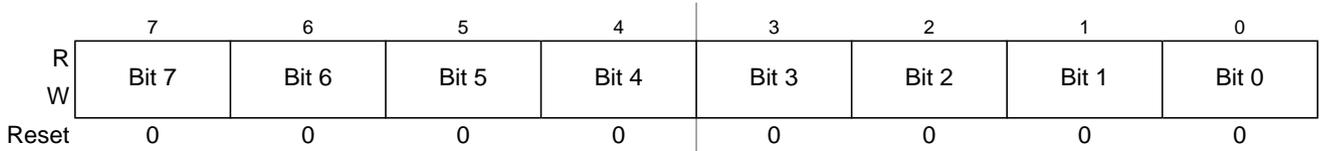
**Figure 6-18. Debug Comparator Address Low Register (DBGXAL)**
