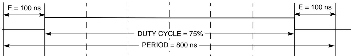
Figure 10-39. PWM Center Aligned Output Example Waveform
