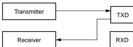
Figure 11-30. Single-Wire Operation (LOOPS = 1, RSRC = 1)
