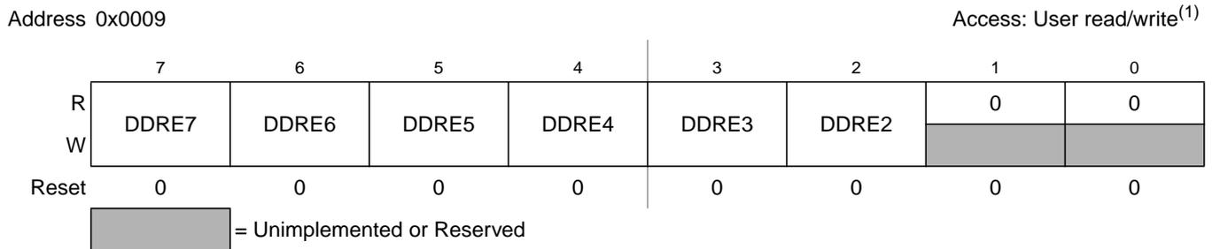
**Figure 2-7. Port E Data Direction Register (DDRE)**
