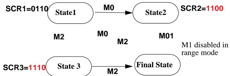
The advantage of using only 2 channels is that now range comparisons can be included (channel0)
