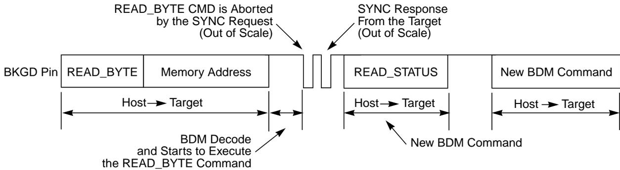
**Figure 5-12. ACK Abort Procedure at the Command Level**
