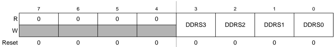
**Figure 2-24. Port S Data Direction Register (DDRS)**
