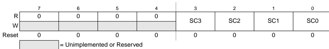
**Figure 6-9. Debug State Control Register 1 (DBGSCR1)**
