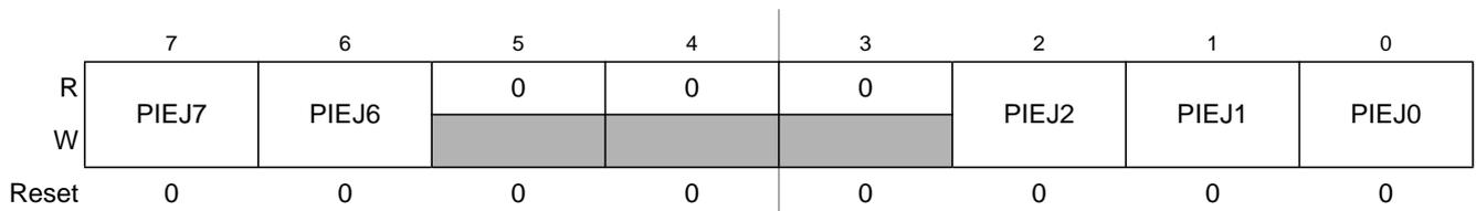
**Figure 2-53. Port J Interrupt Enable Register (PIEJ)**
