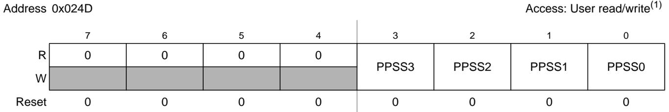
Figure 2-27. Port S Polarity Select Register (PPSS)
