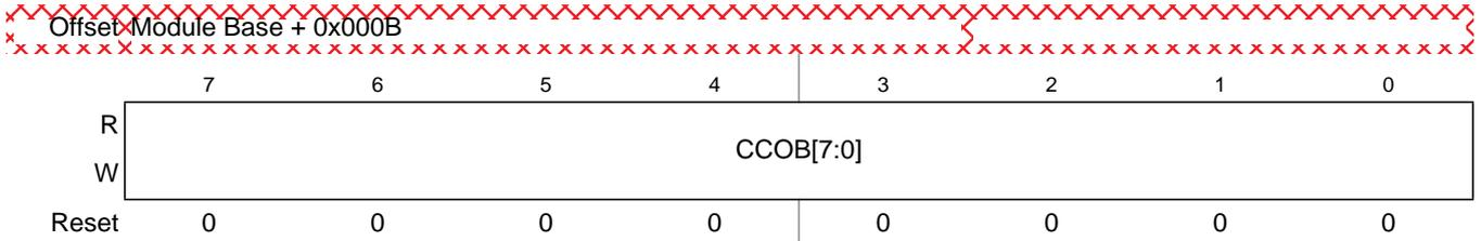
Figure 13-17. Flash Common Command Object Low Register (FCCOBLO)
