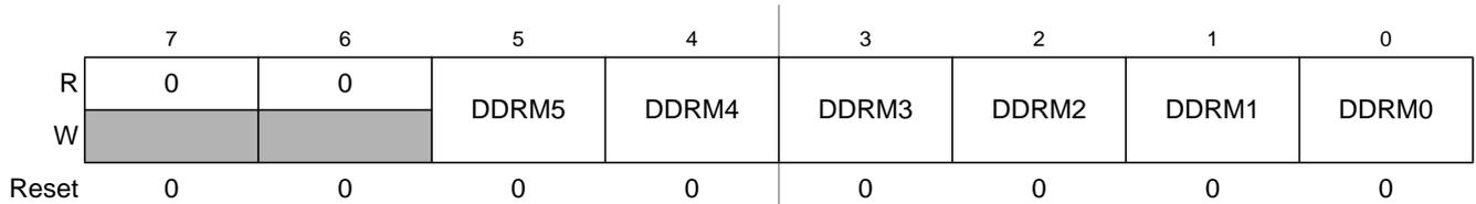
**Figure 2-32. Port M Data Direction Register (DDRM)**
