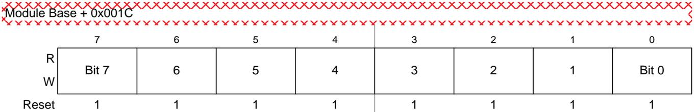
Figure 10-31. PWM Channel Duty Registers (PWMDTY4)
