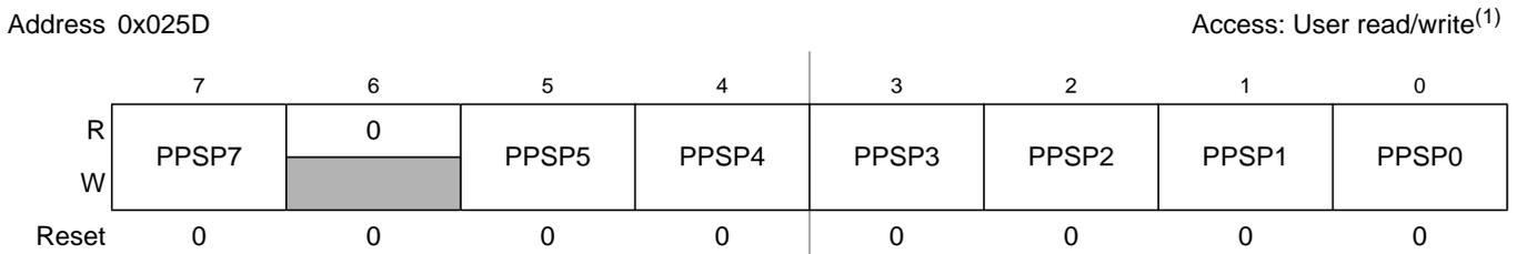
Figure 2-43. Port P Polarity Select Register (PPSP)
