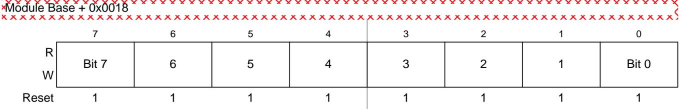
Figure 10-27. PWM Channel Duty Registers (PWMDTY0)
