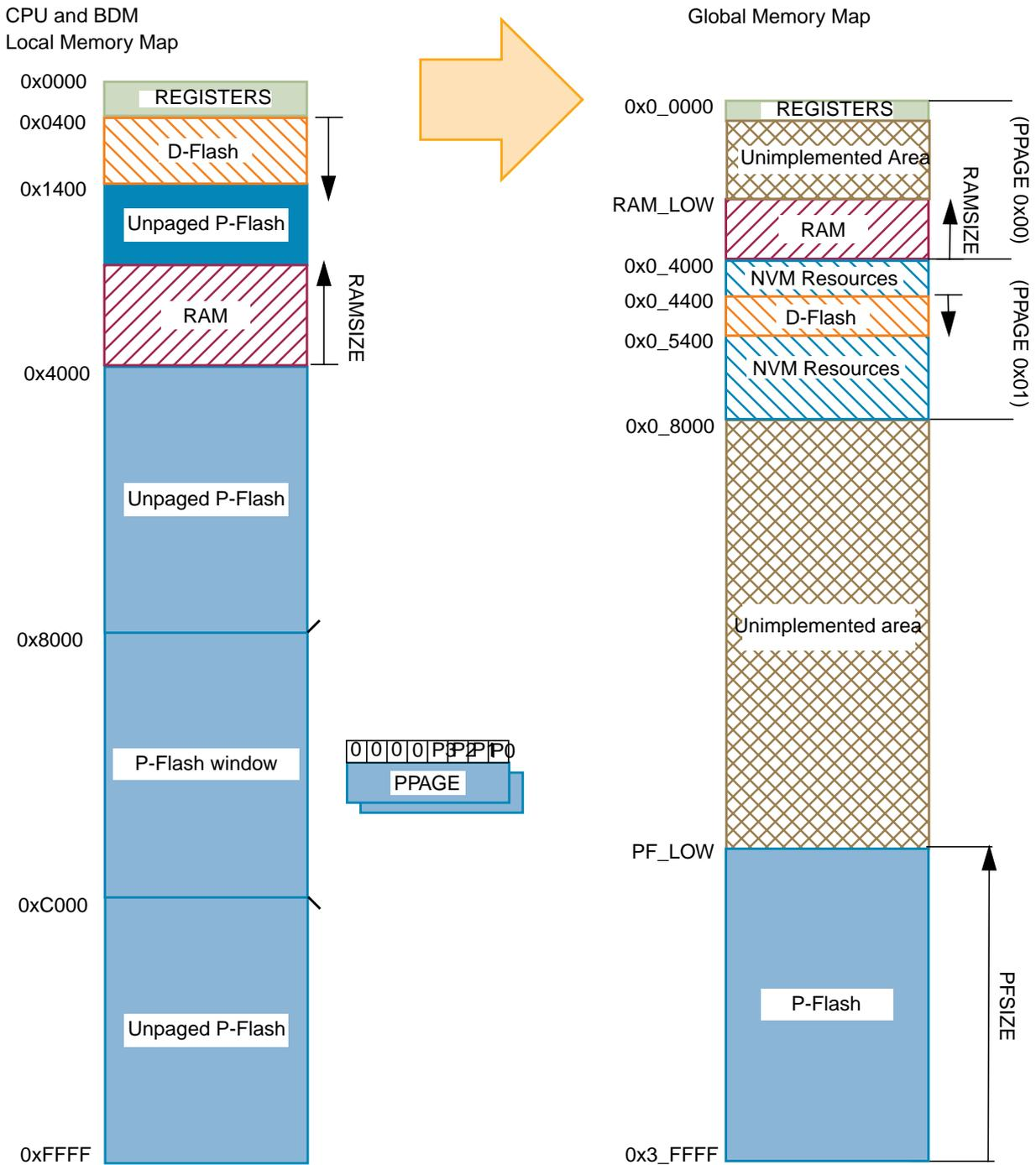
Figure 3-11. Implemented Global Address Mapping
