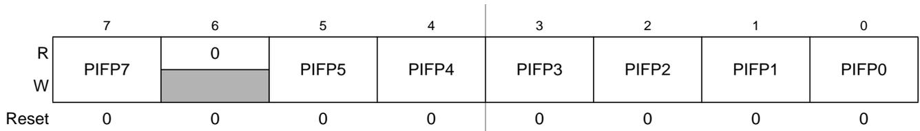
**Figure 2-45. Port P Interrupt Flag Register (PIFP)**
