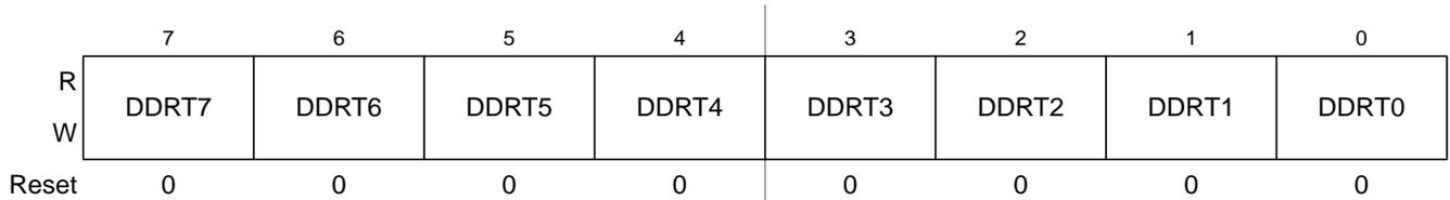
**Figure 2-16. Port T Data Direction Register (DDRT)**
