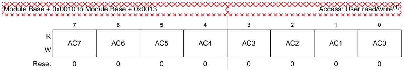
**Figure 8-20. MSCAN Identifier Acceptance Registers (First Bank) — CANIDAR0–CANIDAR3**
