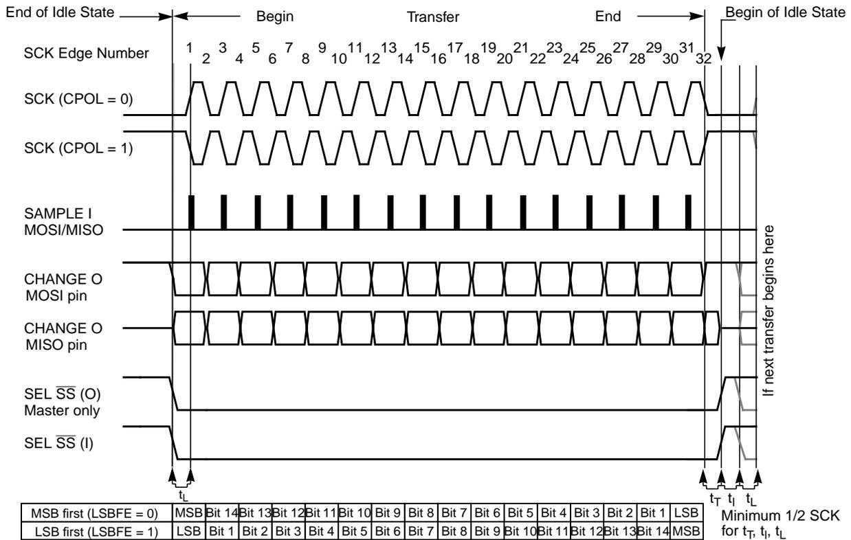
**Figure 12-13. SPI Clock Format 0 (CPHA = 0), with 16-Bit Transfer Width selected (XFRW = 1)**
