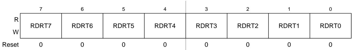
Figure 2-17. Port T Reduced Drive Register (RDRT)
