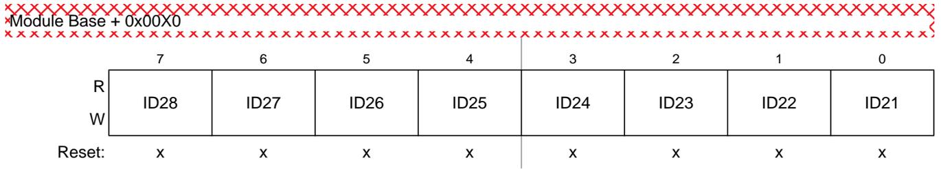
Figure 8-26. Identifier Register 0 (IDR0) — Extended Identifier Mapping
