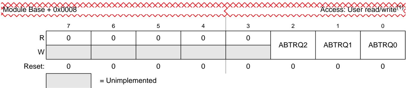
**Figure 8-12. MSCAN Transmitter Message Abort Request Register (CANTARQ)**
