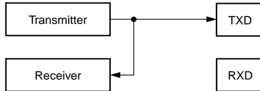
Figure 11-31. Loop Operation (LOOPS = 1, RSRC = 0)
