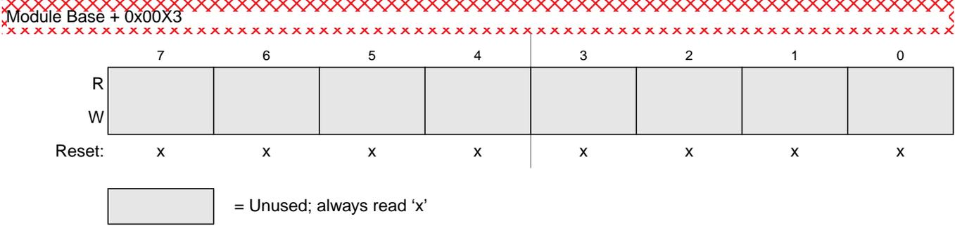
**Figure 8-33. Identifier Register 3 — Standard Mapping**
