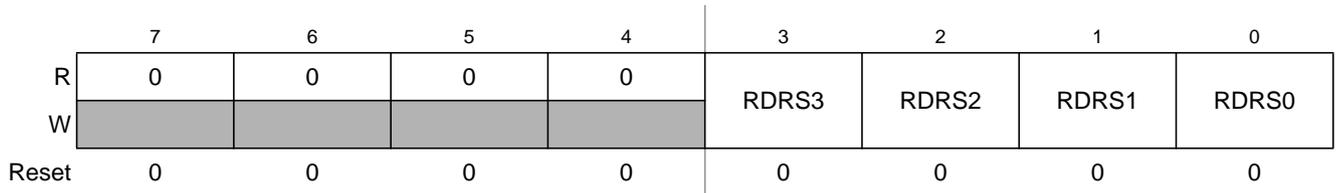
**Figure 2-25. Port S Reduced Drive Register (RDRS)**
