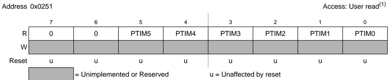
**Figure 2-31. Port M Input Register (PTIM)**
