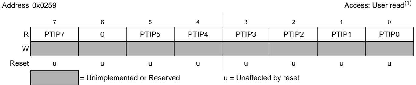
**Figure 2-39. Port P Input Register (PTIP)**
