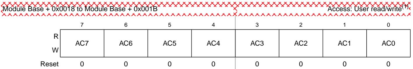
**Figure 8-21. MSCAN Identifier Acceptance Registers (Second Bank) — CANIDAR4–CANIDAR7**
