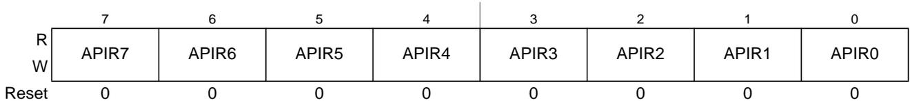
**Figure 7-22. Autonomous Periodical Interrupt Rate Low Register (CPMUAPIRL)**
