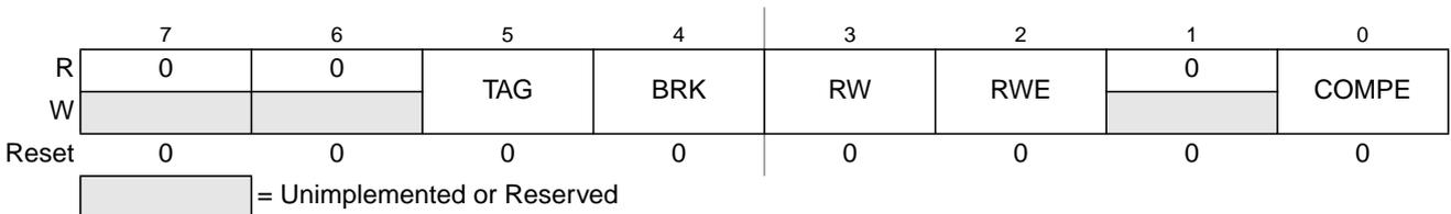
**Figure 6-15. Debug Comparator Control Register DBGCCTL (Comparator C)**
