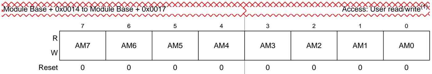
**Figure 8-22. MSCAN Identifier Mask Registers (First Bank) — CANIDMR0–CANIDMR3**
