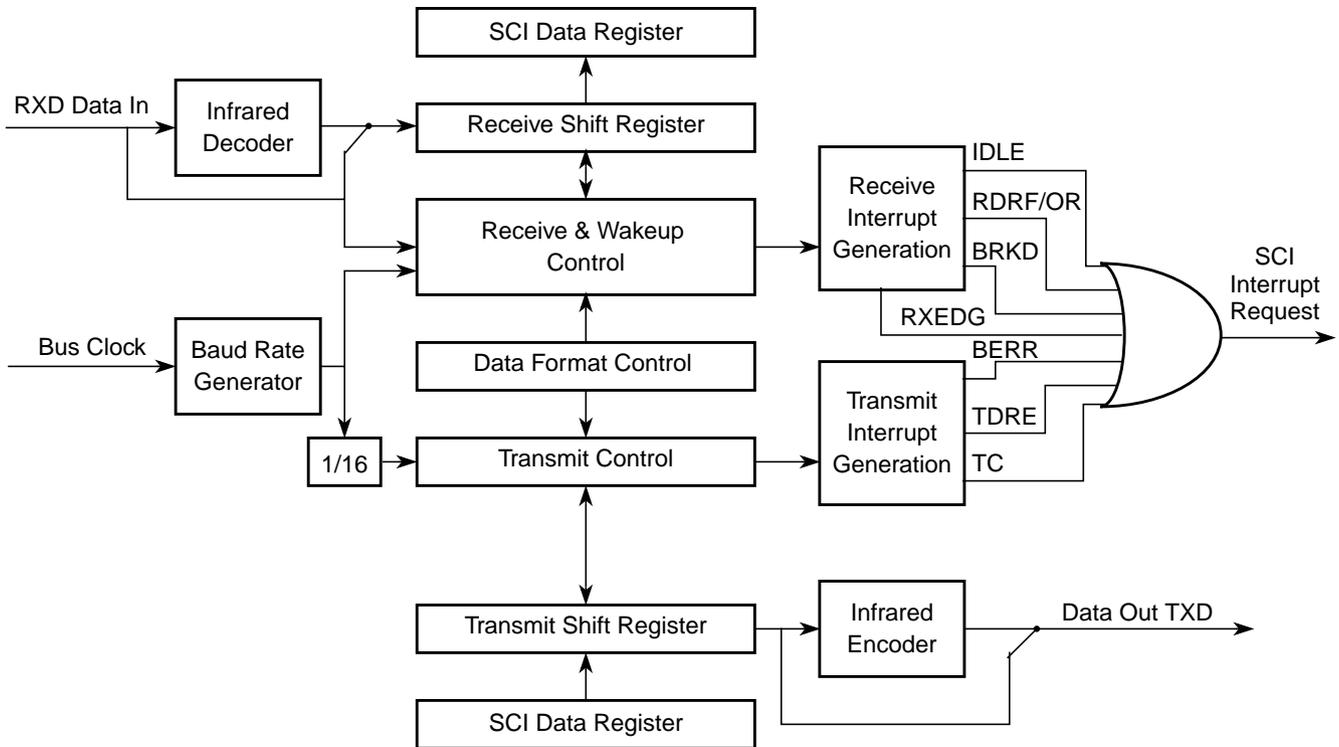
Figure 11-1. SCI Block Diagram
