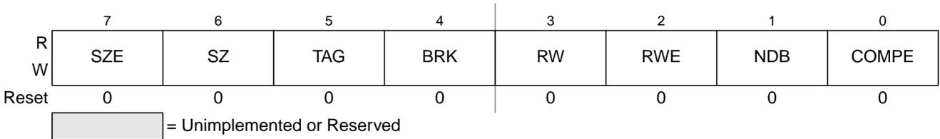
**Figure 6-13. Debug Comparator Control Register DBGACTL (Comparator A)**
