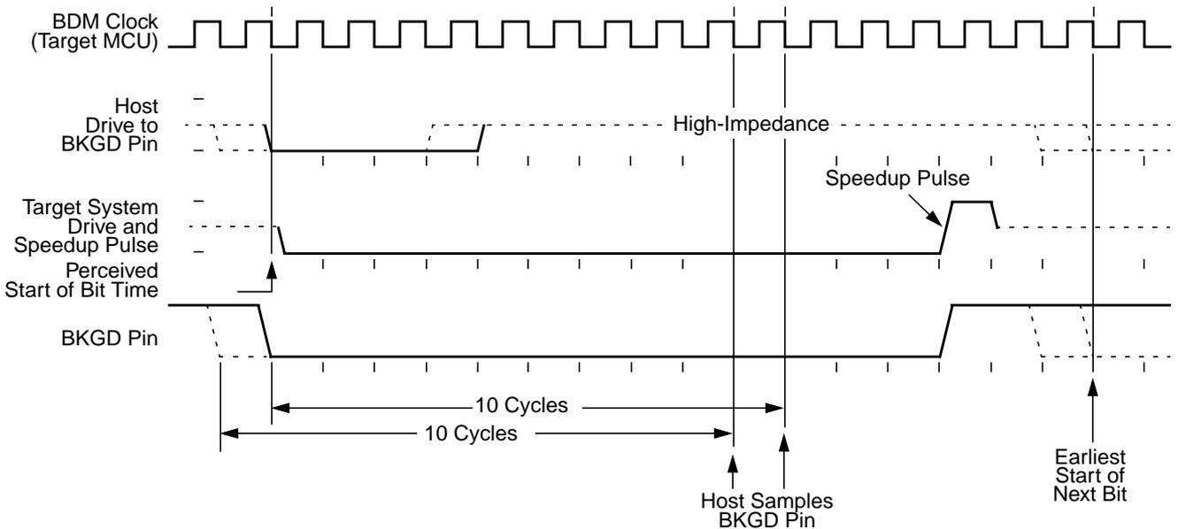
**Figure 5-9. BDM Target-to-Host Serial Bit Timing (Logic 0)**
