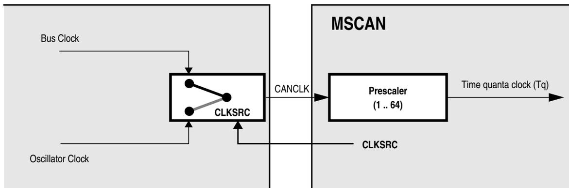
Figure 8-43. MSCAN Clocking Scheme
