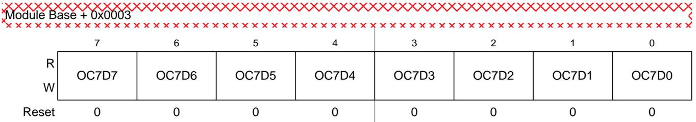
Figure 14-9. Output Compare 7 Data Register (OC7D)
