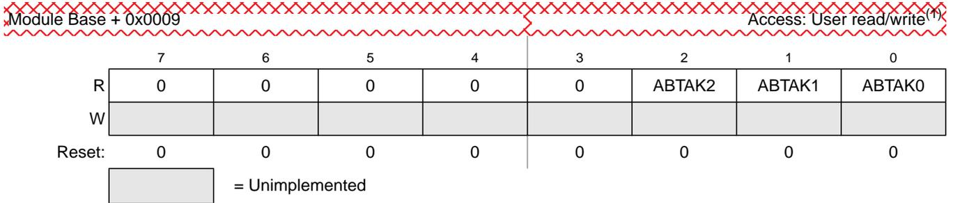
**Figure 8-13. MSCAN Transmitter Message Abort Acknowledge Register (CANTAACK)**
