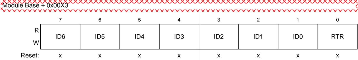
**Figure 8-29. Identifier Register 3 (IDR3) — Extended Identifier Mapping**
