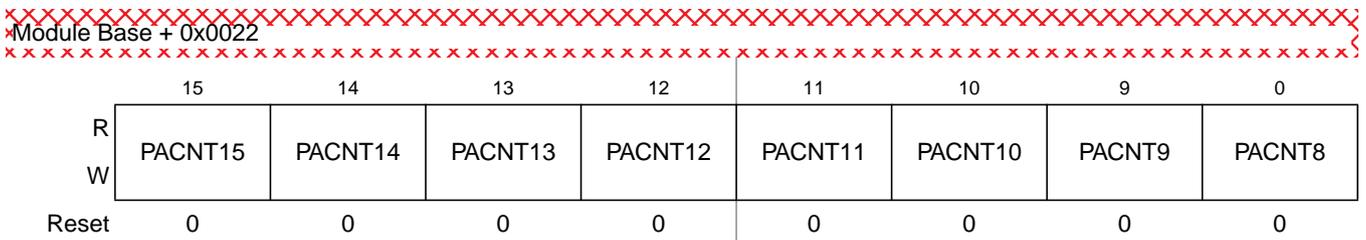
**Figure 14-26. Pulse Accumulator Count Register High (PACNTH)**
