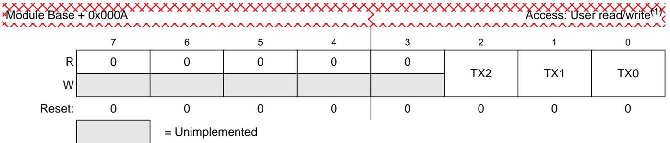
**Figure 8-14. MSCAN Transmit Buffer Selection Register (CANTBSEL)**
