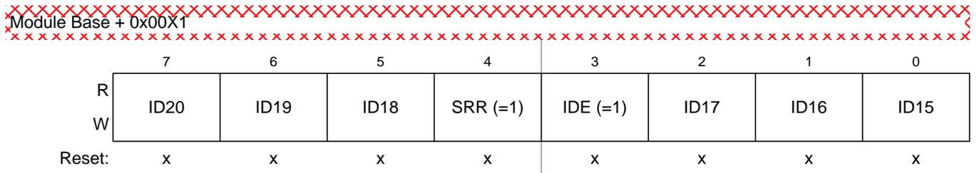
Figure 8-27. Identifier Register 1 (IDR1) — Extended Identifier Mapping
