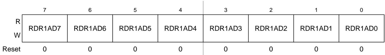
**Figure 2-60. Port AD Reduced Drive Register (RDR1AD)**
