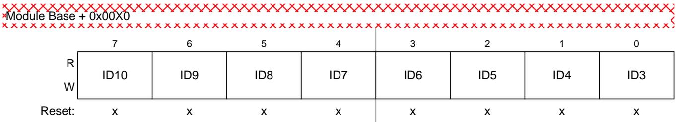
Figure 8-30. Identifier Register 0 — Standard Mapping
