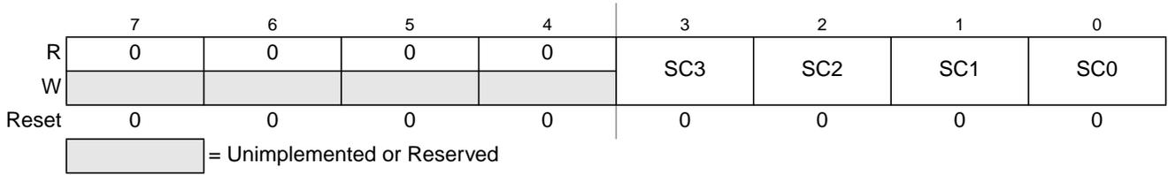
**Figure 6-11. Debug State Control Register 3 (DBGSCR3)**
