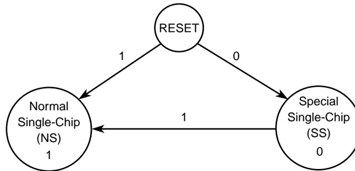
**Figure 3-4. Mode Transition Diagram when MCU is Unsecured**
