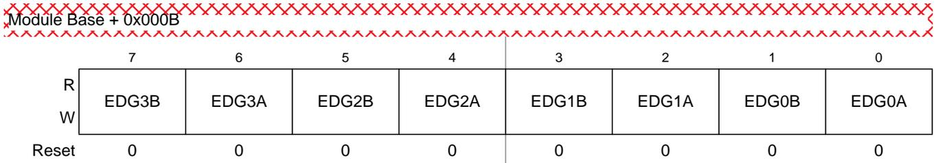
Figure 14-17. Timer Control Register 4 (TCTL4)
