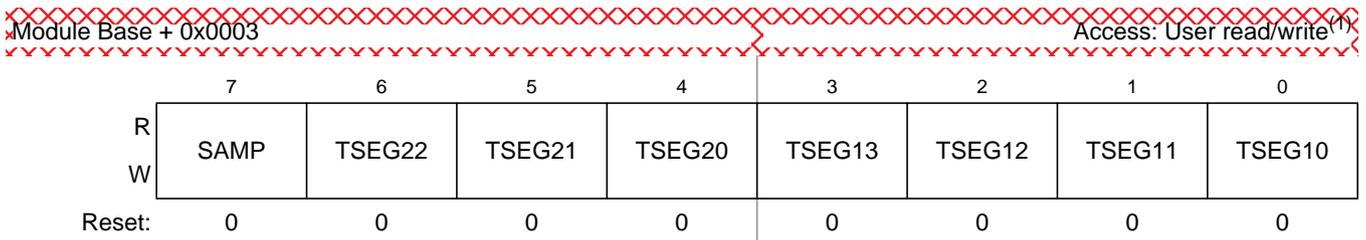
**Figure 8-7. MSCAN Bus Timing Register 1 (CANBTR1)**
