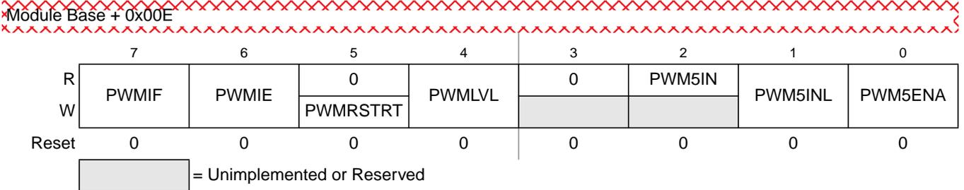
**Figure 10-33. PWM Shutdown Register (PWMSDN)**
