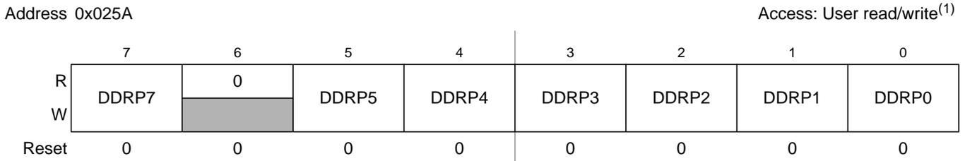
**Figure 2-40. Port P Data Direction Register (DDRP)**
