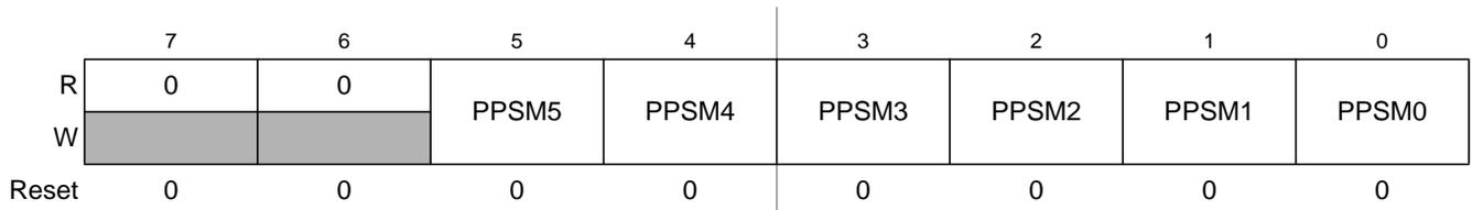
**Figure 2-35. Port M Polarity Select Register (PPSM)**
