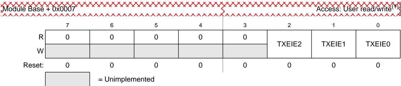
**Figure 8-11. MSCAN Transmitter Interrupt Enable Register (CANTIER)**
