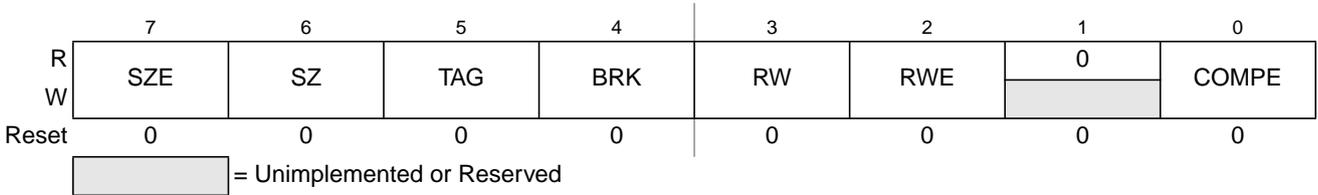
**Figure 6-14. Debug Comparator Control Register DBGBCTL (Comparator B)**
