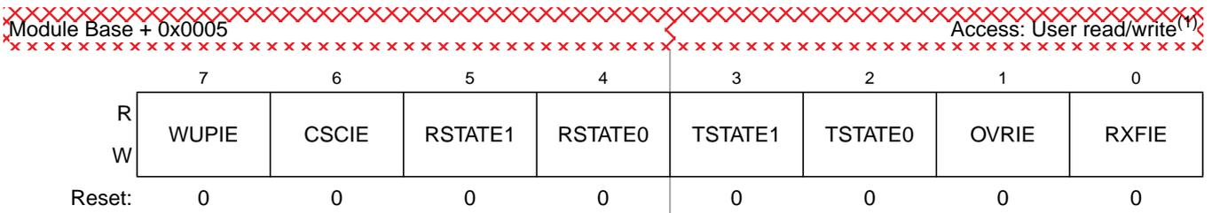
**Figure 8-9. MSCAN Receiver Interrupt Enable Register (CANRIER)**
