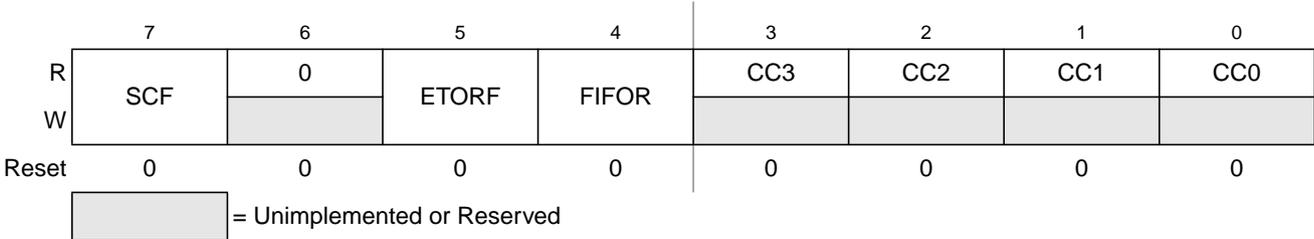
**Figure 9-9. ATD Status Register 0 (ATDSTAT0)**
