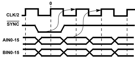
FIGURE 22. DATA SYNCHRONIZATION WITH PROCESSING LEGS ( $\overline{\text{INT/EXT}} = 1$ )
