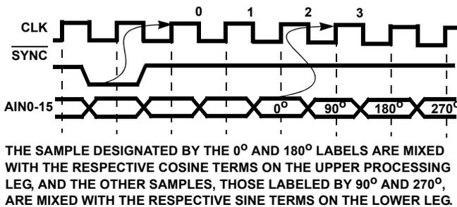
THE SAMPLE DESIGNATED BY THE 0° AND 180° LABELS ARE MIXED WITH THE RESPECTIVE COSINE TERMS ON THE UPPER PROCESSING LEG, AND THE OTHER SAMPLES, THOSE LABELED BY 90° AND 270°, ARE MIXED WITH THE RESPECTIVE SINE TERMS ON THE LOWER LEG.
