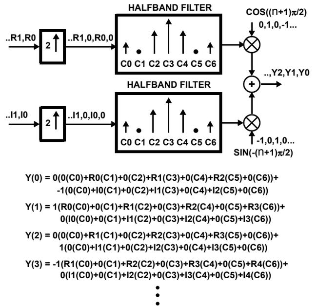
FIGURE 19. QUADRATURE TO REAL CONVERTER USING TRANSVERSAL FILTERS
