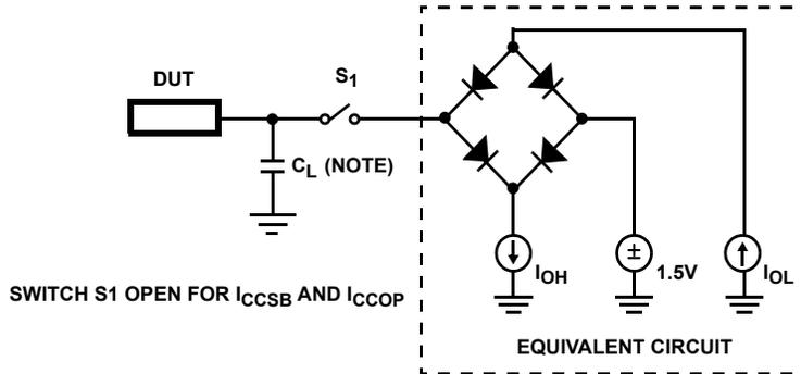
NOTE: Test head capacitance.
