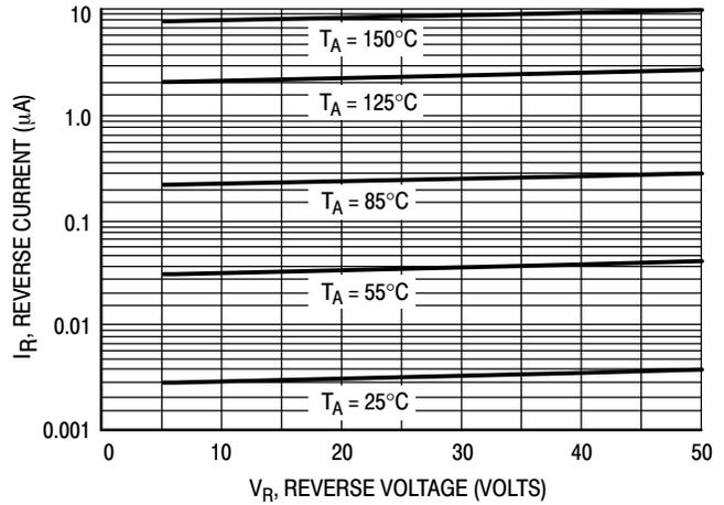
**Figure 3. Leakage Current**
