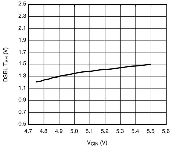
**DSBL Falling Threshold vs. V<sub>CIN</sub>**
