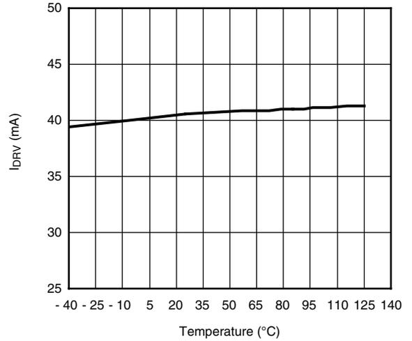
**I<sub>DRV</sub> (mA) vs. Temperature at Frequency = 1 MHz**
