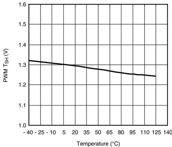
**PWM Falling Tristate (V) vs. Temperature (°C)**
