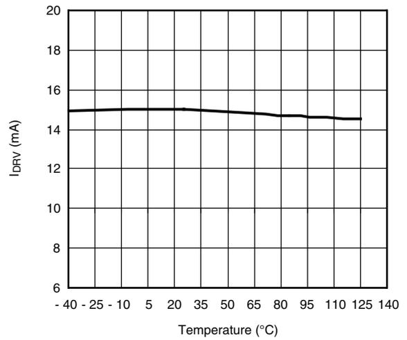
**I<sub>DRV</sub> (mA) vs. Temperature at Frequency = 300 kHz**
