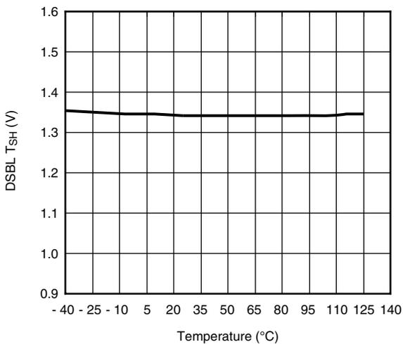
**DSBL Falling Threshold (V) vs. Temperature (°C)**
