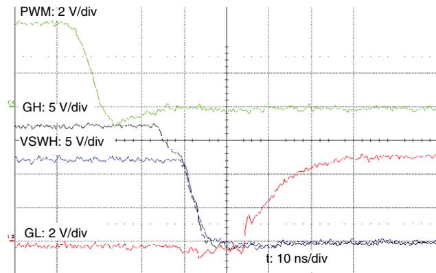
Switching Waveforms at PWM falling edge
