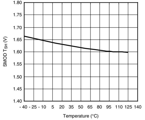
**SMOD Rising Threshold (V) vs. Temperature (°C)**
