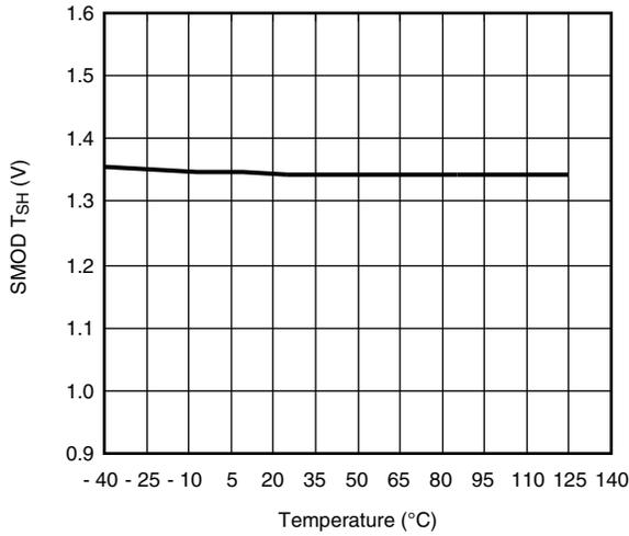
**SMOD Falling Threshold (V) vs. Temperature (°C)**
