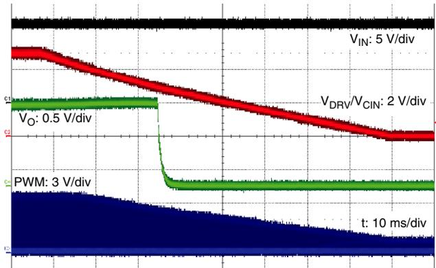
Power Off with  $V_{DRV}/V_{CIN}$  ramping down
