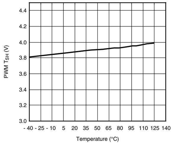
**PWM Rising Threshold (V) vs. Temperature (°C)**
