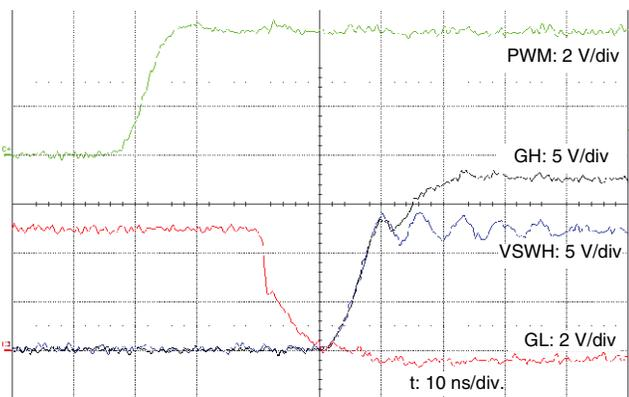
Switching Waveforms at PWM rising edge
