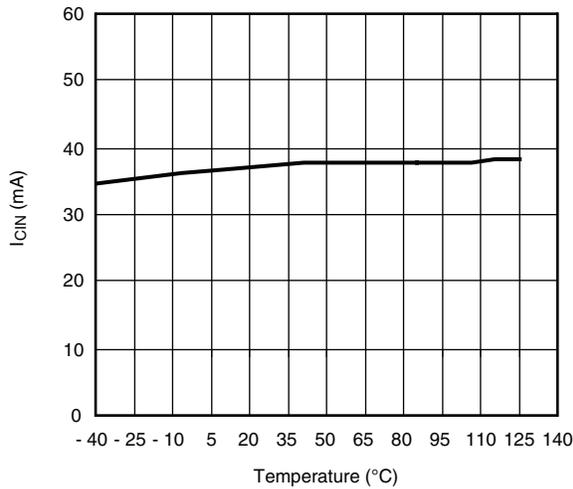
**I<sub>CIN</sub> + I<sub>DRV</sub> (mA) vs. Temperature at Frequency = 1 MHz**
