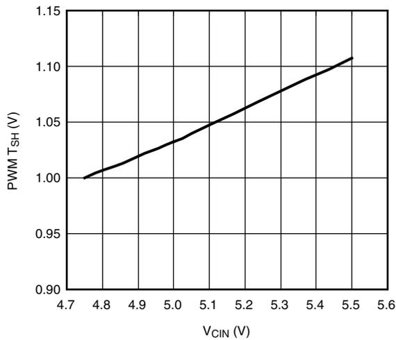
**PWM Falling Threshold vs. V<sub>CIN</sub>**
