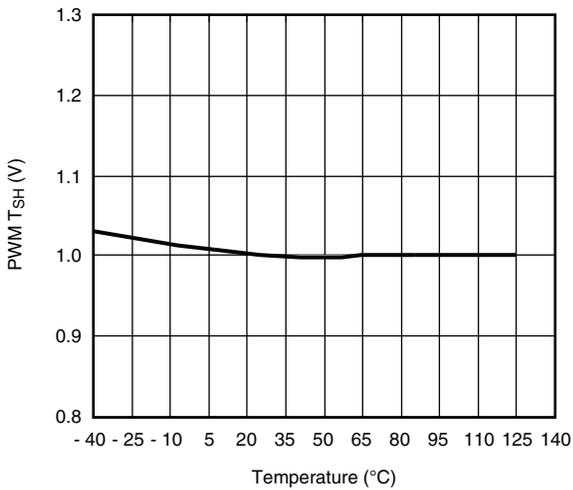
**PWM Falling Threshold (V) vs. Temperature (°C)**
