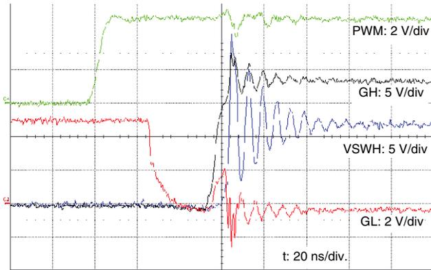
**Switching Waveforms at PWM rising edge**
