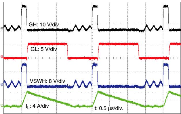
Switching Waveforms with SMOD enabled
