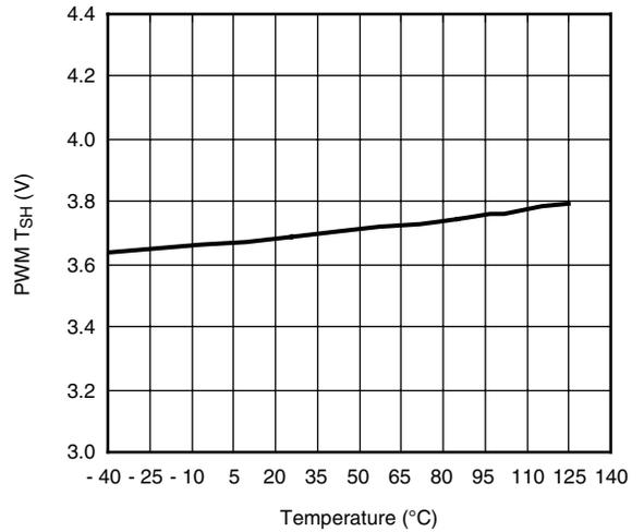
**PWM Rising Tristate Threshold (V) vs. Temperature (°C)**
