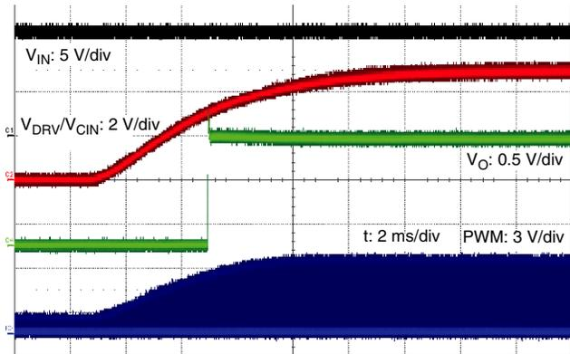
Startup with  $V_{DRV}/V_{CIN}$  ramping up
