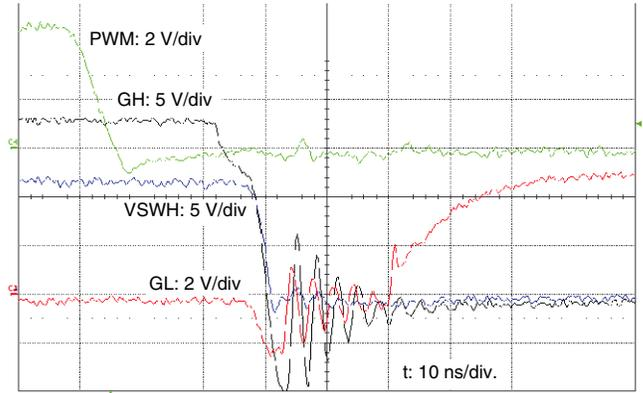
**Switching Waveforms at PWM falling edge**
