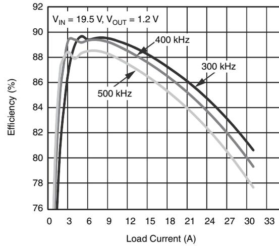
$V_{IN} = 12\text{ V}$  and  $19.5\text{ V}$ ,  $V_{OUT} = 1.2\text{ V}$ ,  $V_{DRV} = V_{CIN} = 5\text{ V}$ ; No Air Flow
