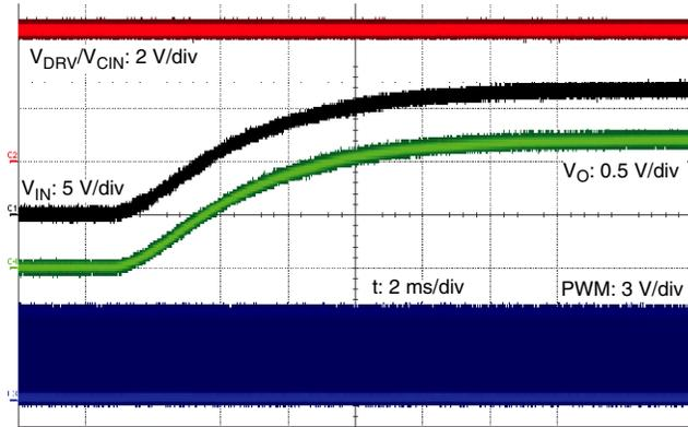
**Startup with  $V_{IN}$  ramping up**
