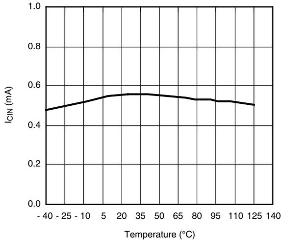
**I<sub>CIN</sub> (mA) vs. Temperature at Frequency = 300 kHz**
