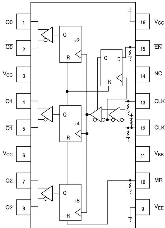
Warning: All  $V_{CC}$  and  $V_{EE}$  pins must be externally connected to Power Supply to guarantee proper operation.
