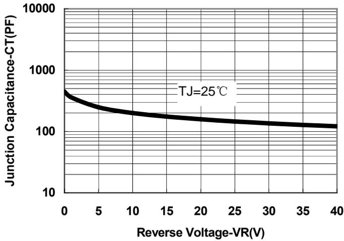
Fig.1-Typical Junction Capacitance
