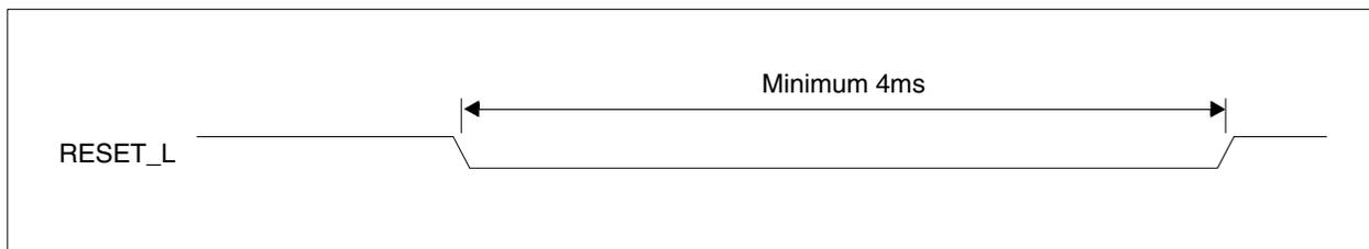
*Figure 14-1: Reset Timing Requirement for Input Clock From Oscillator*
