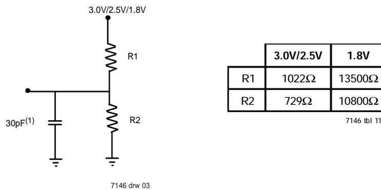
Figure 1. AC Output Test Load
