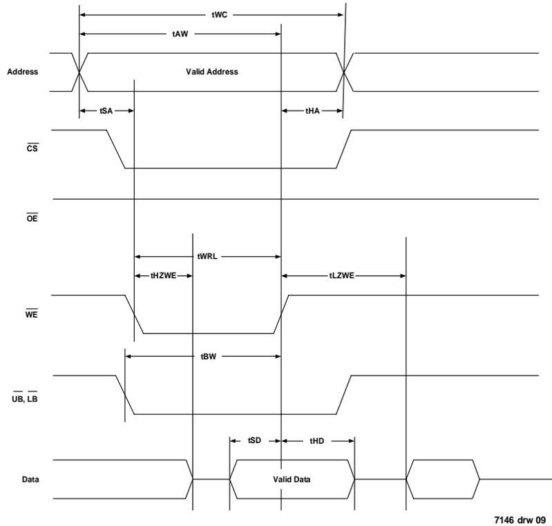
Standard Port Write Cycle (Either Port Access,  **$\overline{CS}$**  Controlled)
