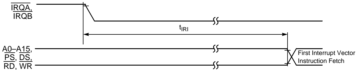
Figure 3-15 Interrupt from Wait State Timing
