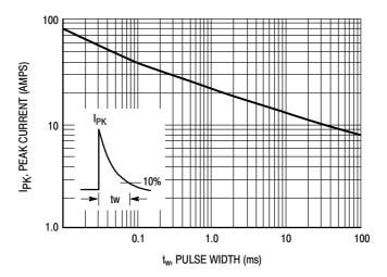
Figure 8. Pulse Rating Curve
