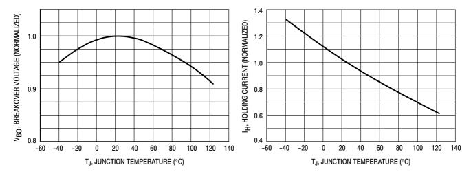
Figure 6. Typical Breakover Voltage
