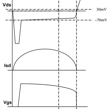
**Figure 4: Synchronous Rectification Operation at Light Load**
