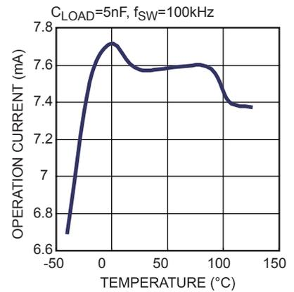
Light Load Mode Current vs. Temperature
