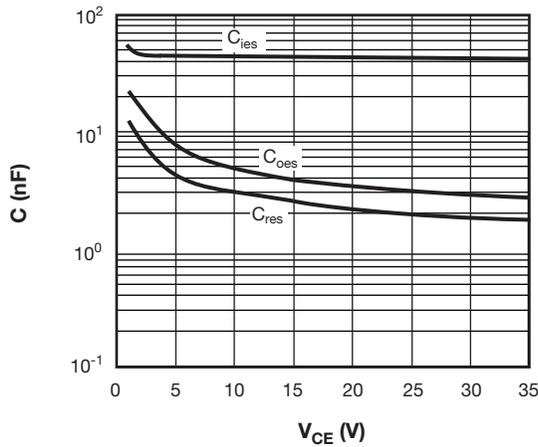
Fig. 6 - Typical Capacitance vs. Collector-Emitter Voltage
