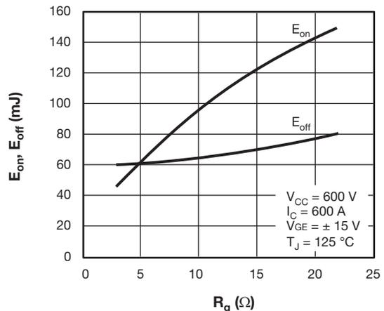
Fig. 4 - Switching Loss vs. Gate Resistor
