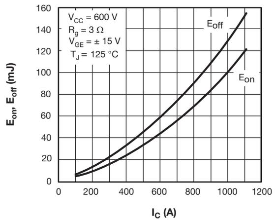
Fig. 3 - Switching Loss vs. Collector Current
