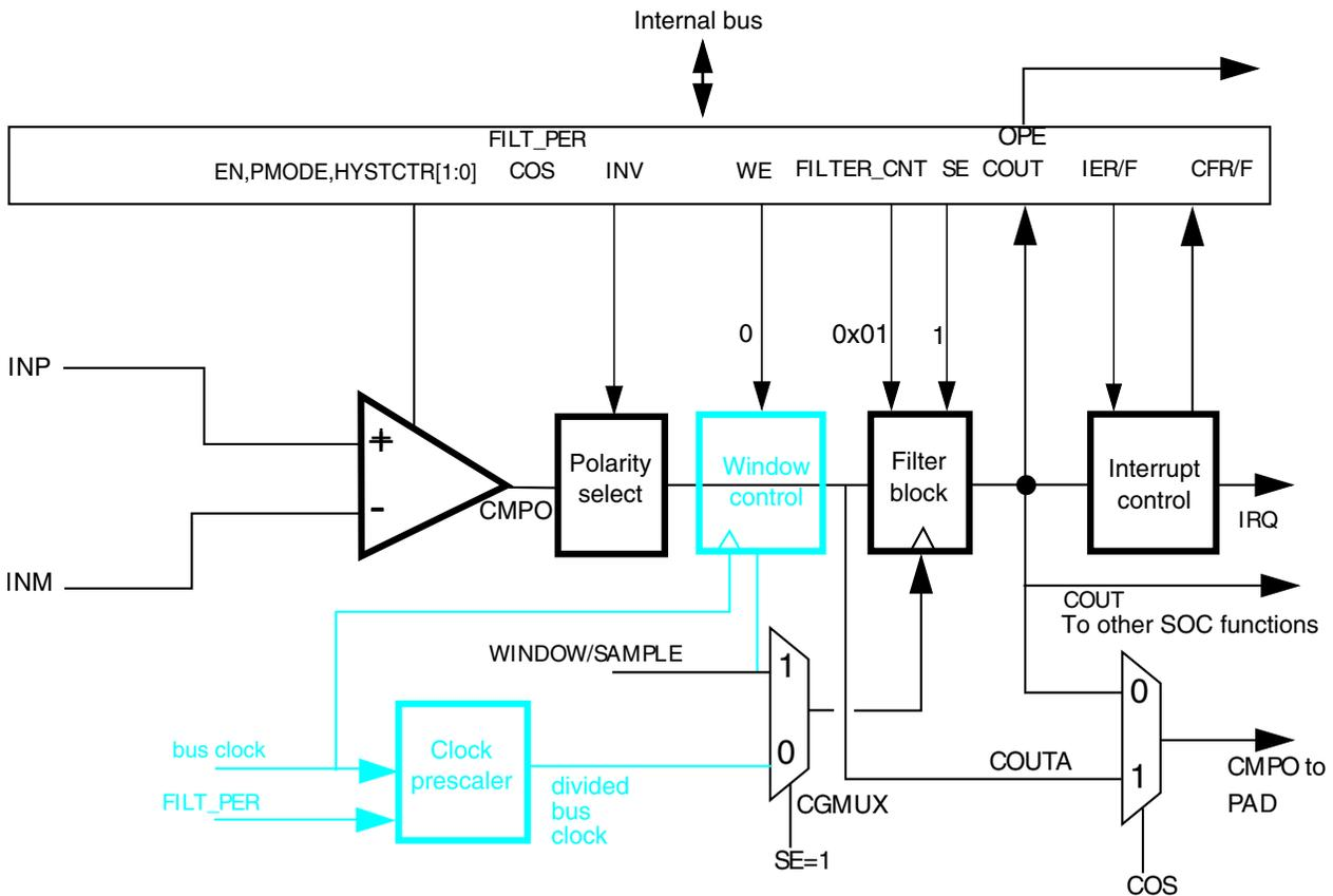
**Figure 33-28. Sampled, Non-Filtered (# 3A): sampling point externally driven**
