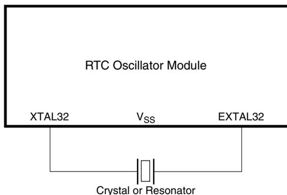
Figure 27-2. Crystal Connections
