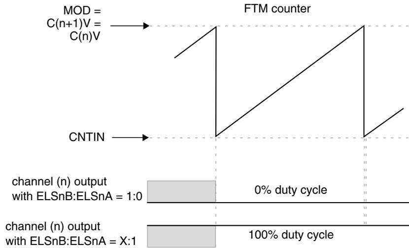
**Figure 37-196. Channel (n) output if  $(C(n)V = C(n+1)V = MOD)$**
