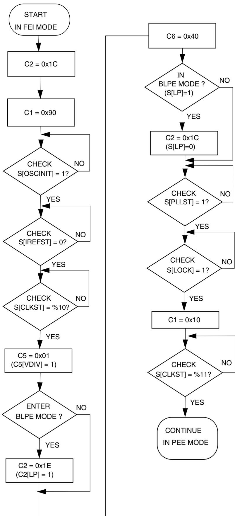
Figure 25-17. Flowchart of FEI to PEE mode transition using an 4 MHz crystal
