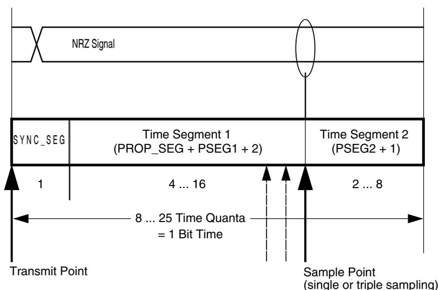
**Figure 45-99. Segments within the bit time**
