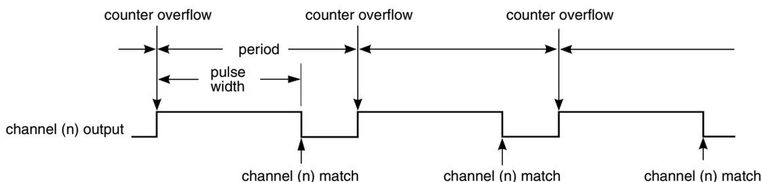
**Figure 37-181. EPWM period and pulse width with ELSnB:ELSnA = 1:0**
