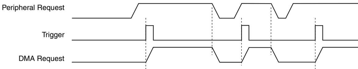
**Figure 21-20. DMA MUX channel triggering: normal operation**
