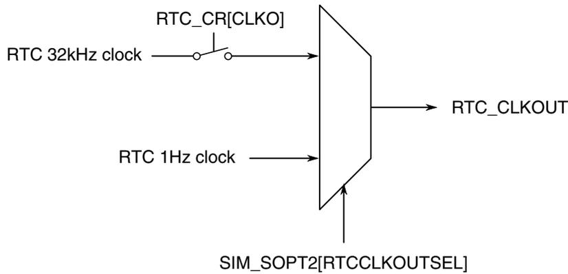
Figure 3-46. RTC\_CLKOUT generation
