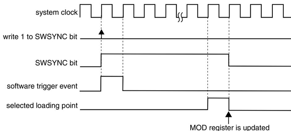
**Figure 37-213. MOD synchronization with (SYNCMODE = 0) and (PWMSYNC = 1)**
