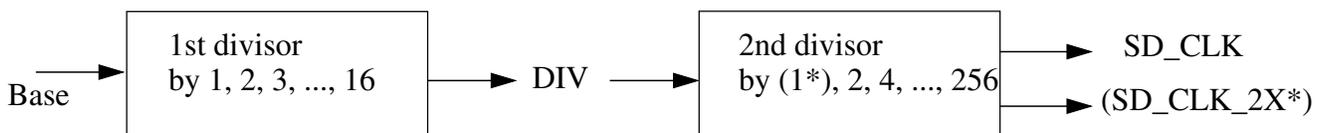
**Figure 49-35. Two stages of the clock divider**
