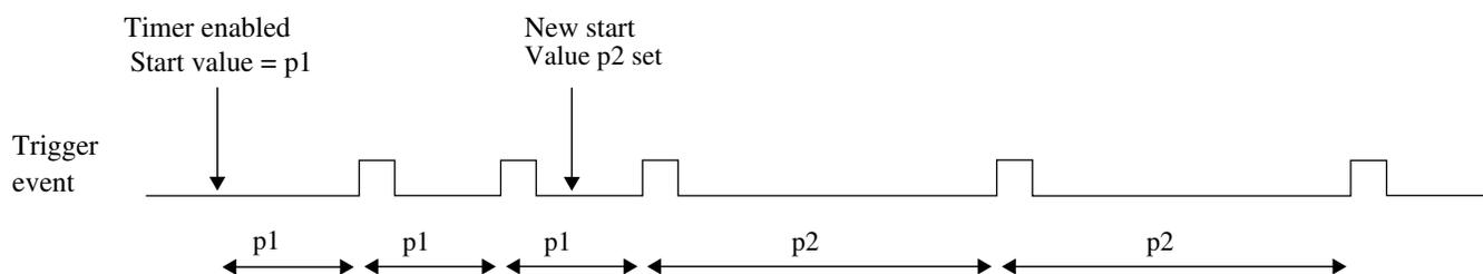
**Figure 38-25. Dynamically setting a new load value**
