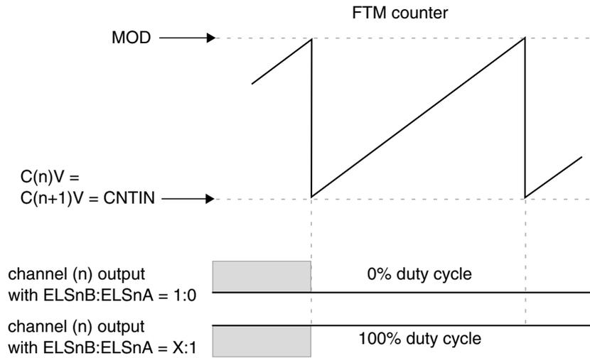
**Figure 37-195. Channel (n) output if  $(C(n)V = C(n+1)V = CNTIN)$**
