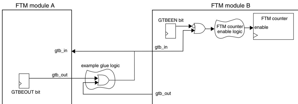
**Figure 37-258. Global time base (GTB) block diagram**
