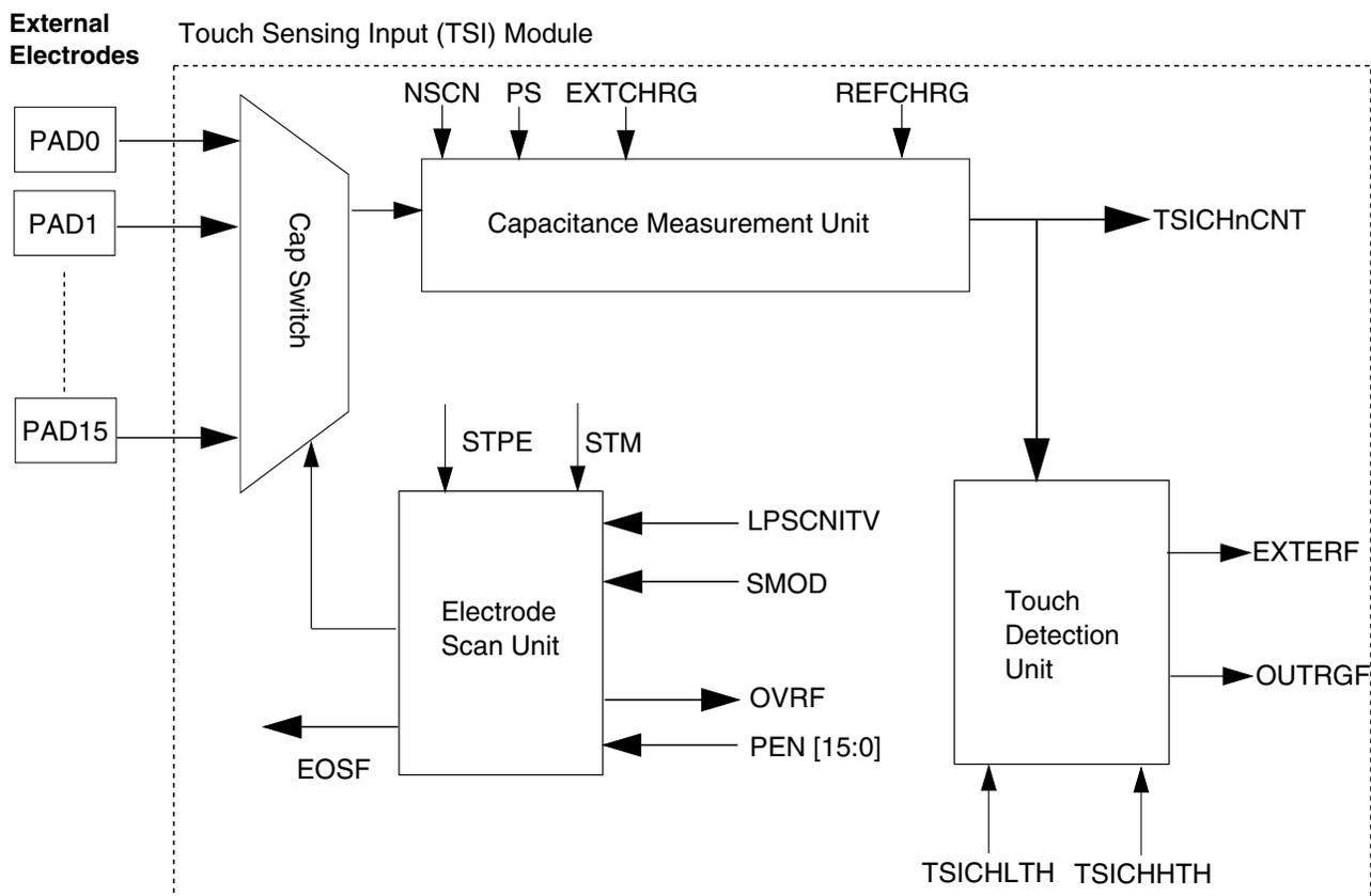
Figure 52-1. TSI block diagram
