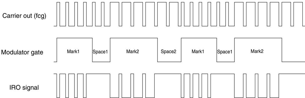
**Figure 40-18. Example: CMT output in FSK mode**
