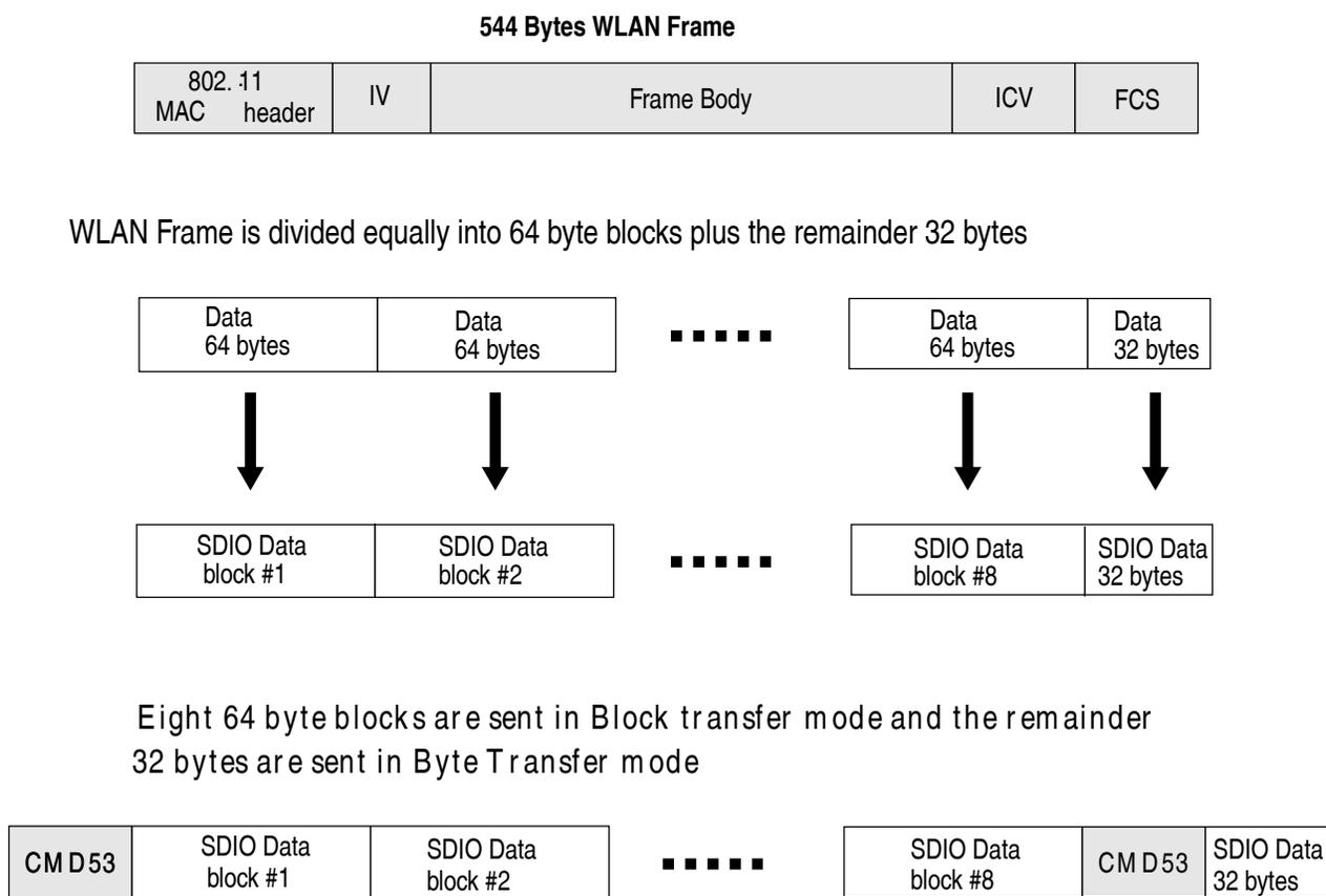
**Figure 49-30. Example for dividing large data transfers**
