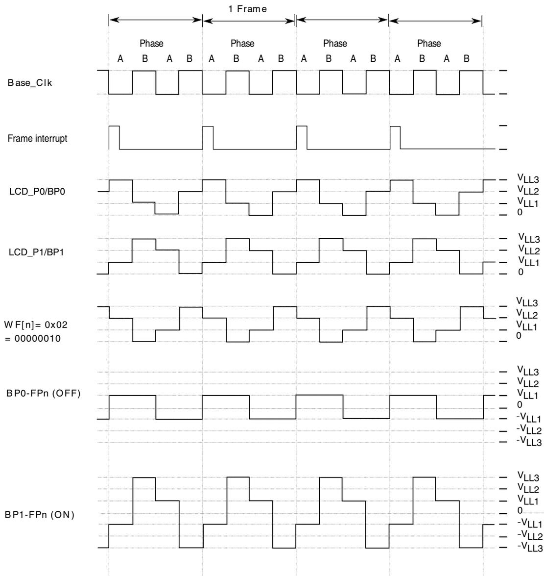
Figure 53-29. 1/2 duty and 1/3 bias (low-power waveform)
