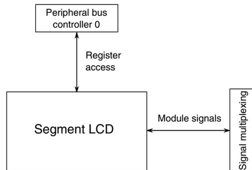
Figure 3-62. SLCD configuration
