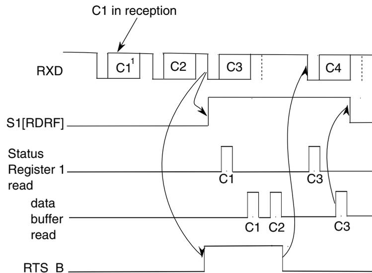
**Figure 48-345. Receiver hardware flow control timing diagram**
