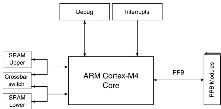
**Figure 3-1. Core configuration**
