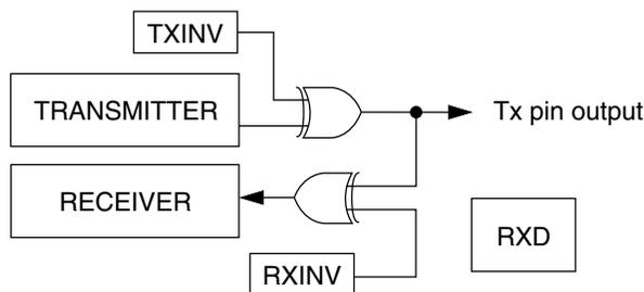
**Figure 48-359. Loop operation ( $C1[LOOPS] = 1, C1[RSRC] = 0$ )**
