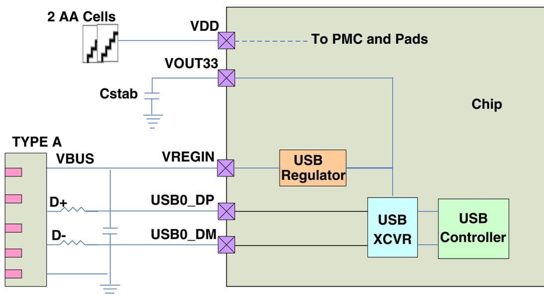
Figure 3-48. USB regulator AA cell usecase
