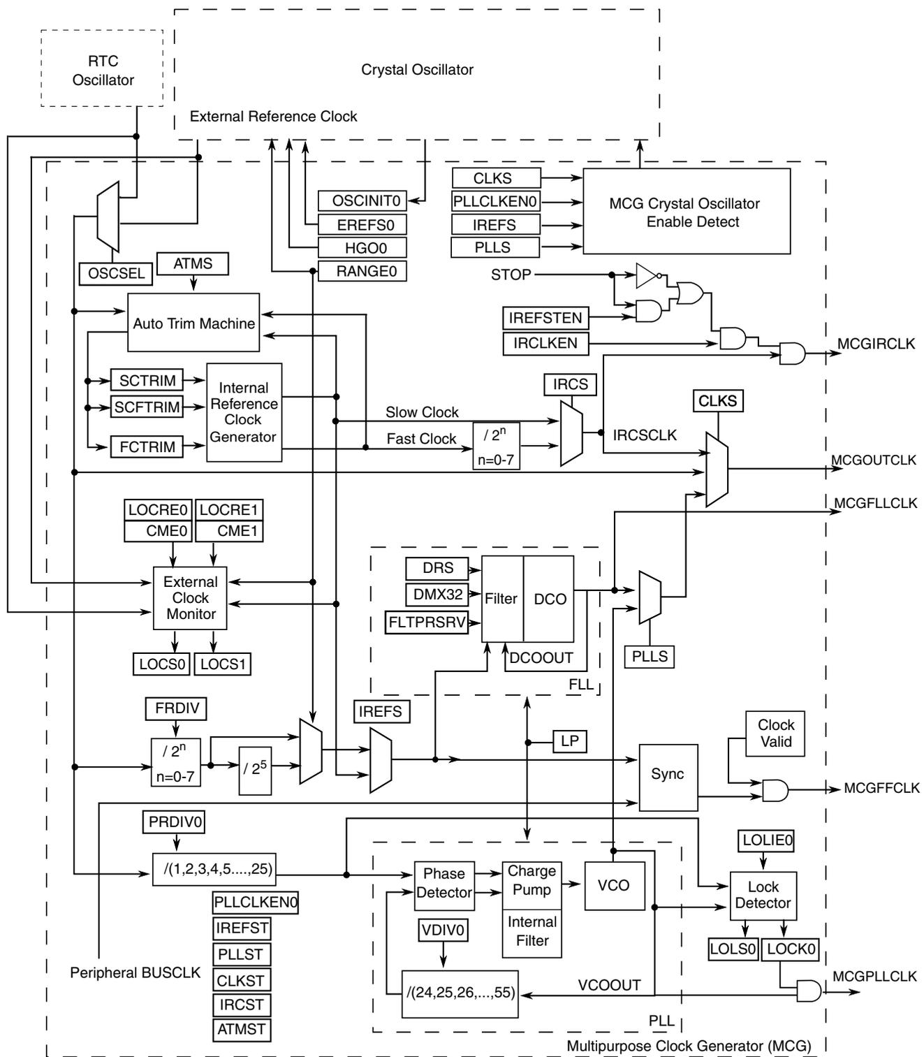
Figure 25-1. Multipurpose Clock Generator (MCG) block diagram
