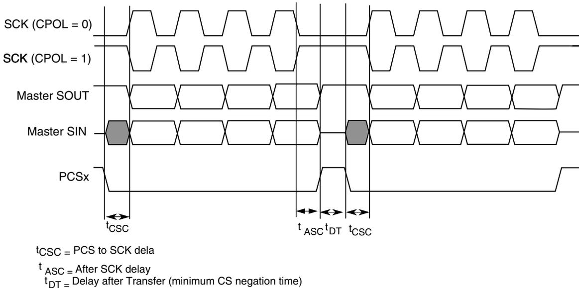
**Figure 46-95. Example of non-continuous format (CPHA=1, CONT=0)**
