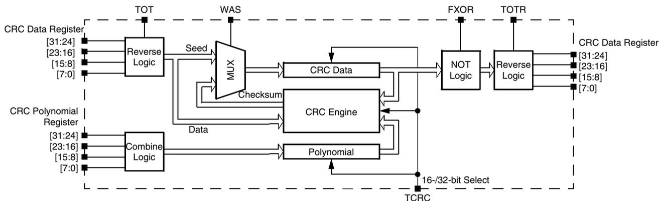
Figure 31-1. Programmable cyclic redundancy check (CRC) block diagram
