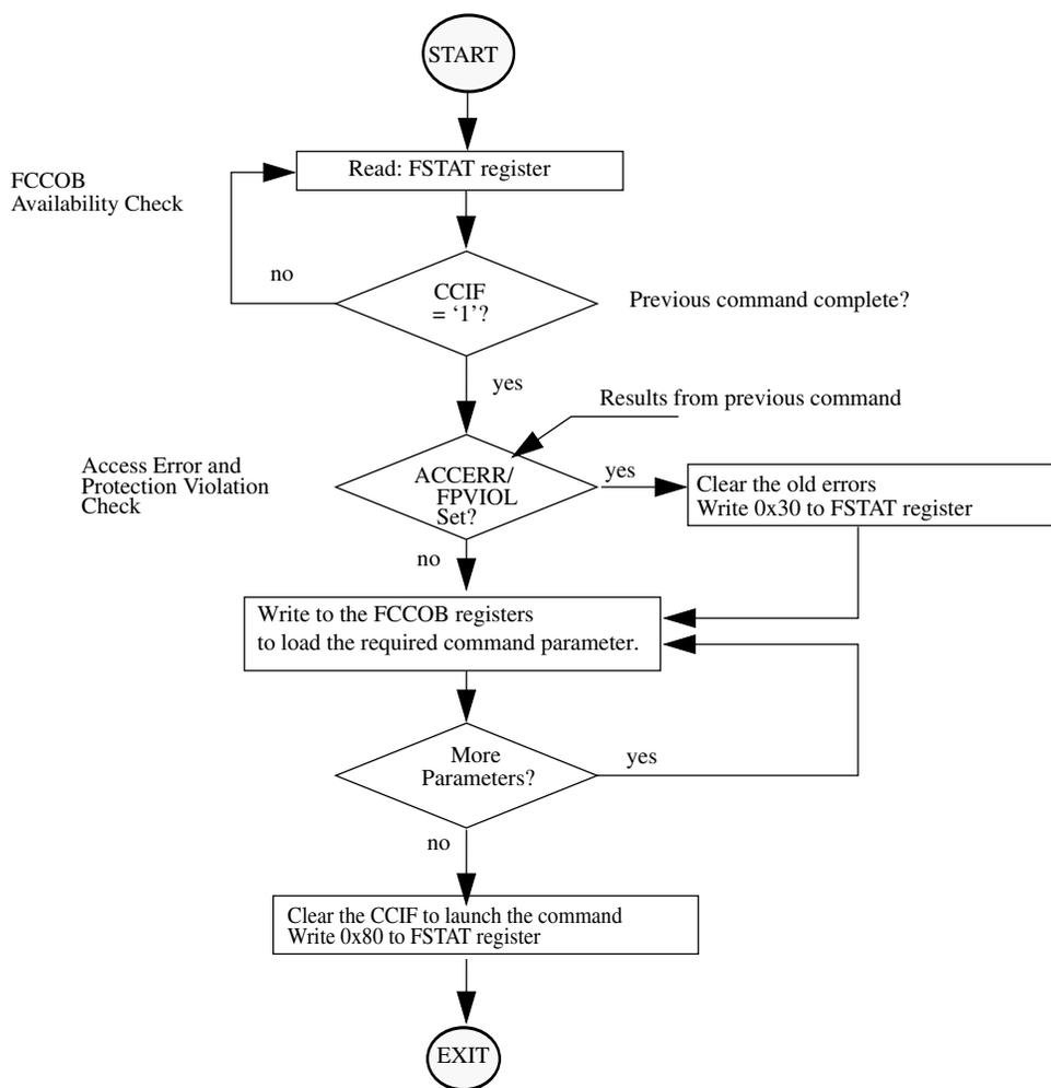
Figure 29-25. Generic Flash Command Write Sequence Flowchart
