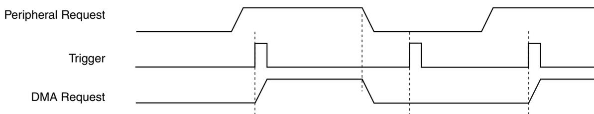
**Figure 21-21. DMA MUX channel triggering: ignored trigger**
