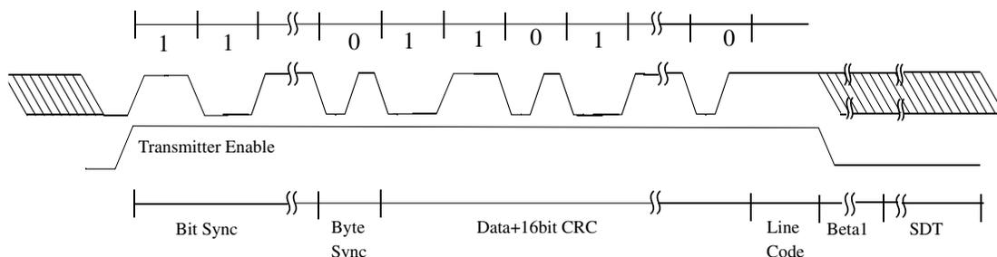
**Figure 48-337. Frame format with differential manchester encoding**
