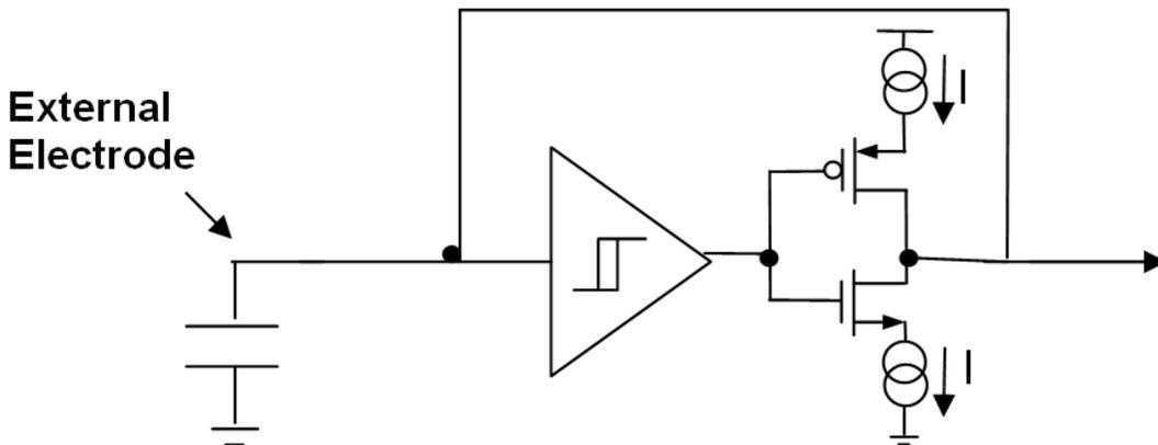
**Figure 52-33. TSI electrode oscillator circuit**
