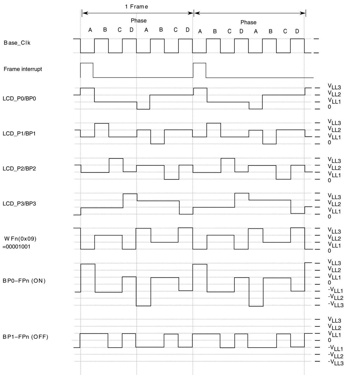
Figure 53-30. 1/4 duty and 1/3 bias (low-power waveform)
