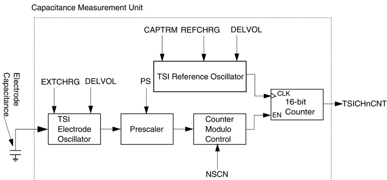
**Figure 52-2. TSI capacitance measurement unit block diagram**
