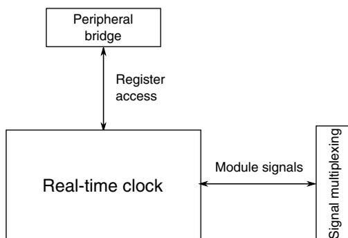
Figure 3-45. RTC configuration
