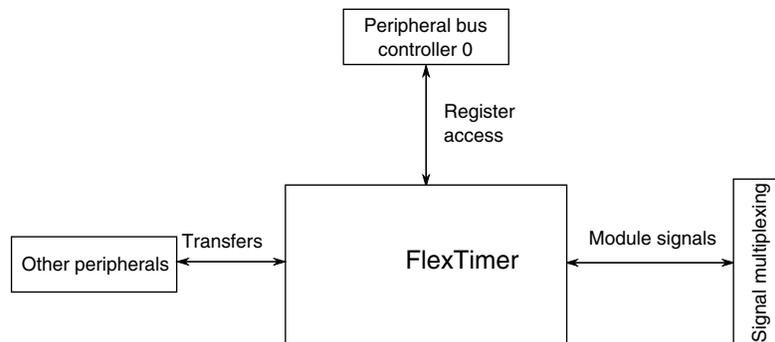
**Figure 3-40. FlexTimer configuration**
