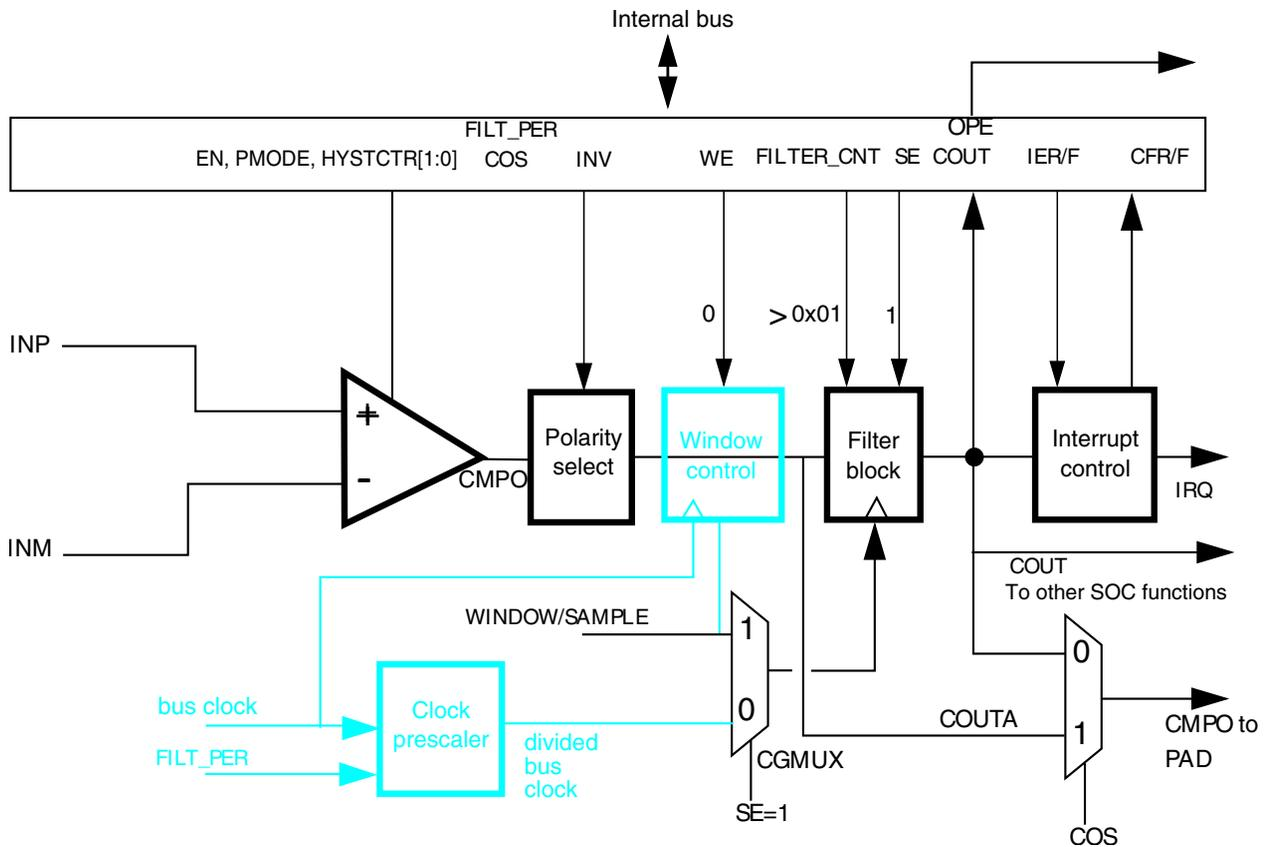
Figure 33-30. Sampled, Filtered (# 4A): sampling point externally driven
