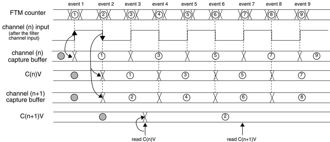
**Figure 37-249. Dual Edge Capture mode read coherency mechanism**
