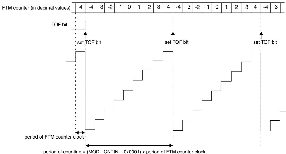
**Figure 37-168. Example of FTM up and signed counting**
