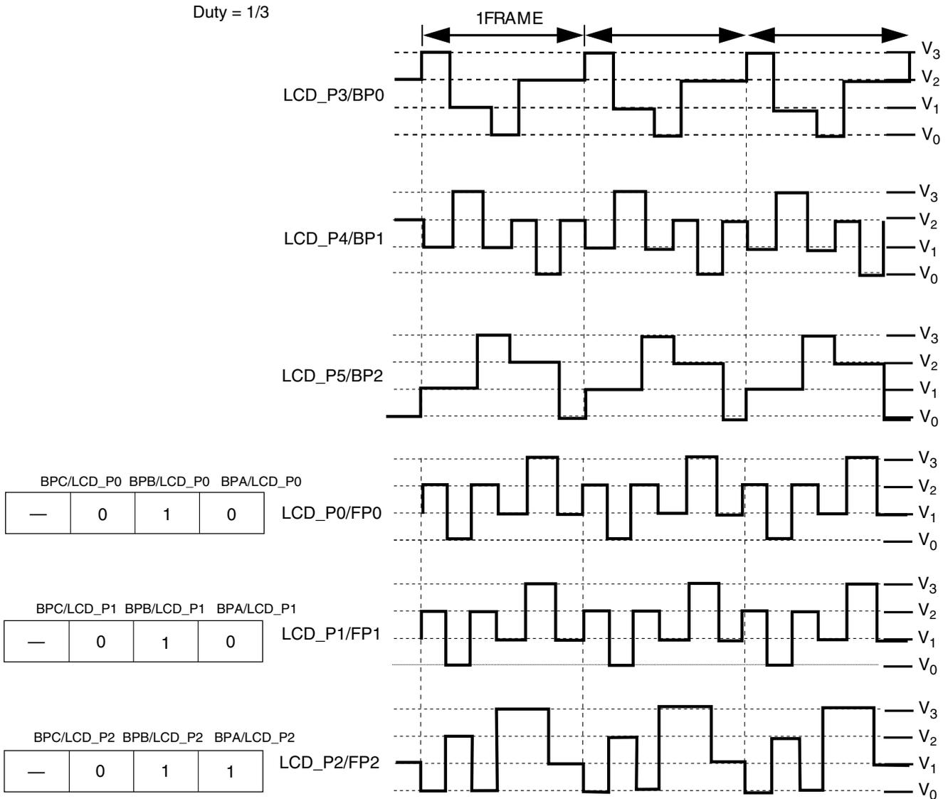
Figure 53-40. LCD waveforms
