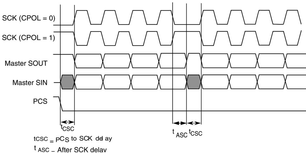
**Figure 46-96. Example of continuous transfer (CPHA=1, CONT=1)**
