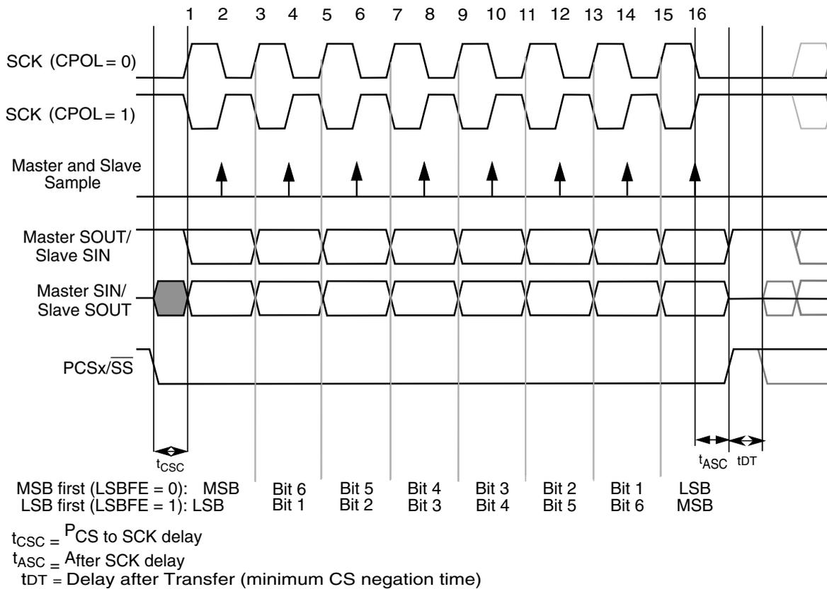
**Figure 46-94. Module transfer timing diagram (MTFE=0, CPHA=1, FMSZ=8)**
