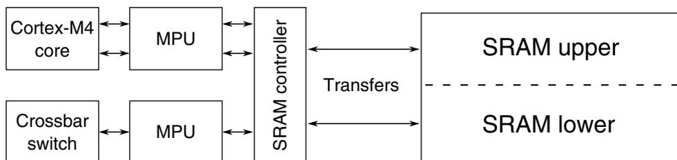
Figure 3-23. SRAM configuration
