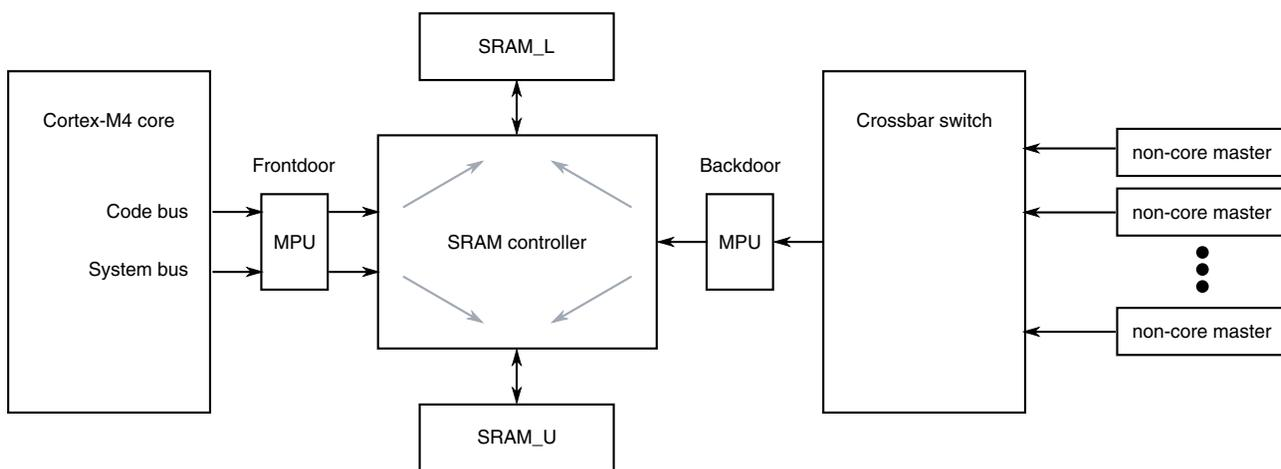
**Figure 3-25. SRAM access diagram**
