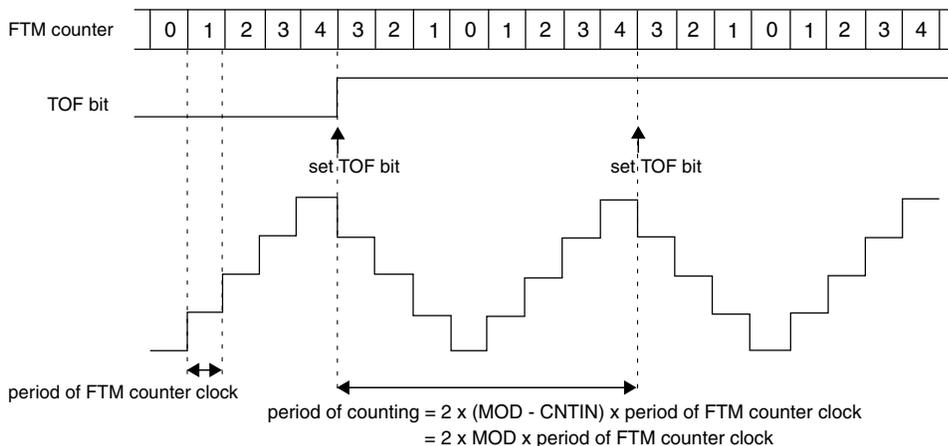
Figure 37-171. Example of up-down counting when CNTIN = 0x0000
