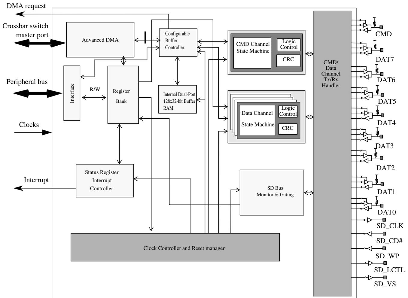
Figure 49-2. Enhanced secure digital host controller block diagram
