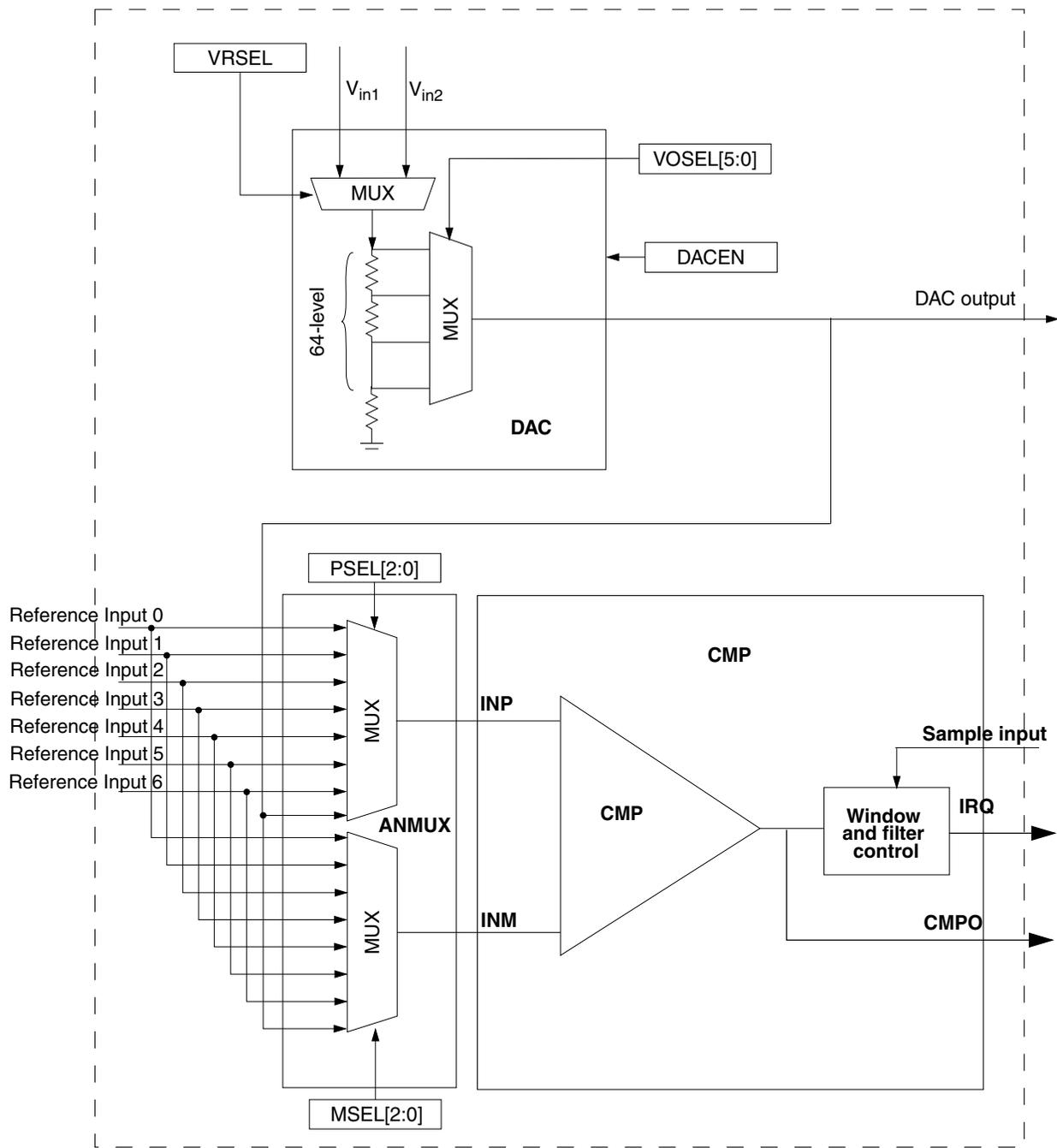
Figure 33-1. CMP, DAC and ANMUX block diagram
