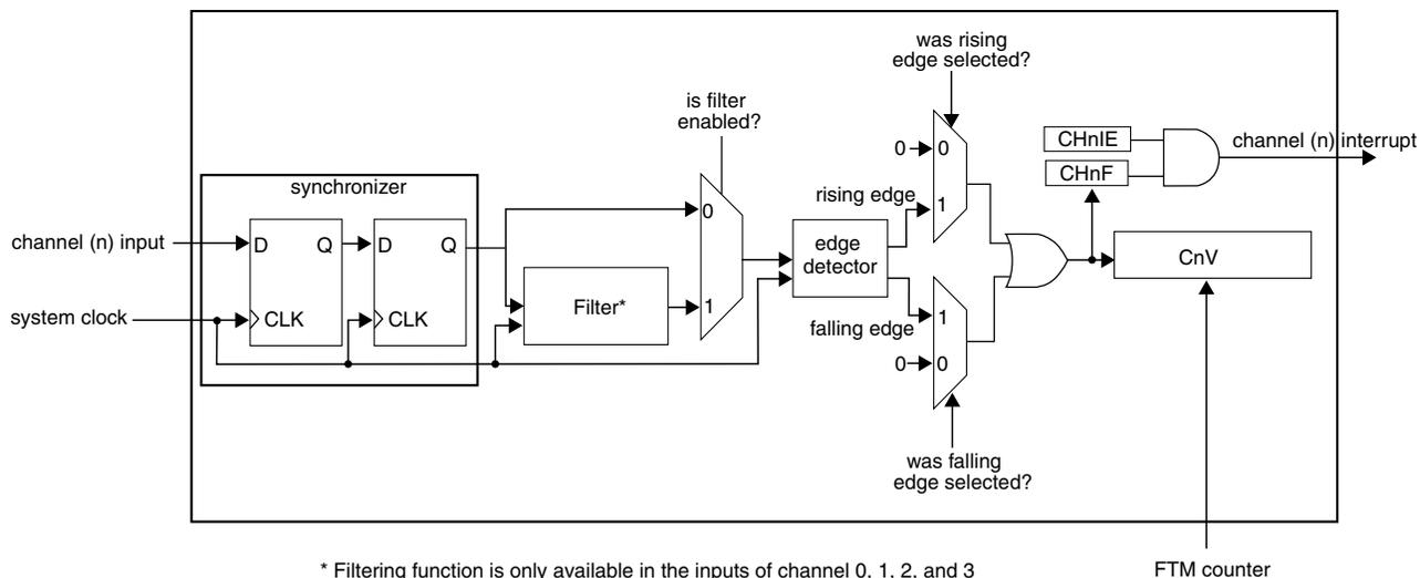
**Figure 37-175. Input Capture mode**
