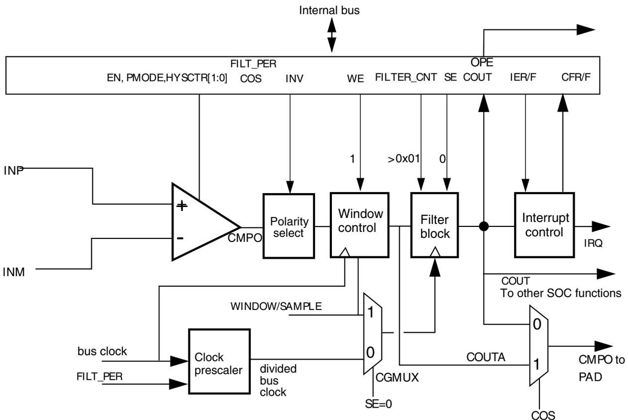
Figure 33-35. Windowed/Filtered mode
