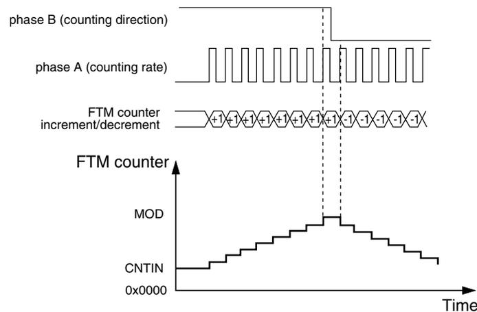
**Figure 37-251. Quadrature Decoder – Count and Direction Encoding mode**
